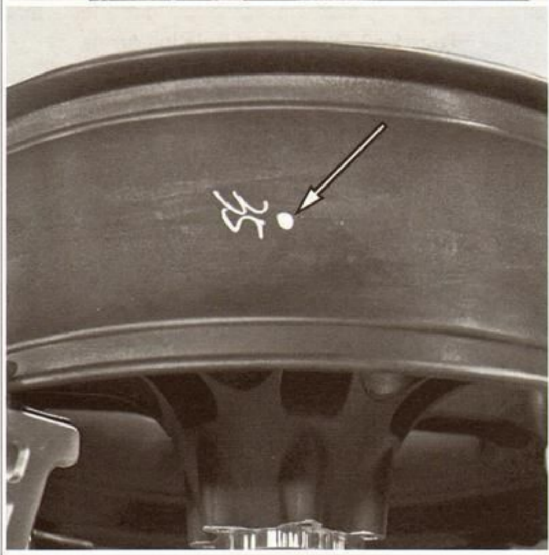
Figure 2-15. Tire and Wheel Balance Dots
