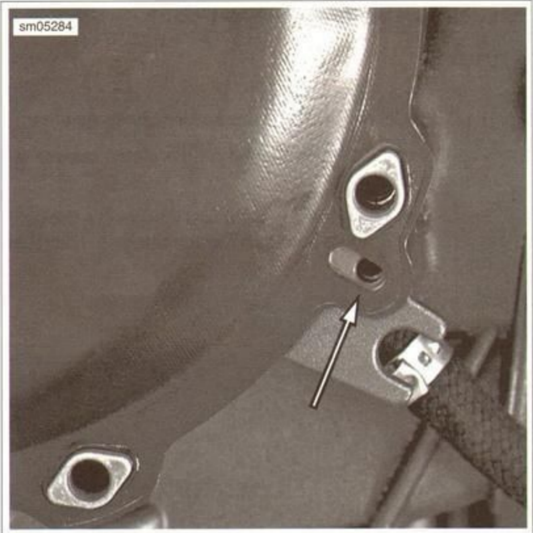
Figure 6-33. Gasket, Inner Cover and Diaphragm Alignment
