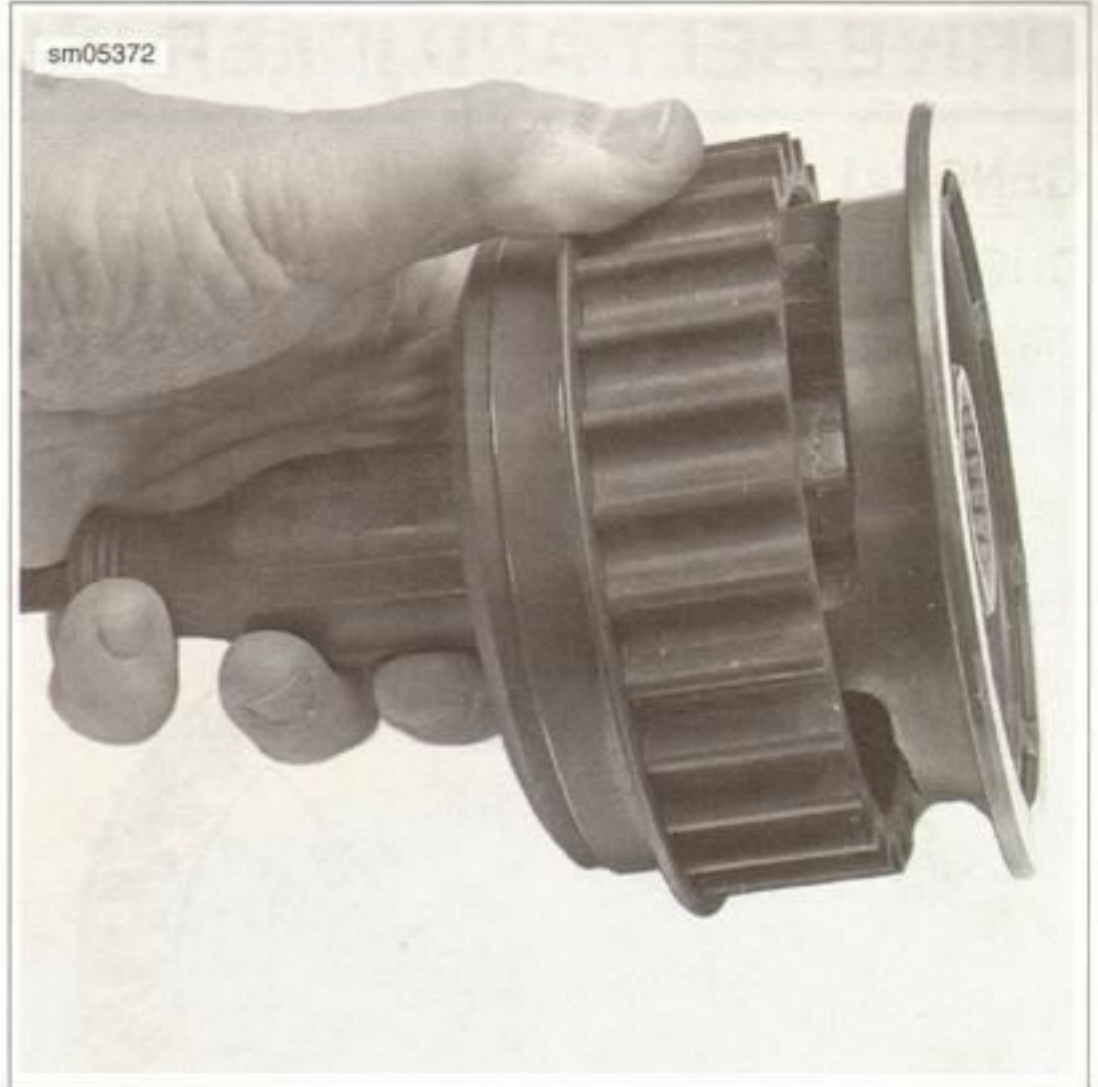
Figure 6-111. Separating the Pulley Assembly
