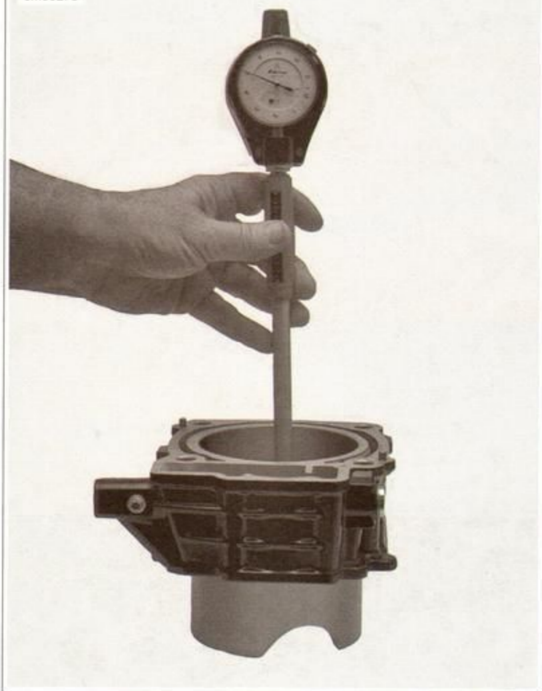
Figure 3-99. Measuring Cylinder Bore
