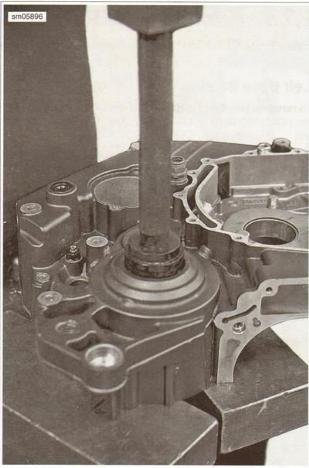
Figure 6-98. Mainshaft Bearing Removal: Left Case
