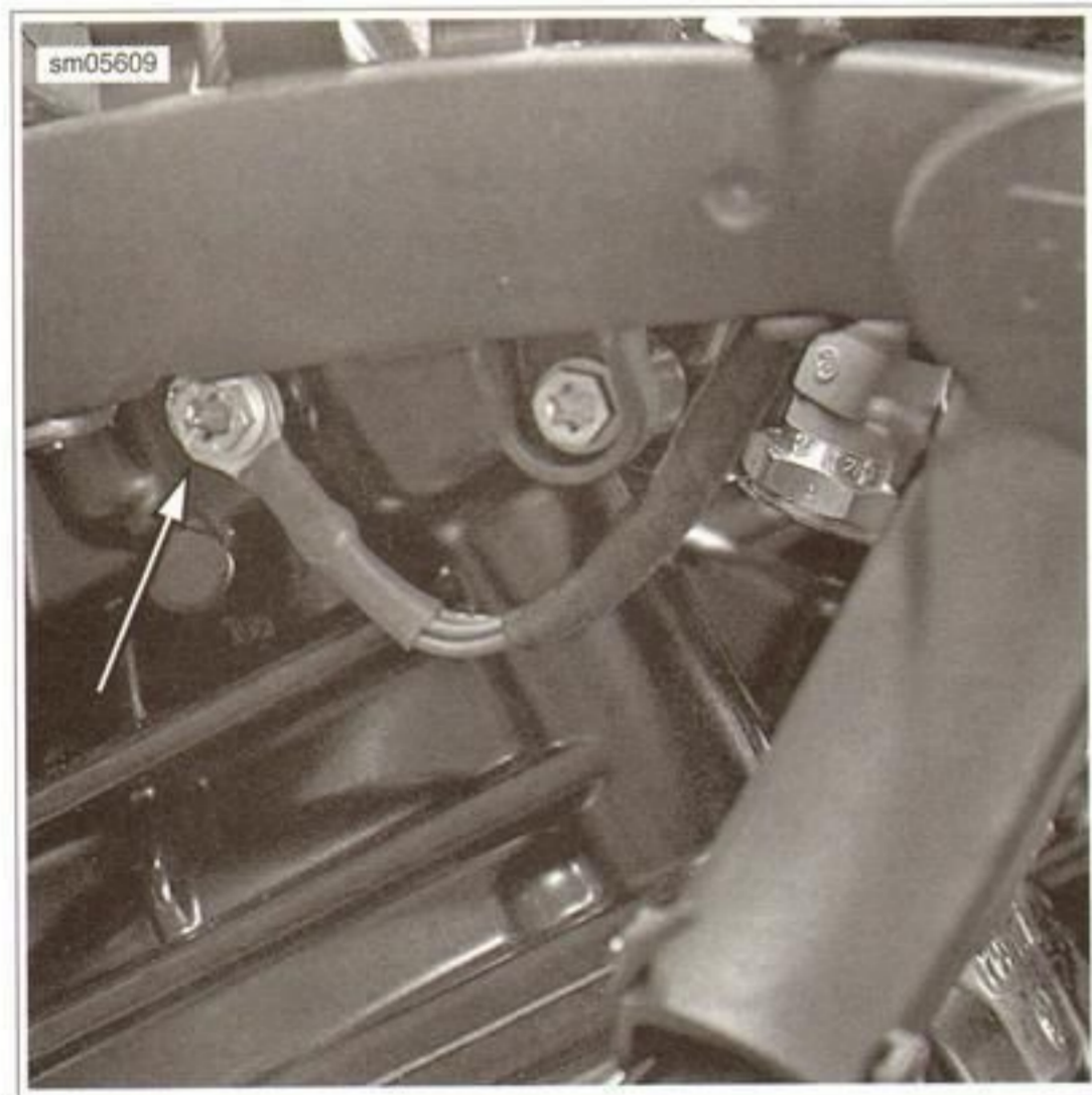
Figure 7-108. Engine Ground Connection
