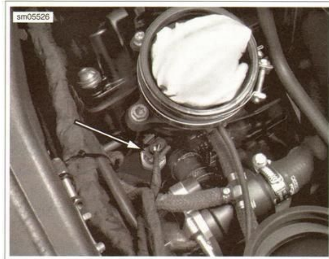
Figure 3-22. Engine Temperature Sensor
