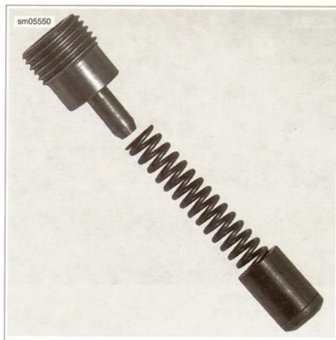
Figure 3-140. Pressure Relief Valve
