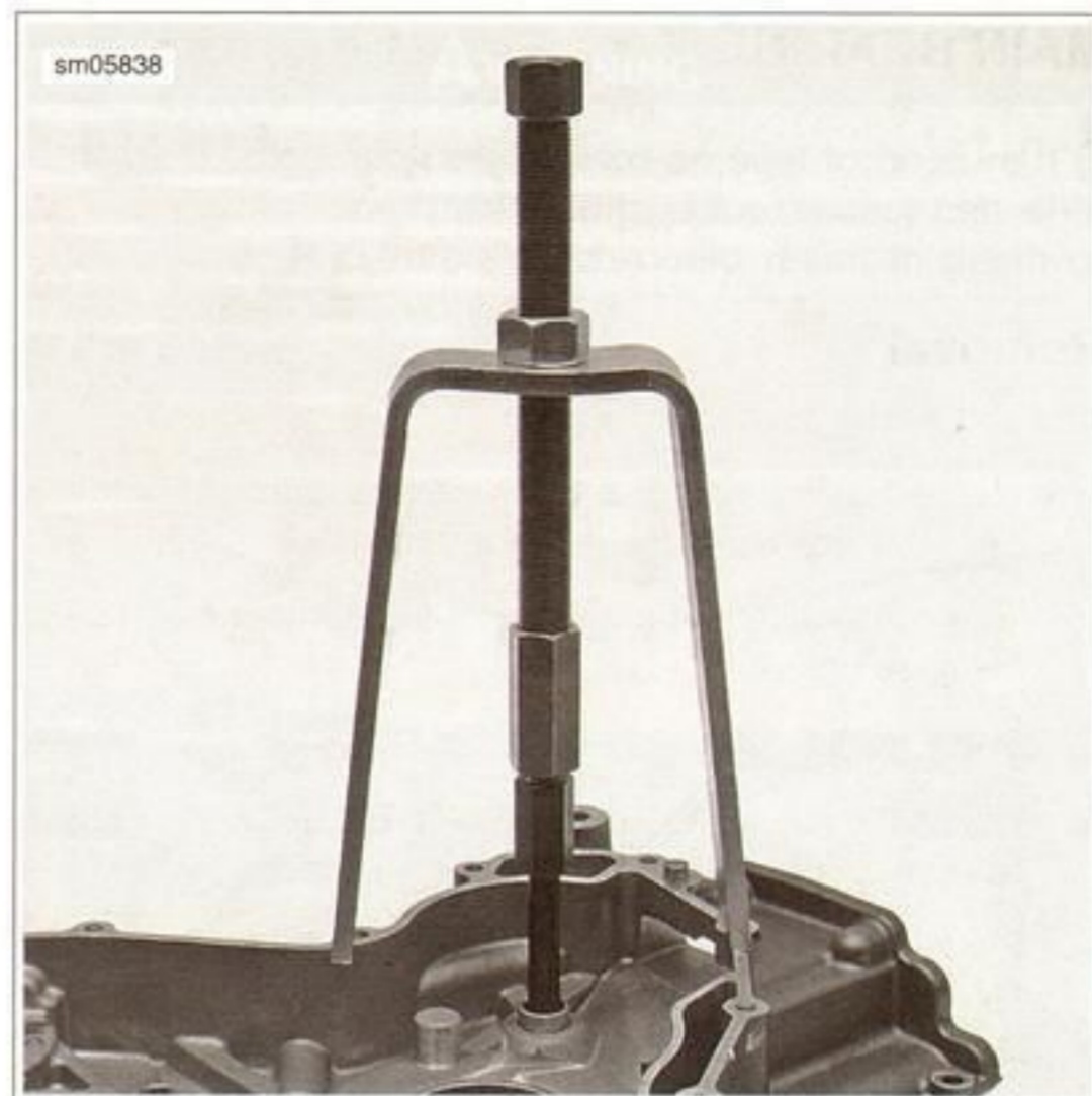
Figure 3-181. Remove the Water Pump Shaft Case Bearing
