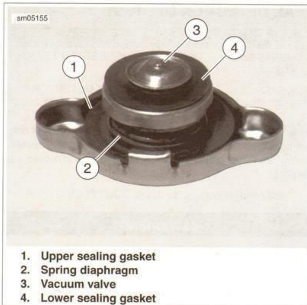
Figure 5-2. Pressure Cap
