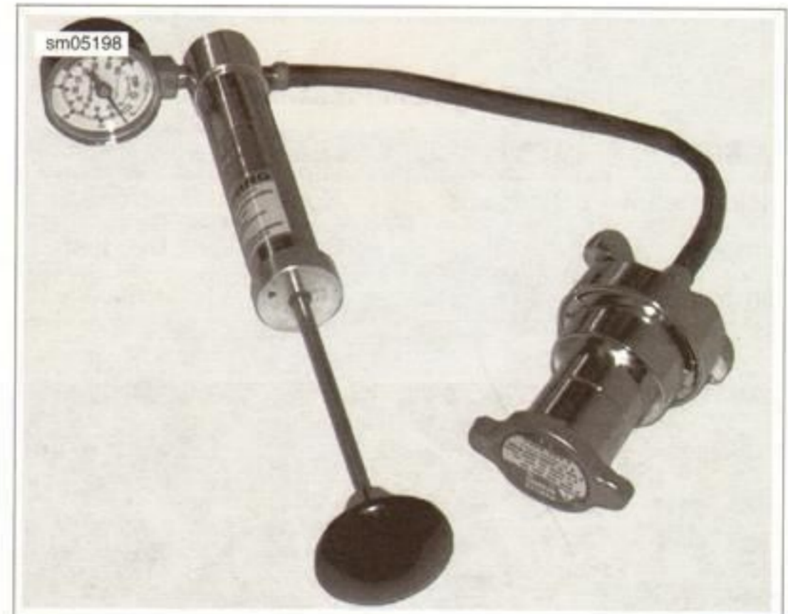
Figure 5-4. Pressure Cap Test
