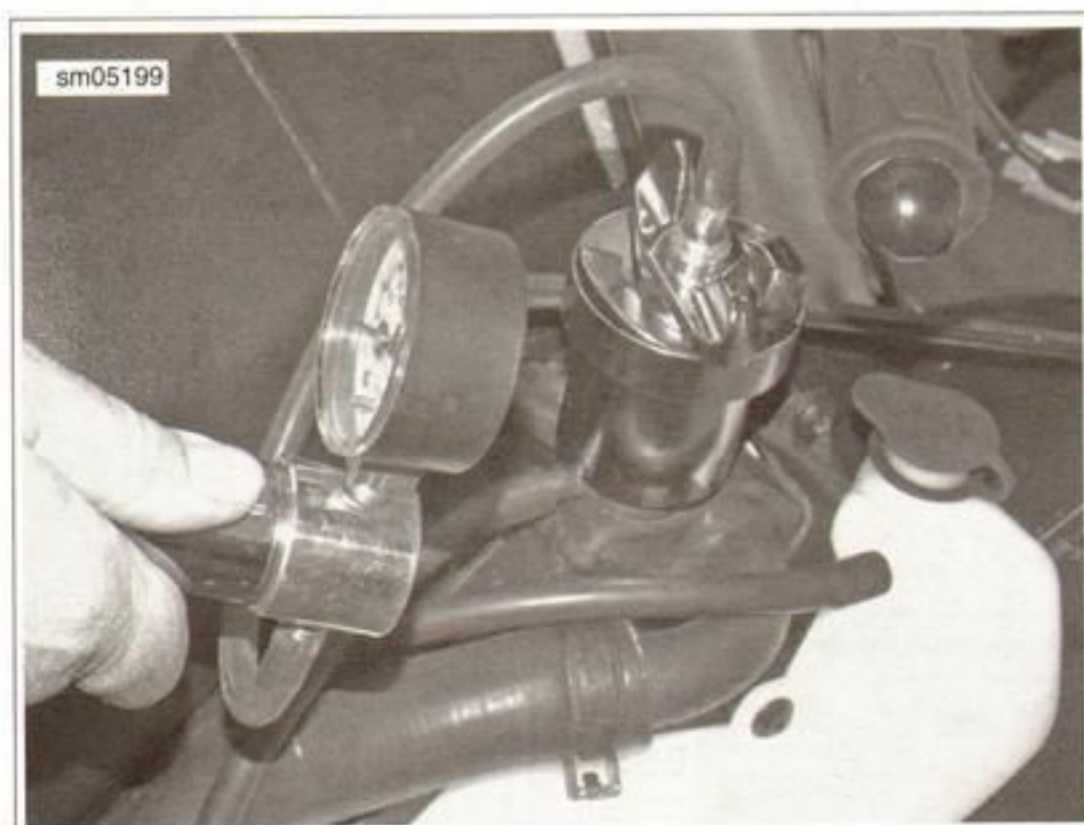
Figure 5-5. System Pressure Test
