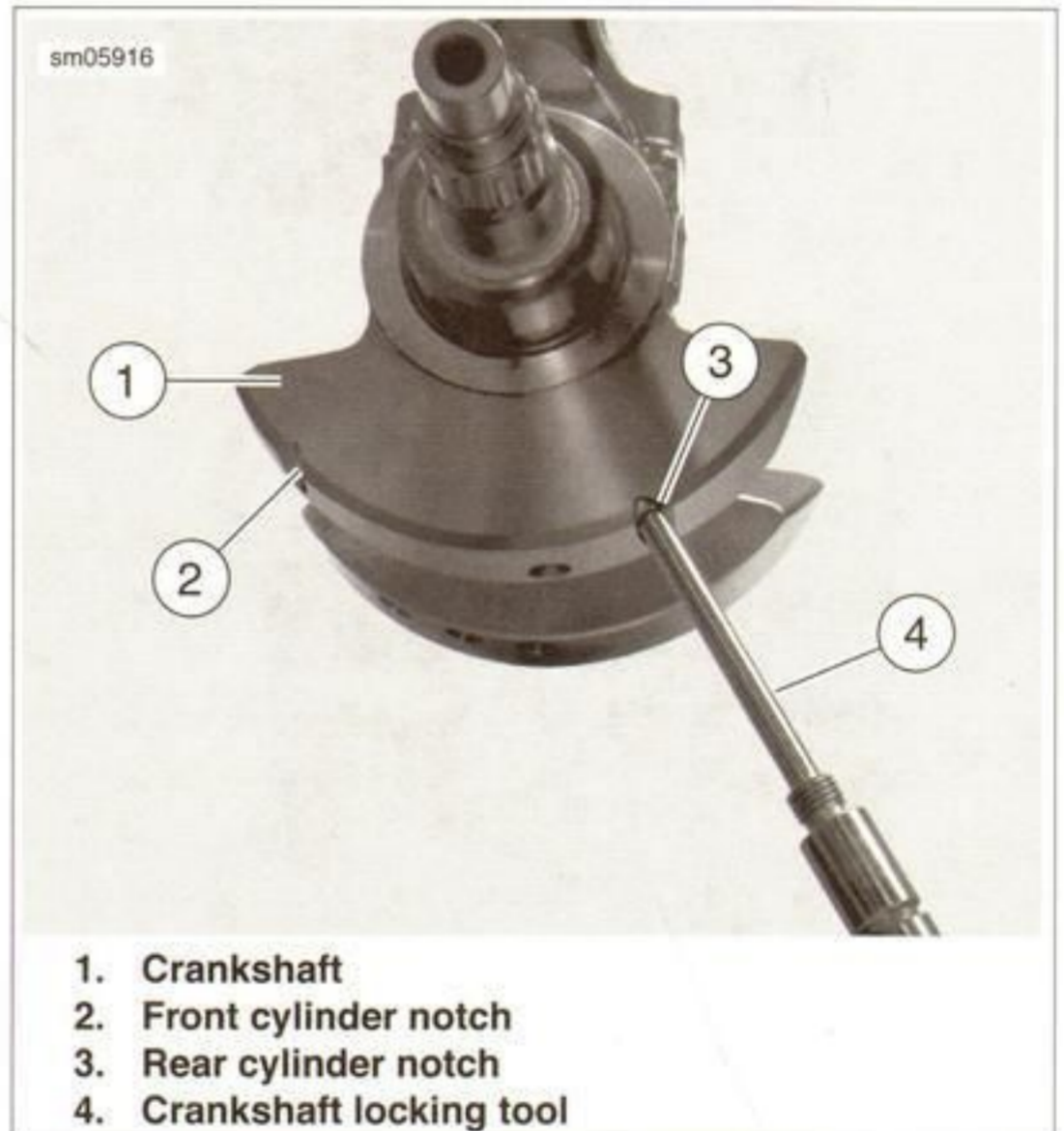
Figure 3-61. Locking Crankshaft
