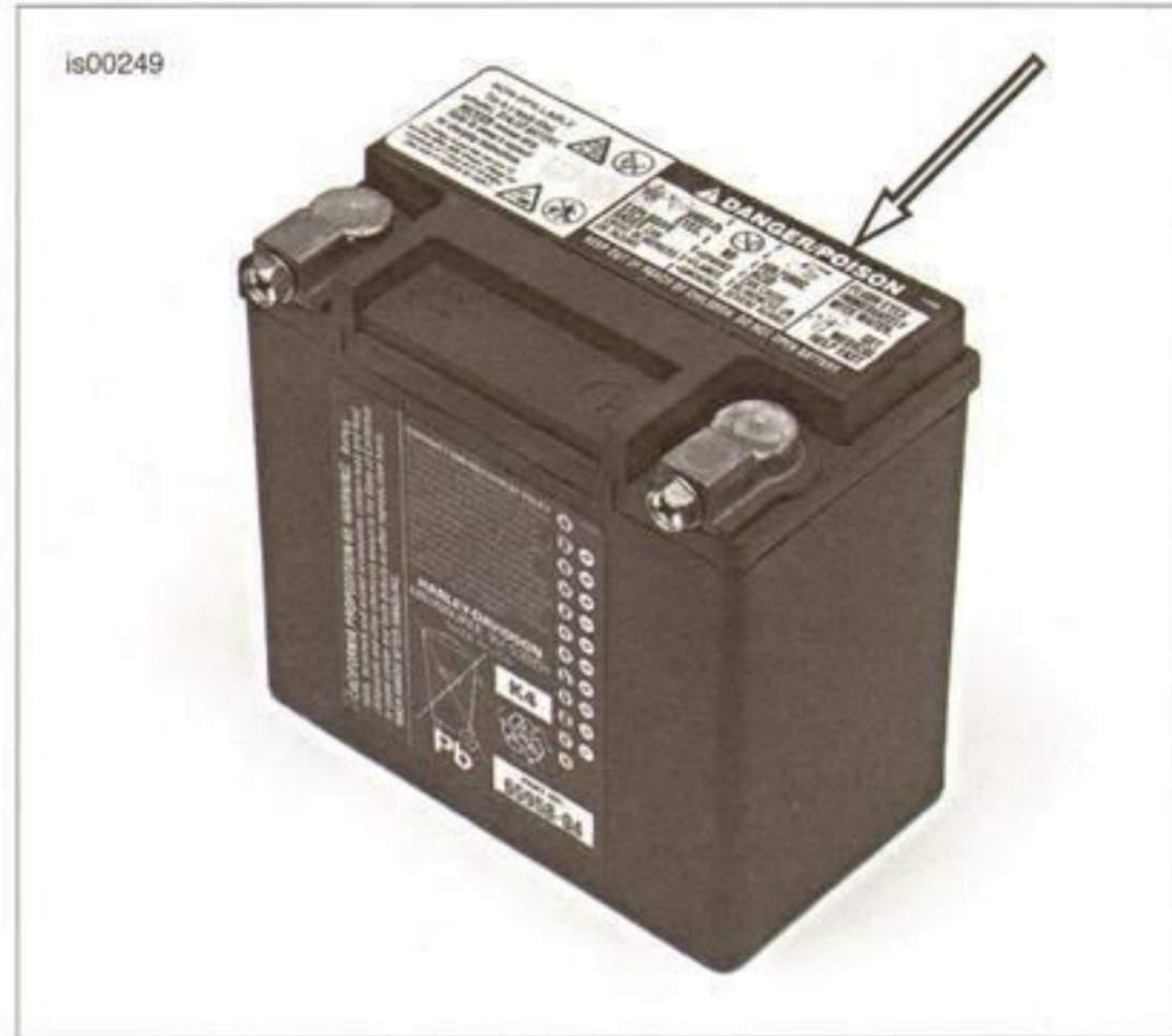
Figure 1-46. AGM Battery with Warning Label
