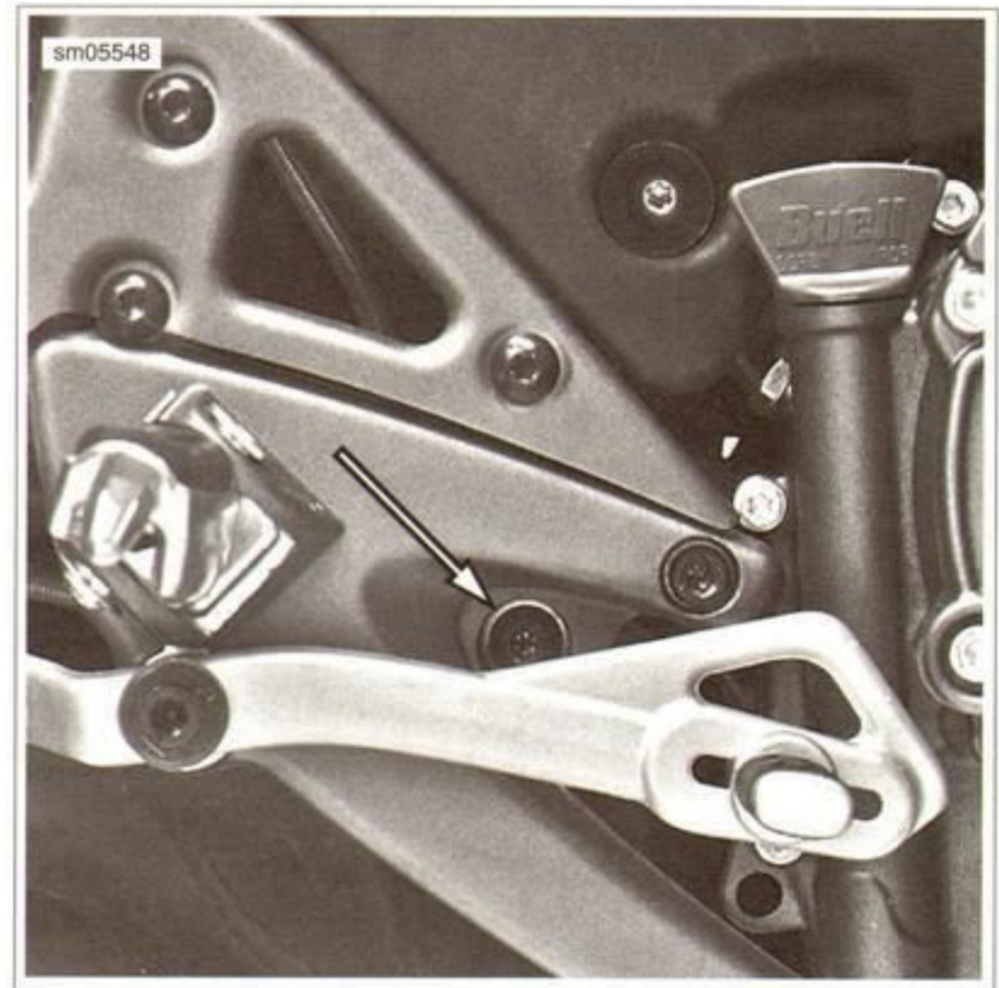
Figure 4-47. Muffler Bolt through Footpeg Mount
