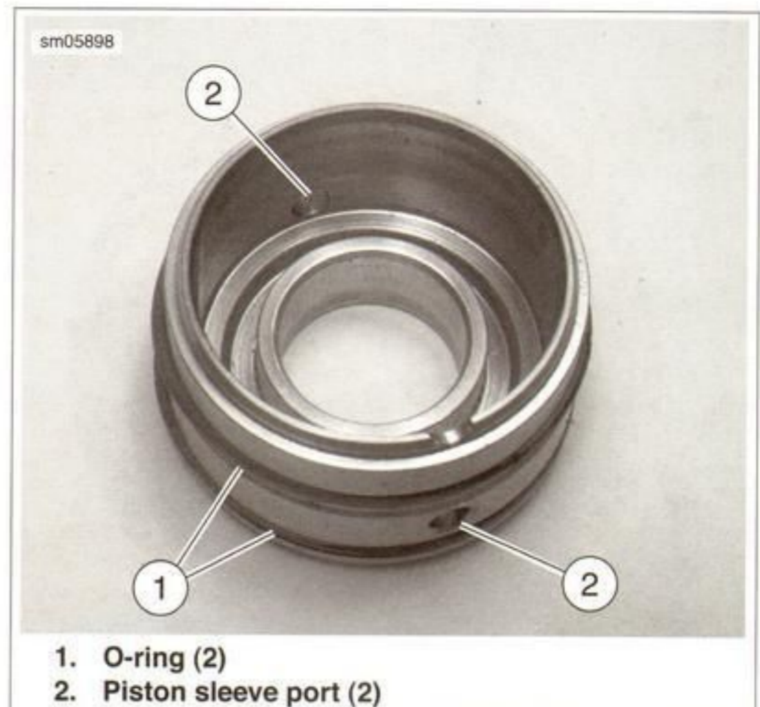
Figure 6-22. Piston Sleeve
