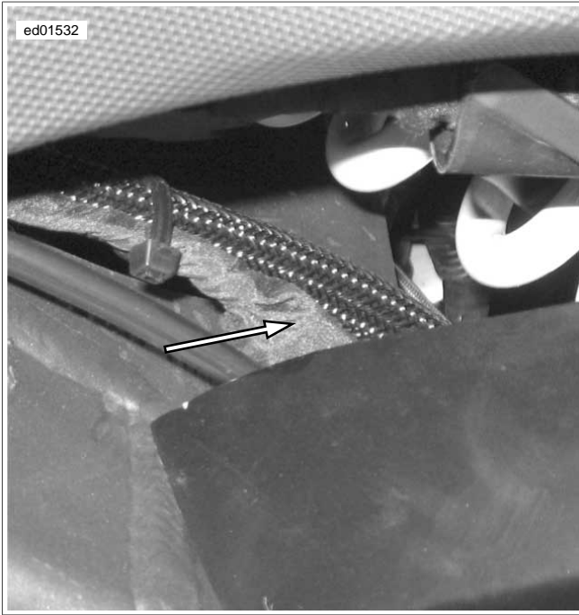
Figure 2-36. Fuel Pump Connector [86] (Lightning - swingarm removed for illustration)
