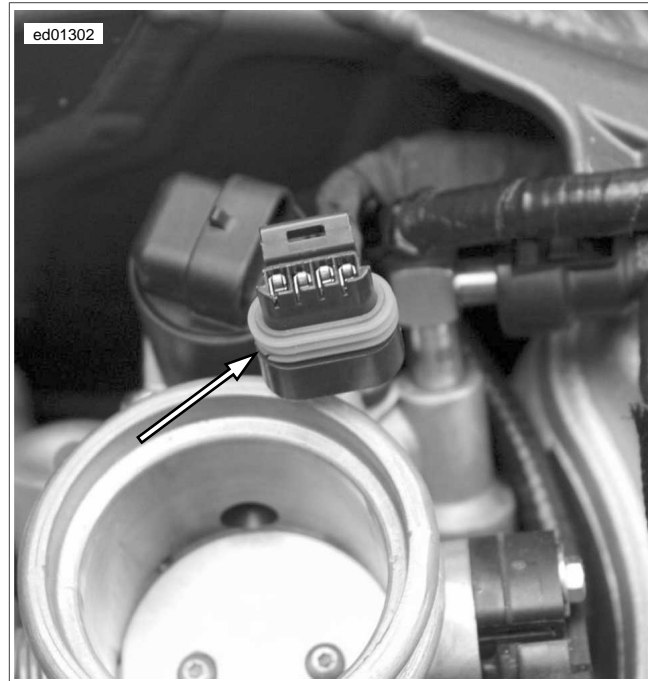
Figure 2-65. IAC Motor Connector
