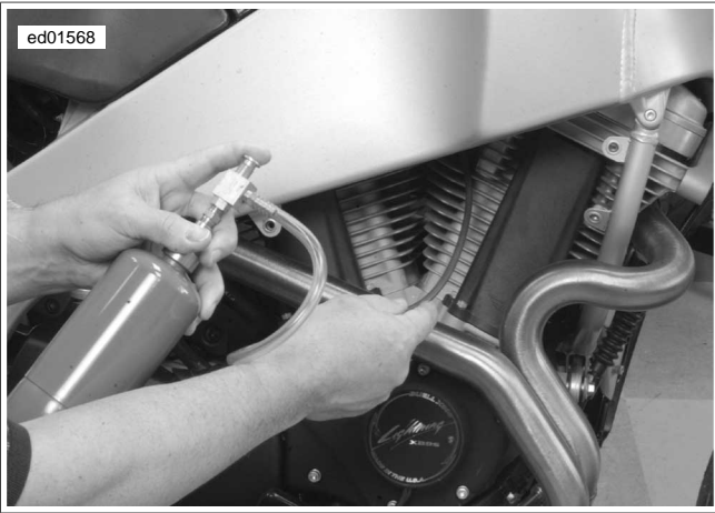
Figure 2-16. Checking for Leaks
