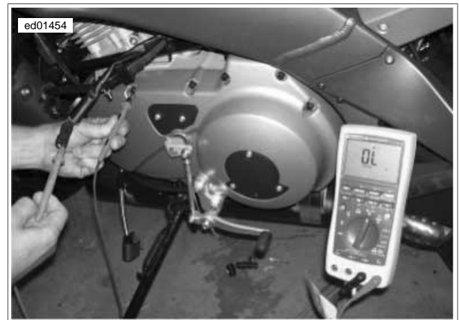
Figure 1-23. Test for Grounded Stator (Typical)
