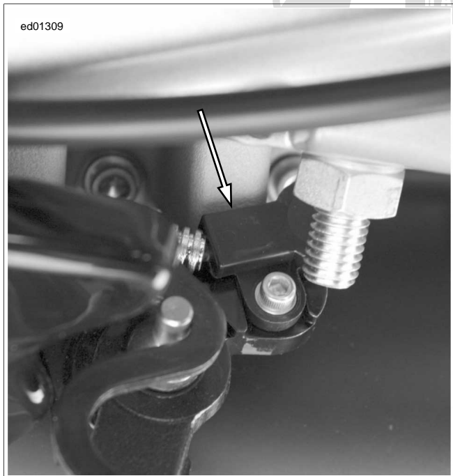
Figure 2-102. Side Stand Sensor
