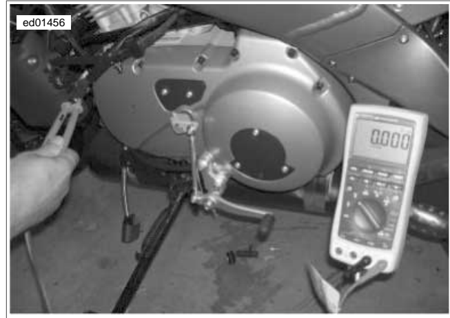
Figure 1-25. Check Stator AC Voltage Output (Typical)
