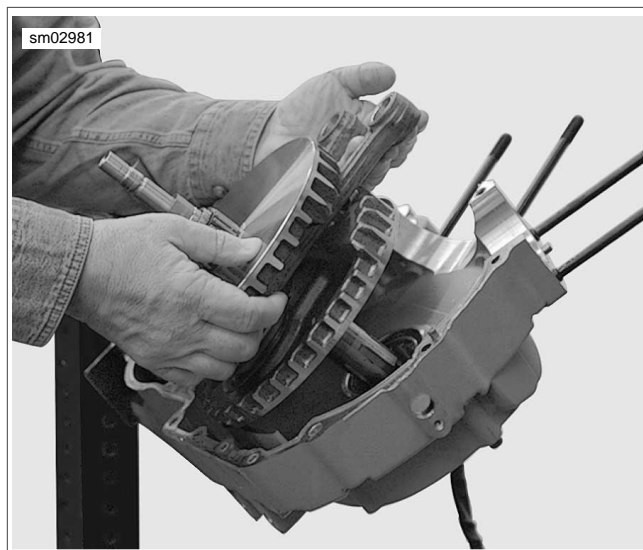
Figure 5-54. Removing Flywheels from Left Crankcase
