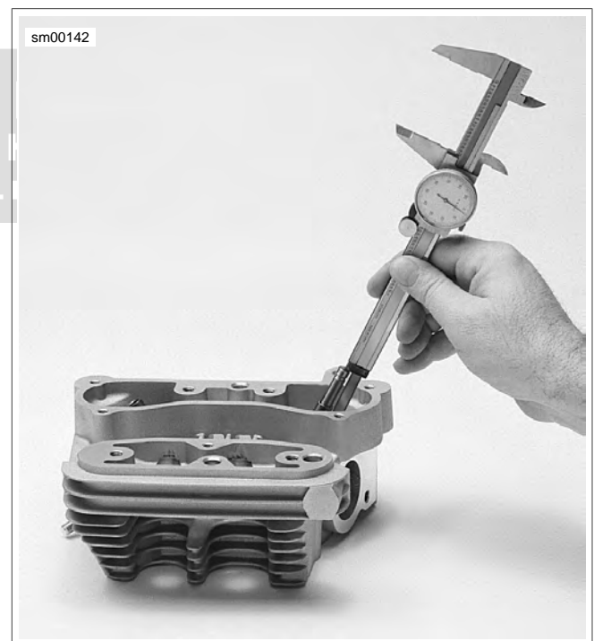
Figure 3-53. Measuring Valve Stem Protrusion
