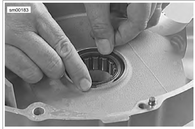
Figure 3-123. Removing Sprocket Shaft Bearing Retaining Ring
