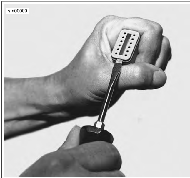
Figure A-13. Deutsch Connector: Remove Secondary Locking Wedge
