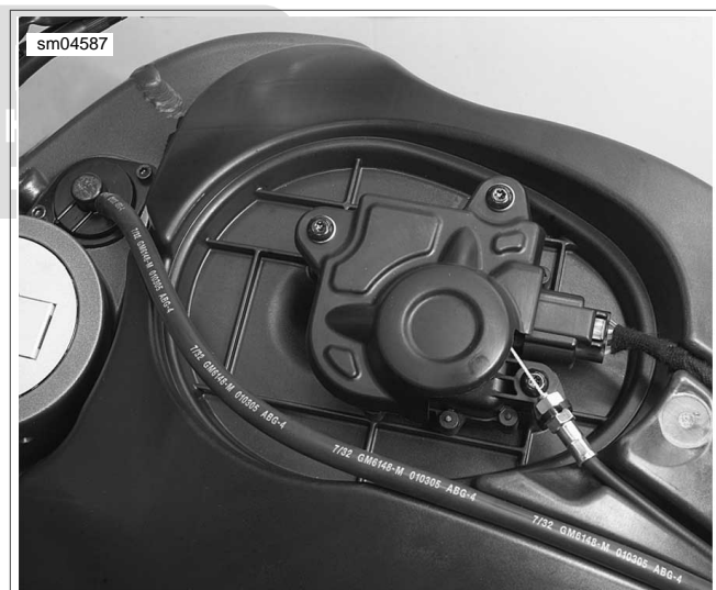
Figure 4-3. Interactive Exhaust Actuator to be used with Translucid Intake Cover (XB12)
