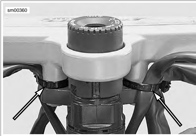
Figure 6-3. Cable Straps On Upper Fork Clamp: Firebolt
