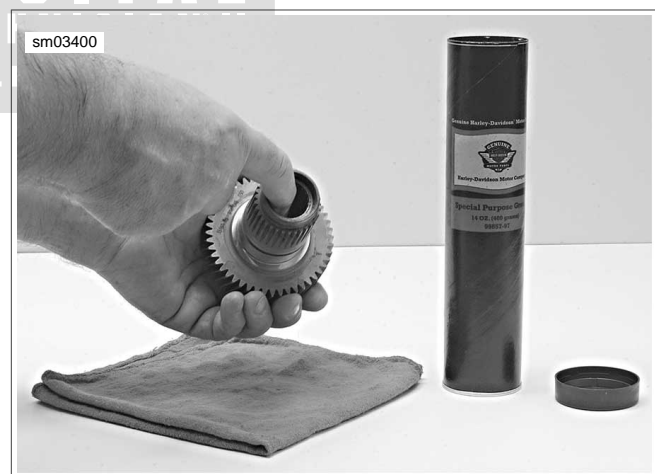
Figure 5-75. Lubricating Main Drive Gear Needle Bearing
