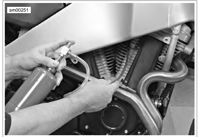
Figure 4-50. Checking for Intake Leak
