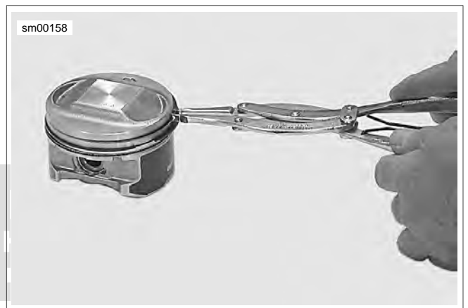
Figure 3-78. Installing Piston Rings Using Transmission Shaft Retaining Ring Pliers (Part No. J-5586-A)
