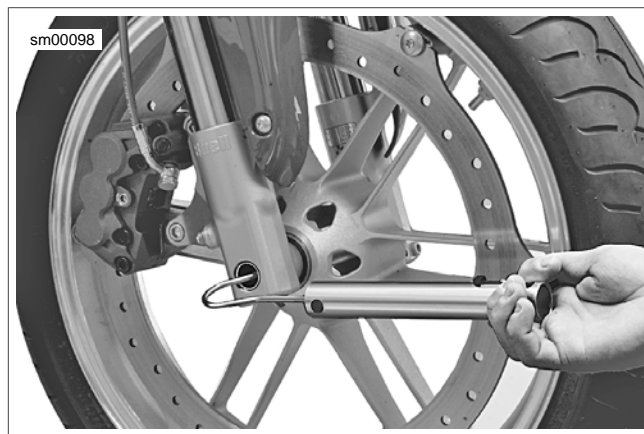
Figure 1-34. Measuring Steering Head Bearing Resistance (Typical)
