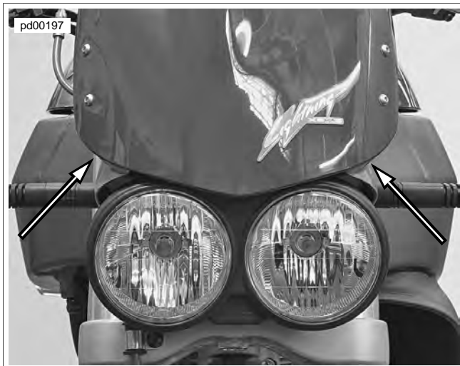
Figure 1-50. Horizontal Headlamp Adjustment Fastener Locations: Lightning
