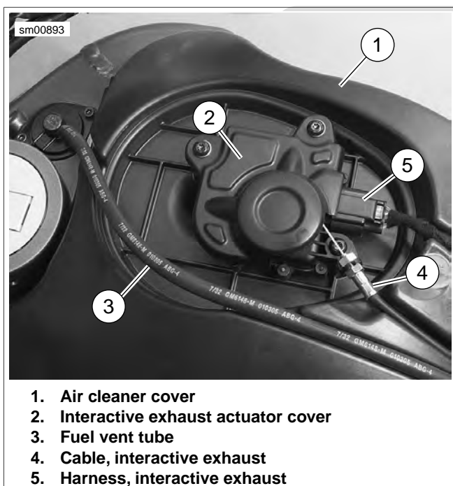
Figure 4-57. Air Cleaner Cover, Fuel Vent Tube and Fuel Vapor Valve (XB12 "Translucid" models)
