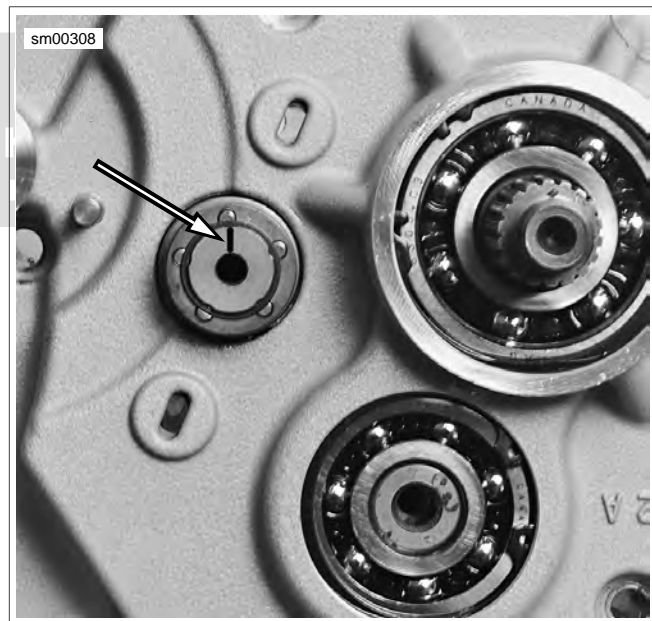
Figure 5-48. Shifter Drum and Mainshaft (Transmission in Neutral)
