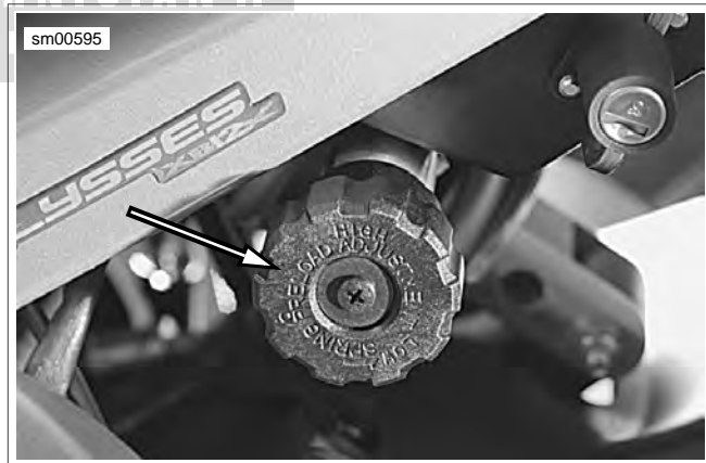
Figure 2-125. Rear Shock Absorber Preload Adjuster Knob: Ulysses
