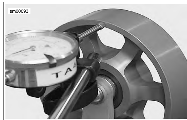
Figure 1-30. Measuring Lateral Side Play on Idler Pulley
