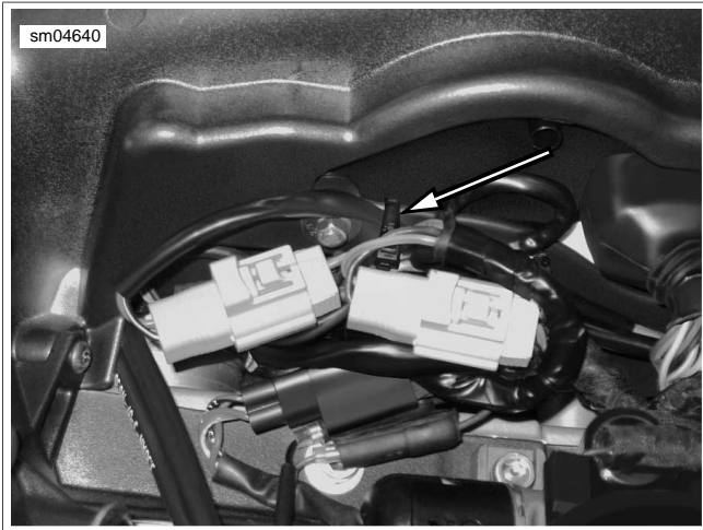
Figure 6-38. Location of Cable Strap Attached to Instrument Cluster
