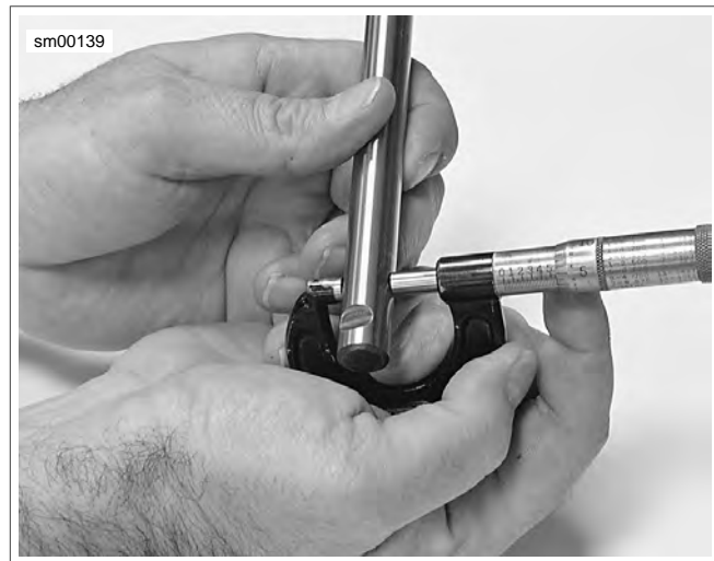
Figure 3-50. Measuring Rocker Arm Shaft Diameter (Rocker Arm Bushing Position)
