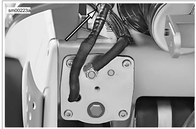
Figure 4-45. Fuel Pump Connector [86] (Swingarm removed for illustration)
