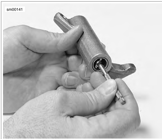
Figure 3-52. Measuring Rocker Arm Bushing Inner Diameter
