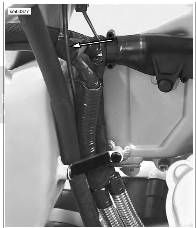
Figure 6-62. Interactive Exhaust Cable Behind Wire Harness Strap and Guide
