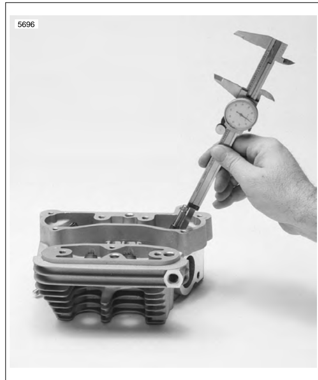
Figure 3-59. Measuring Valve Stem Protrusion
