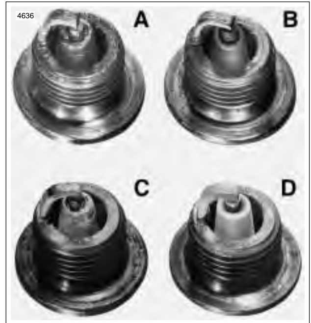
Figure 1-34. Typical Spark Plug Deposits
