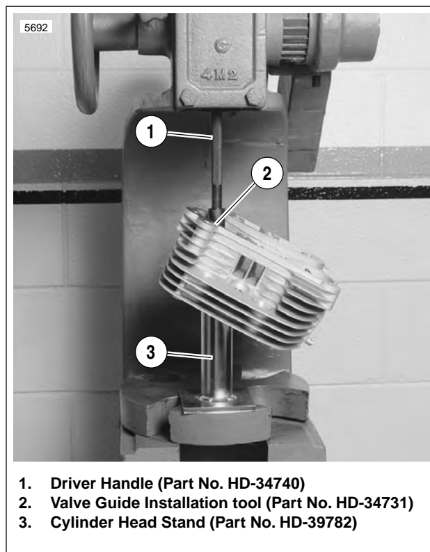
Figure 3-55. Installing Shoulderless Valve Guide
