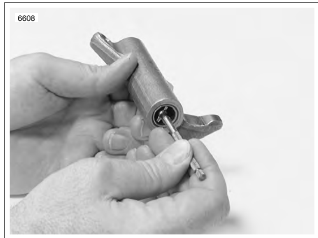
Figure 3-51. Measuring Rocker Arm Bushing Inner Diameter
