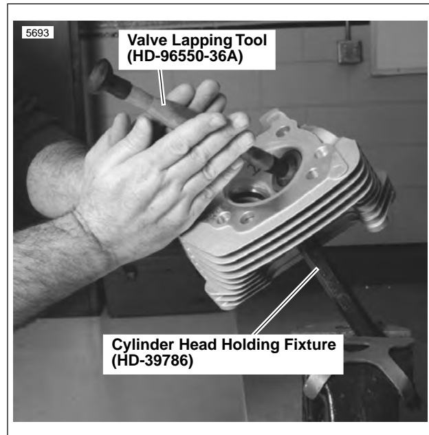
Figure 3-60. Lapping Valves
