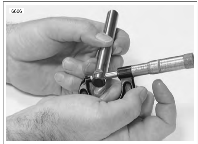
Figure 3-48. Measuring Rocker Arm Shaft Diameter (Rocker Cover Position)
