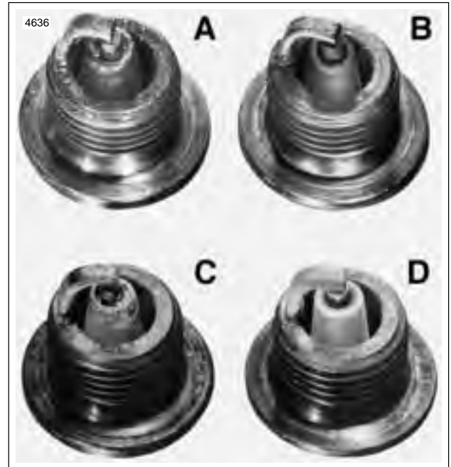
Figure 1-34. Typical Spark Plug Deposits
