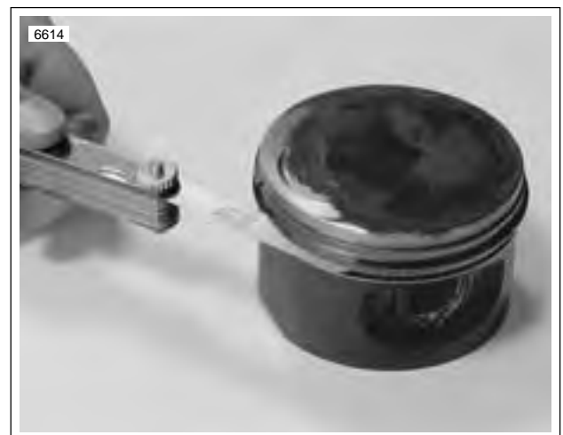
Figure 3-75. Measuring Ring Clearance in Groove
