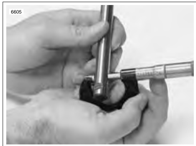
Figure 3-49. Measuring Rocker Arm Shaft Diameter (Rocker Arm Bushing Position)
