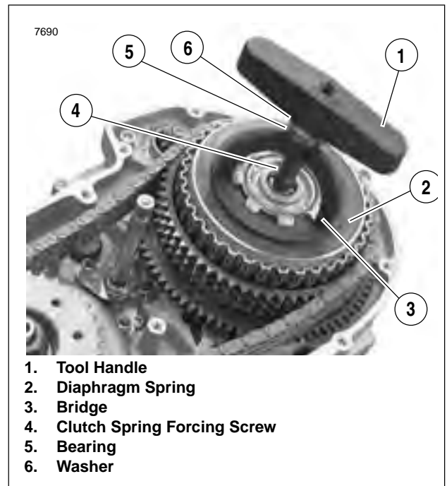
Figure 6-20. Compressing Clutch Diagram Spring
