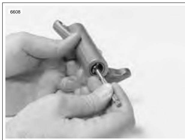
Figure 3-51. Measuring Rocker Arm Bushing Inner Diameter
