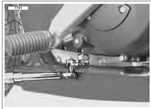
Figure 1-23. Tightening Chain Limiting Screw
