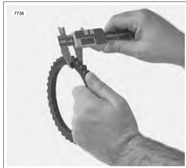
Figure 6-25. Measuring Friction Plates
