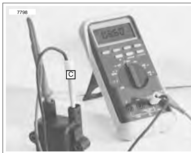
Figure 7-26. Ignition Coil Secondary Resistance Test
