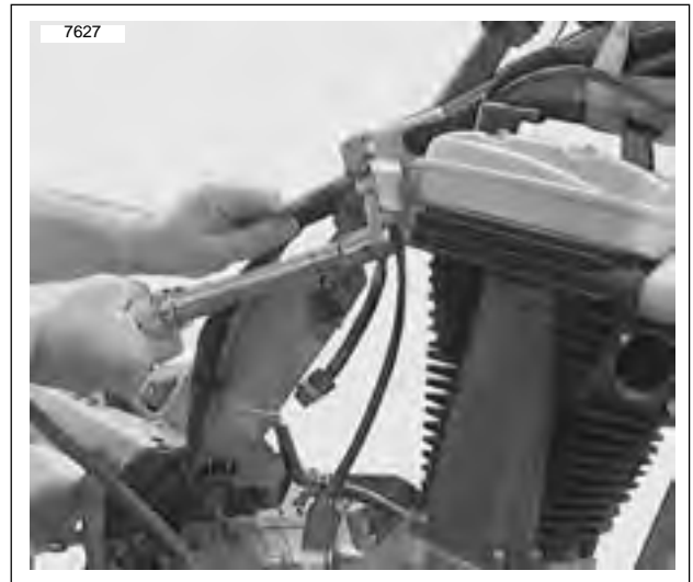
Figure 3-38. Install Top Rear Tie Bar
