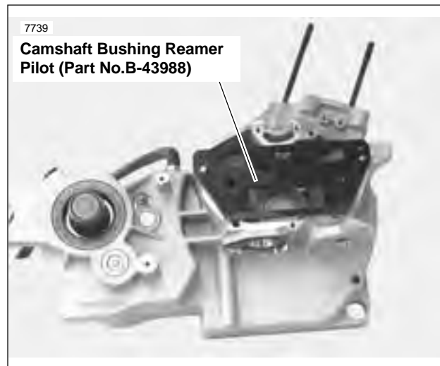
Figure 3-107. Reaming Cam Gear Bushing in Right Crankcase Half
