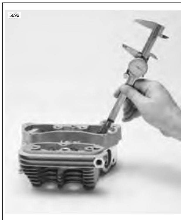
Figure 3-59. Measuring Valve Stem Protrusion
