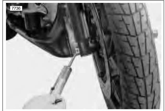
Figure 1-33. Steering Head Bearing Check
