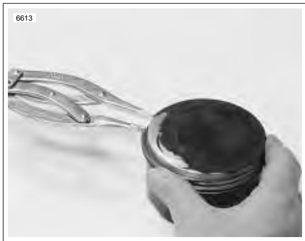
Figure 3-77. Installing Piston Rings using Transmission Shaft Retaining Ring Pliers (Part No. J-5586)
