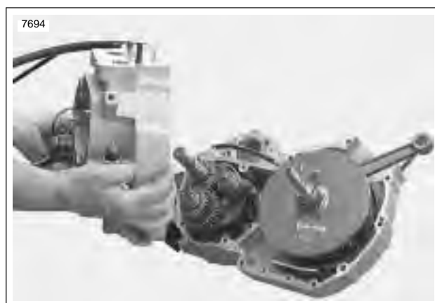
Figure 6-27. Splitting Crankcase Halves
