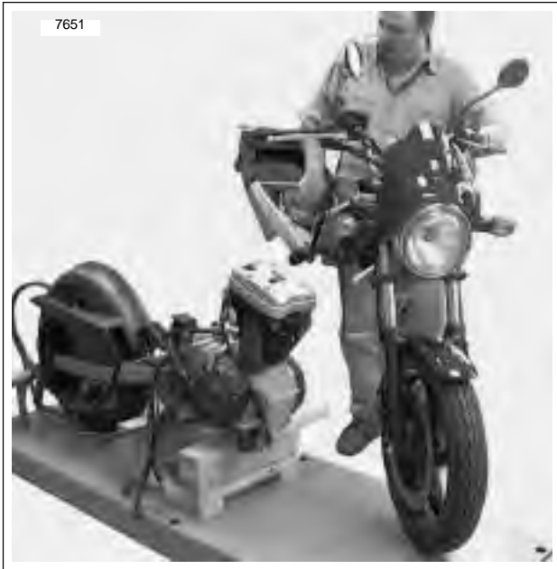
Figure 3-15. Move Chassis From Engine
