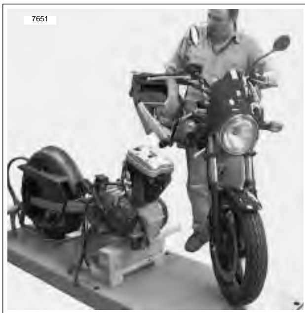
Figure 3-26. Move Chassis to Engine
