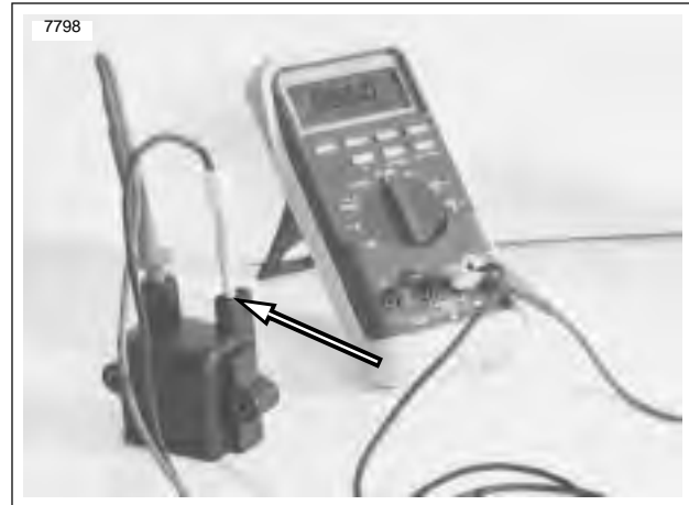
Figure 7-26. Ignition Coil Secondary Resistance Test at Terminal C
