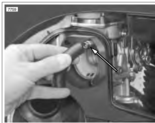
Figure 1-38. Fix Hose End Onto Allen Head Screw
