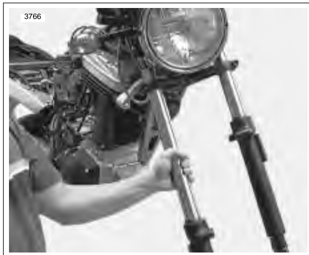
Figure 2-95. Installing Fork Tube
