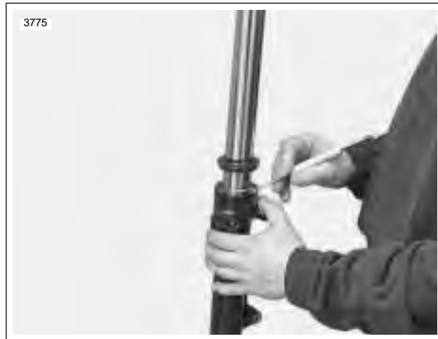
Figure 2-74. Removing Dust Seal
