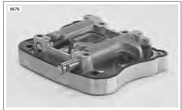
Figure 3-46. Removing Rocker Arm Shafts
