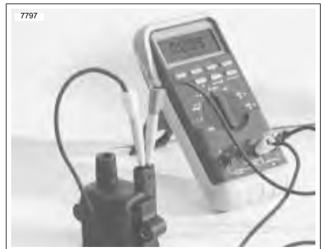
Figure 7-25. Ignition Coil Primary Resistance Test
