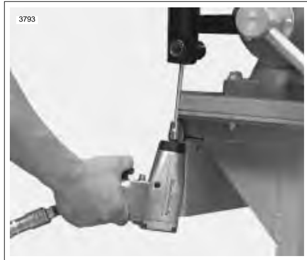
Figure 2-85. Install Center Bolt
