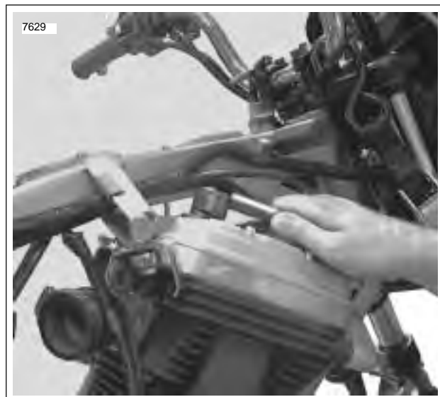
Figure 3-42. Install Crankcase Breather Hose
