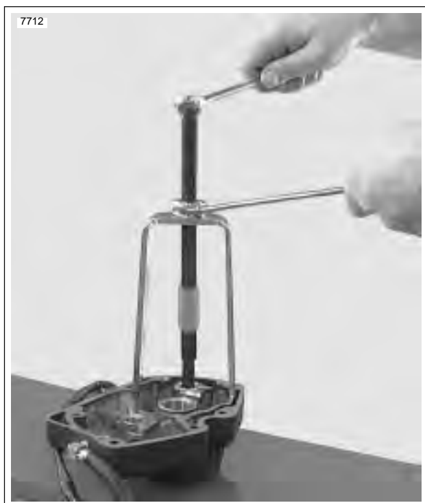
Figure 3-107. Removing Bushing with Bushing and Bearing Puller (Part No. HD-95760-69A)
