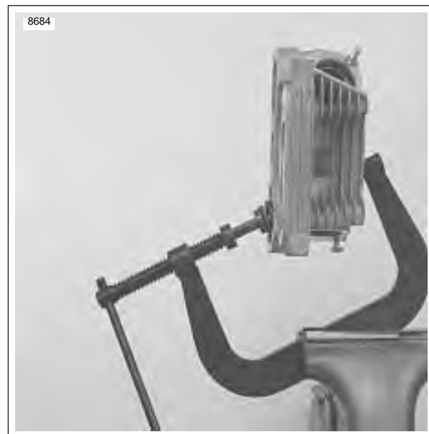
Figure 3-48. Valve Spring Compressor (Part No. HD-34736B)
