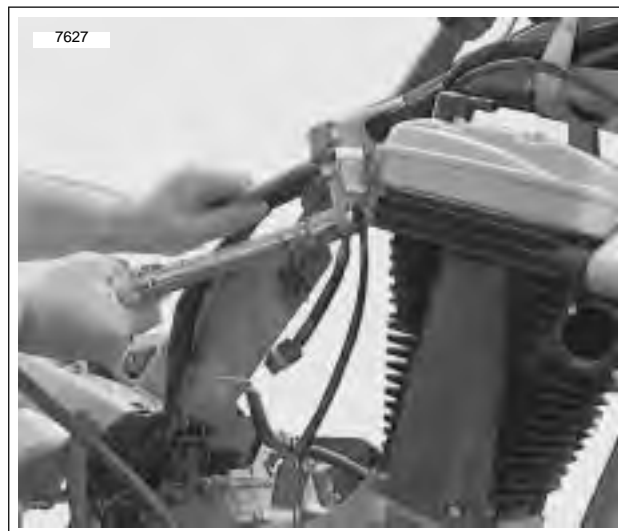
Figure 3-4. Remove Top Rear Tie Bar
