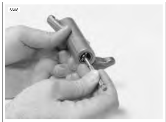
Figure 3-54. Measuring Rocker Arm Bushing Inner Diameter
