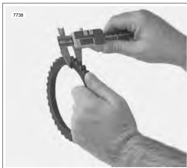
Figure 6-17. Measuring Friction Plates
