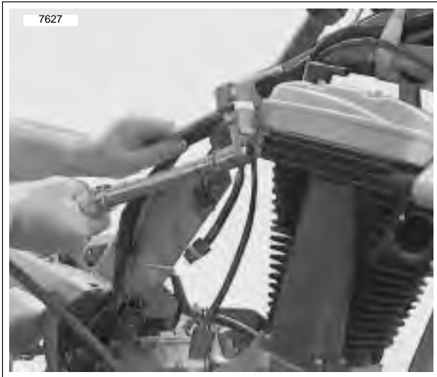
Figure 3-38. Install Top Rear Tie Bar
