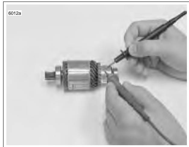
Figure 5-22. Open Armature Test
