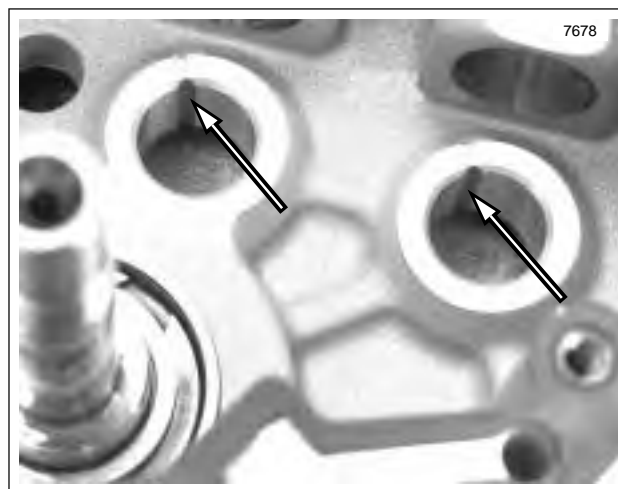
Figure 3-108. Cam Gear Bushing Installed in Crankcase
