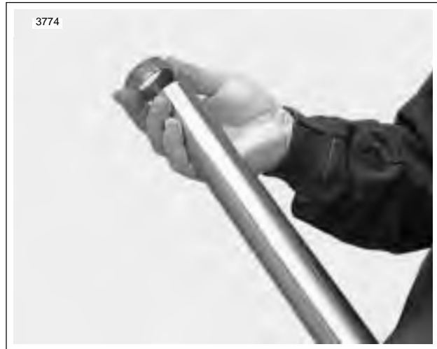
Figure 2-86. Install Guide Bushing
