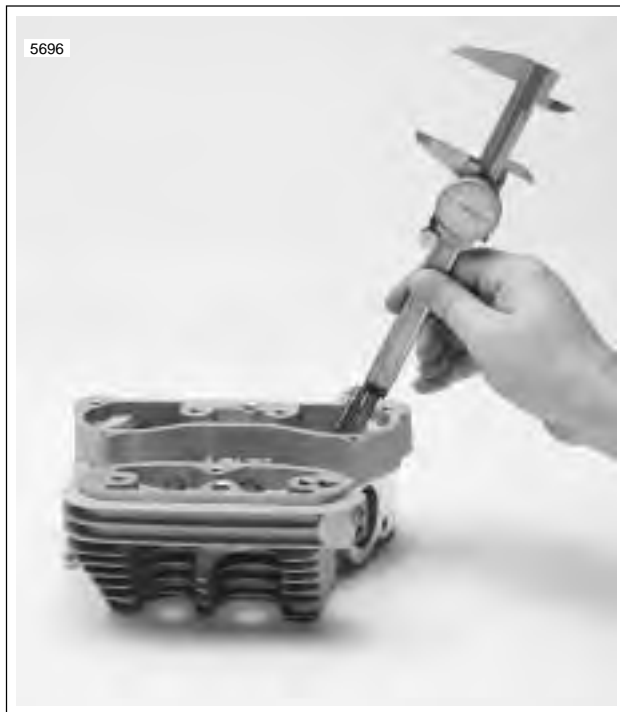
Figure 3-55. Measuring Valve Stem Protrusion
