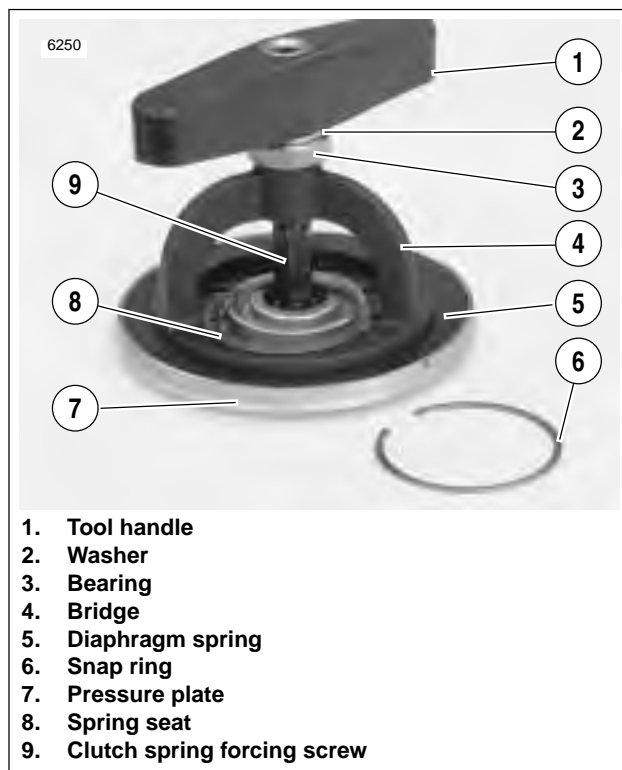
Figure 6-13. Pressure Plate Assembly
