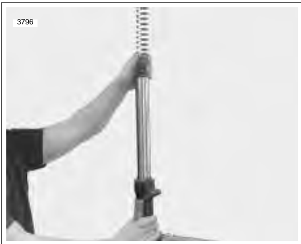
Figure 2-84. Install Rebound Spring
