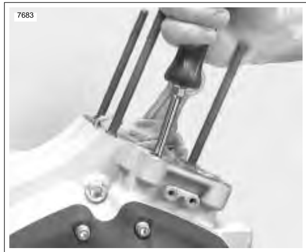
Figure 3-118. Checking Cam Gear End Play
