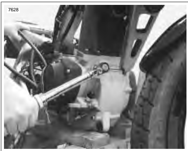
Figure 3-39. Install Front Tie Bar
