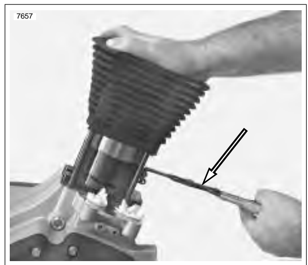
Figure 3-89. Compressing Piston Rings Using Piston Ring Compressor (Part No. HD-96333-51C)
