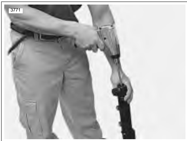
Figure 2-72. Removing Center Bolt
