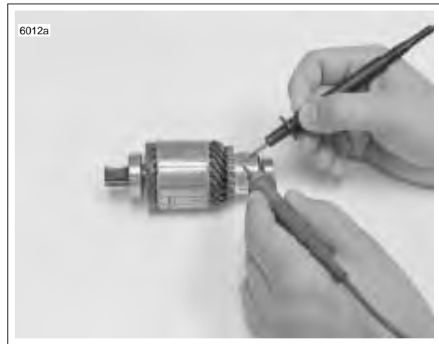
Figure 5-22. Open Armature Test
