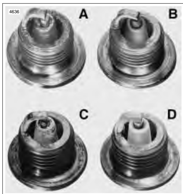
Figure 1-35. Typical Spark Plug Deposits
