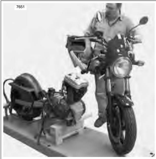
Figure 3-15. Move Chassis From Engine
