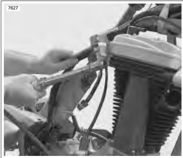
Figure 3-38. Install Top Rear Tie Bar
