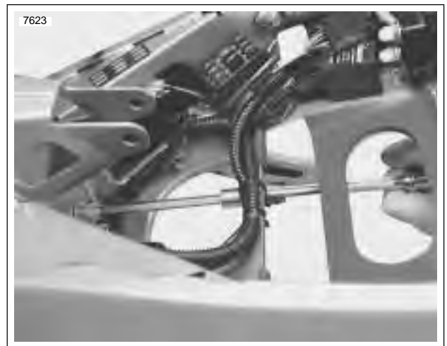
Figure 3-14. Removing Rear Motor Mount Bolts
