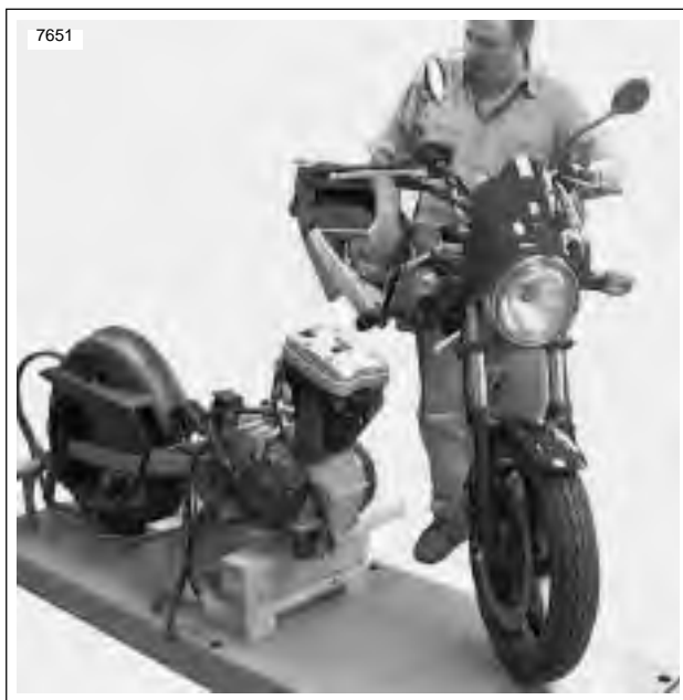
Figure 3-26. Move Chassis to Engine
