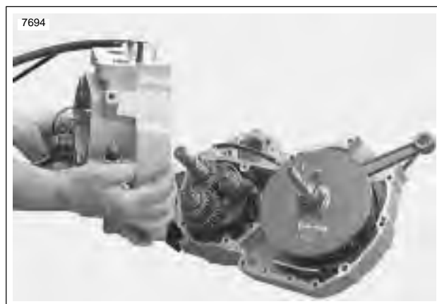
Figure 6-27. Splitting Crankcase Halves
