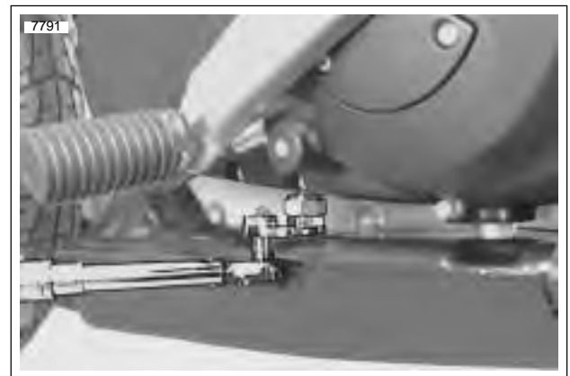
Figure 1-24. Tightening Chain Limiting Screw
