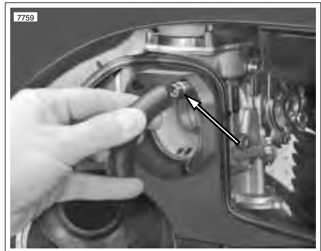
Figure 1-38. Fix Hose End Onto Allen Head Screw
