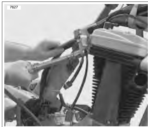
Figure 3-4. Remove Top Rear Tie Bar
