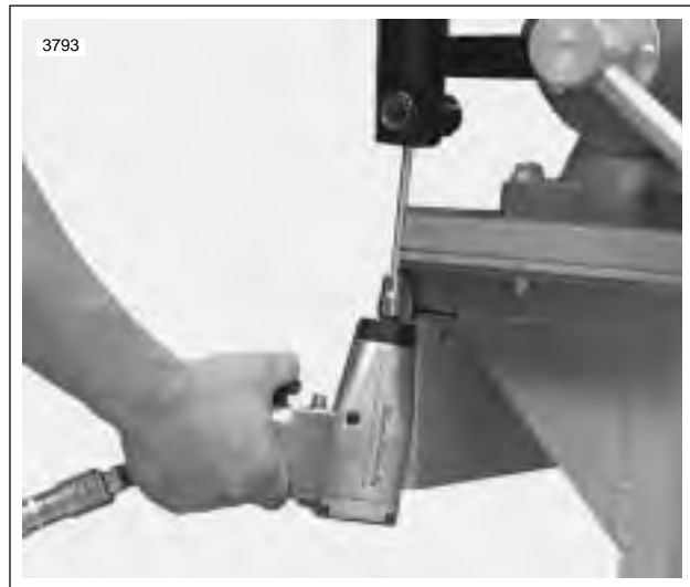
Figure 2-85. Install Center Bolt
