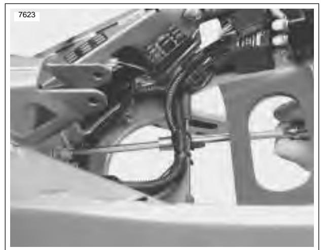
Figure 3-28. Installing Rear Motor Mount Bolts
