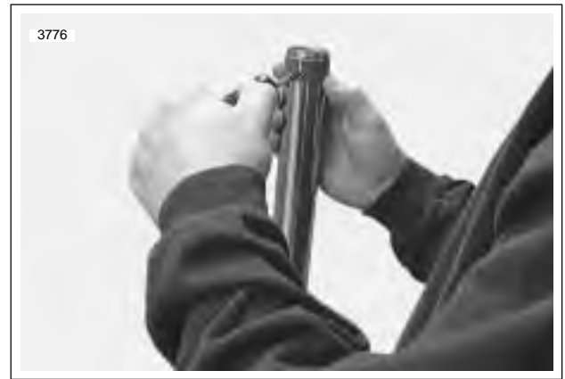
Figure 2-76. Removing Slide Bushing
