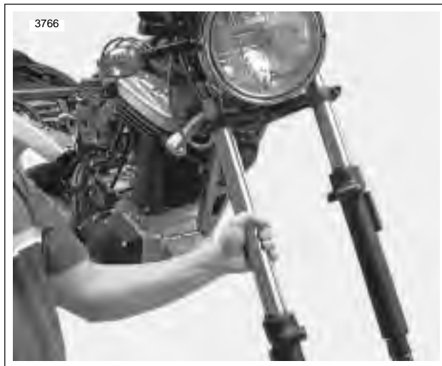
Figure 2-95. Installing Fork Assemblies
