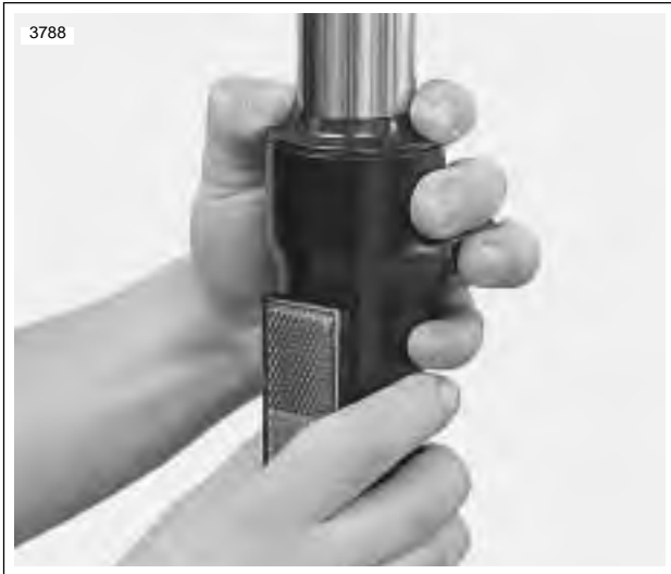
Figure 2-91. Install New Dust Seal
