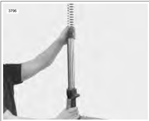
Figure 2-84. Install Rebound Spring
