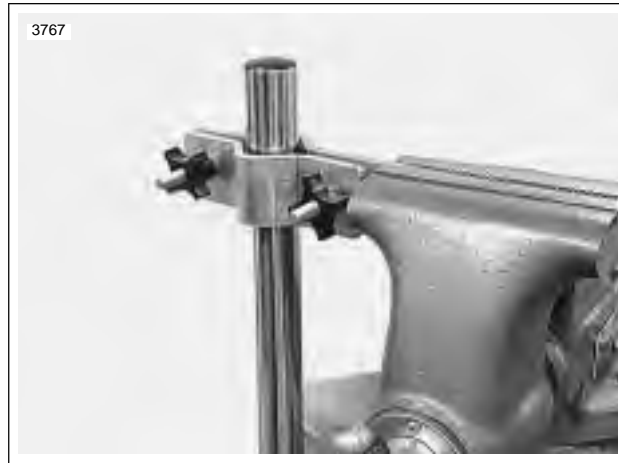
Figure 2-67. Clamping the Fork
