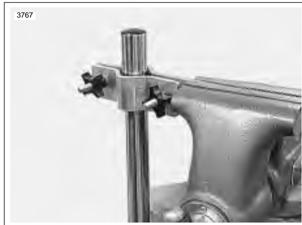
Figure 1-26. Clamping the Fork
