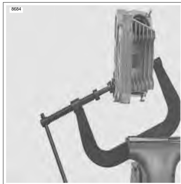
Figure 3-48. Valve Spring Compressor (Part No. HD-34736B)
