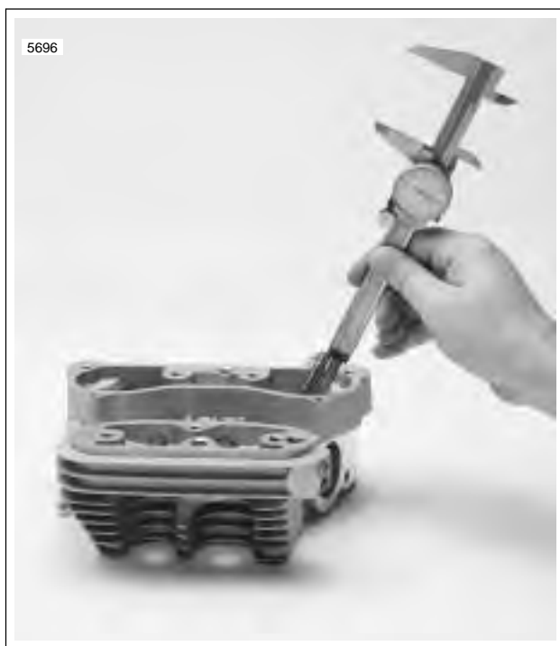
Figure 3-55. Measuring Valve Stem Protrusion
