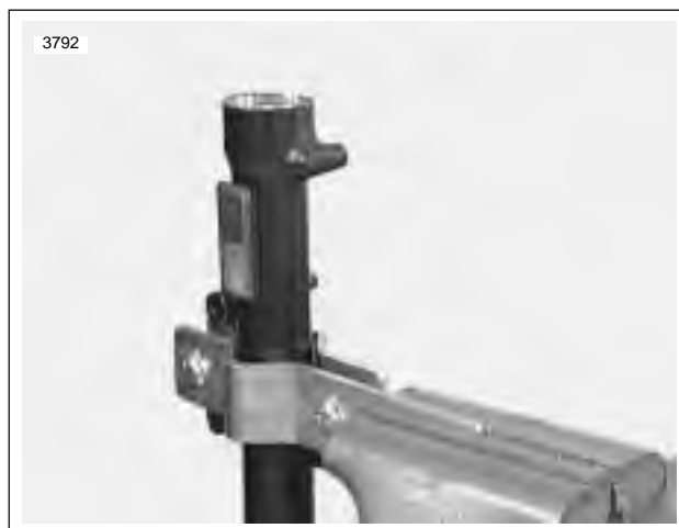
Figure 2-82. Clamping the Slider Assembly
