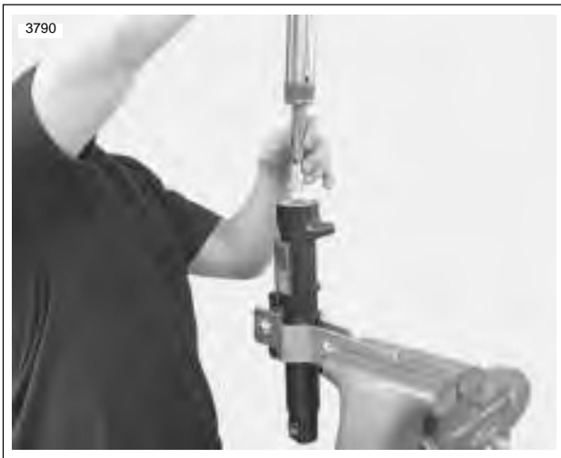
Figure 2-83. Installing Slider Tube
