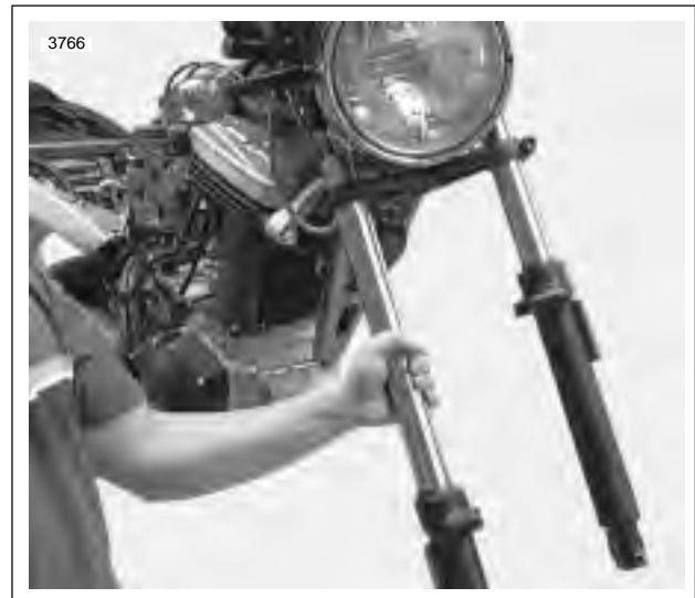
Figure 2-66. Front Fork Removal
