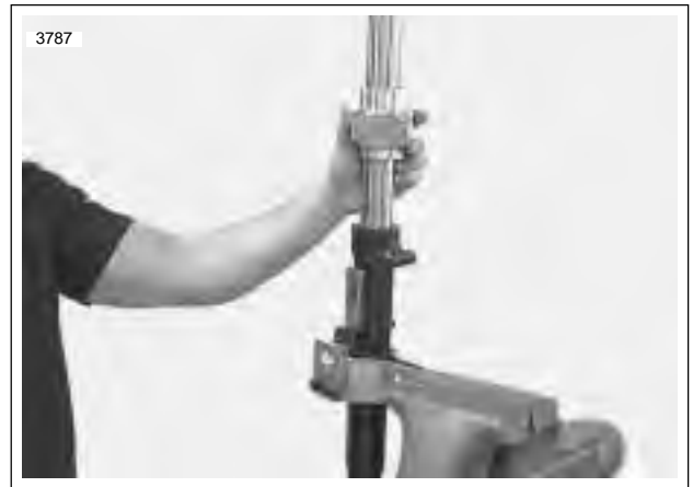
Figure 2-89. Fork Seal Driver
