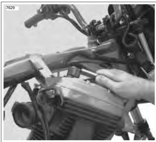
Figure 3-1. Remove Crankcase Breather Hose
