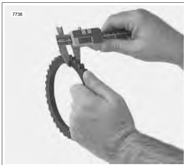
Figure 6-17. Measuring Friction Plates
