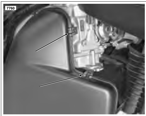
Figure 1-36. Release Air Box Cover Latches
