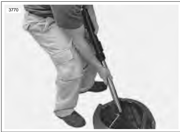
Figure 2-71. Pumping Fork Oil
