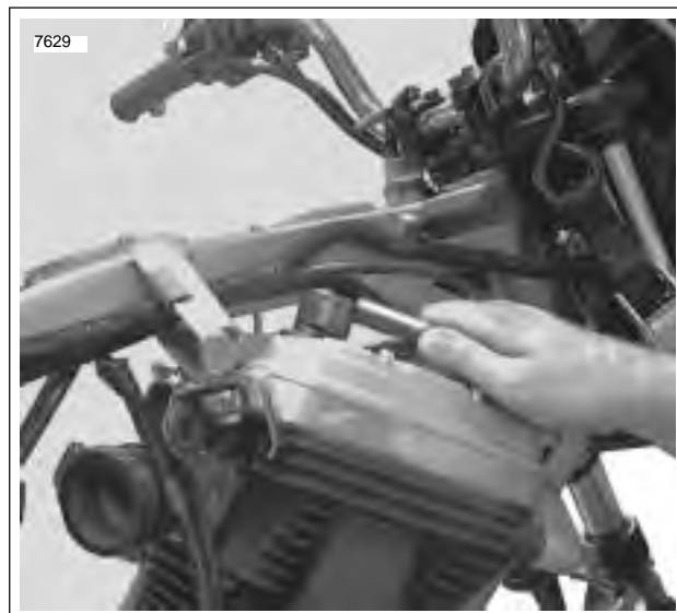
Figure 3-42. Install Crankcase Breather Hose
