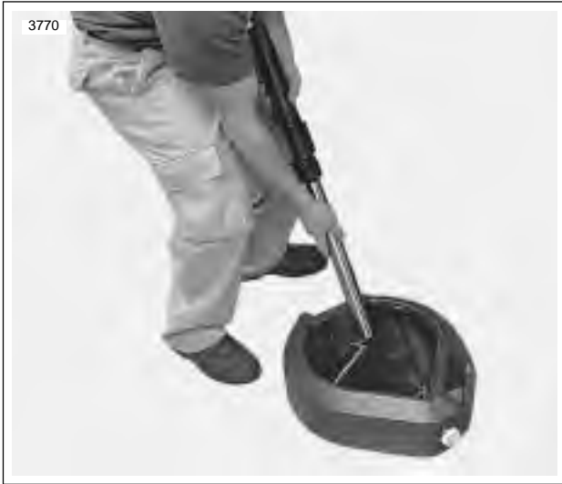
Figure 1-30. Pumping Fork Oil
