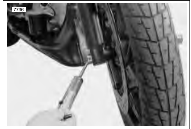
Figure 1-33. Steering Head Bearing Check
