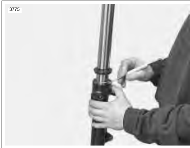
Figure 2-74. Removing Dust Seal
