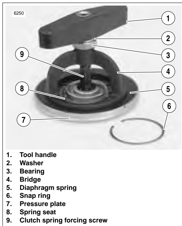
Figure 6-13. Pressure Plate Assembly
