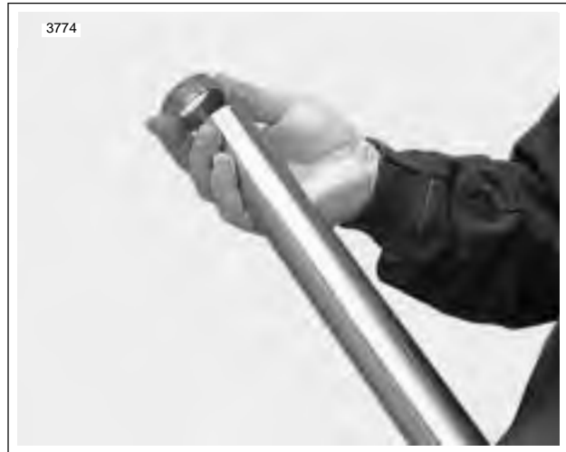
Figure 2-86. Install Guide Bushing
