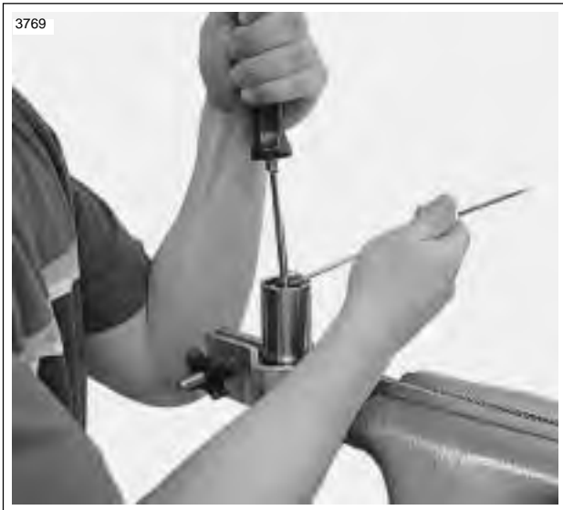
Figure 1-31. Compressing Spring Seat
