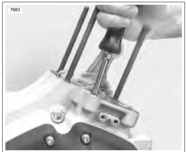
Figure 3-110. Checking Cam Gear End Play
