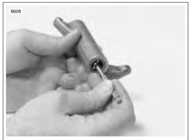
Figure 3-54. Measuring Rocker Arm Bushing Inner Diameter
