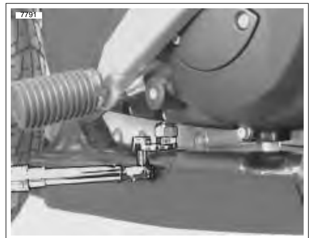
Figure 6-6. Torquing Chain Limiting Screw
