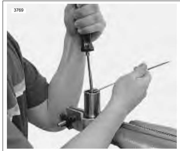
Figure 2-93. Compressing Spring Seat to Install Stopper Ring
