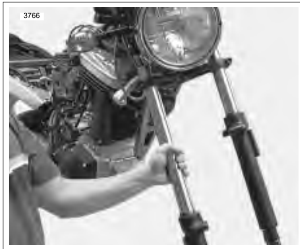
Figure 2-95. Installing Fork Assemblies
