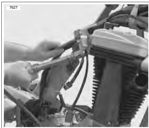
Figure 3-4. Remove Top Rear Tie Bar
