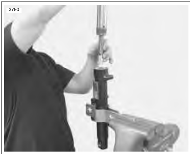
Figure 2-83. Installing Slider Tube
