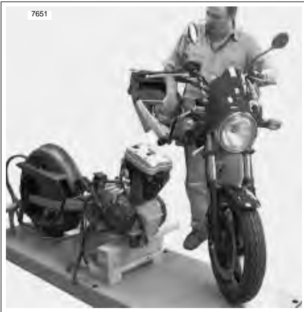
Figure 3-15. Move Chassis From Engine
