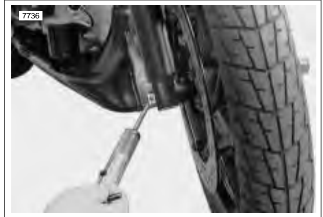
Figure 1-33. Steering Head Bearing Check
