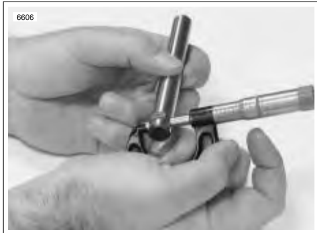
Figure 3-51. Measuring Rocker Arm Shaft Diameter (Rocker Cover Position)
