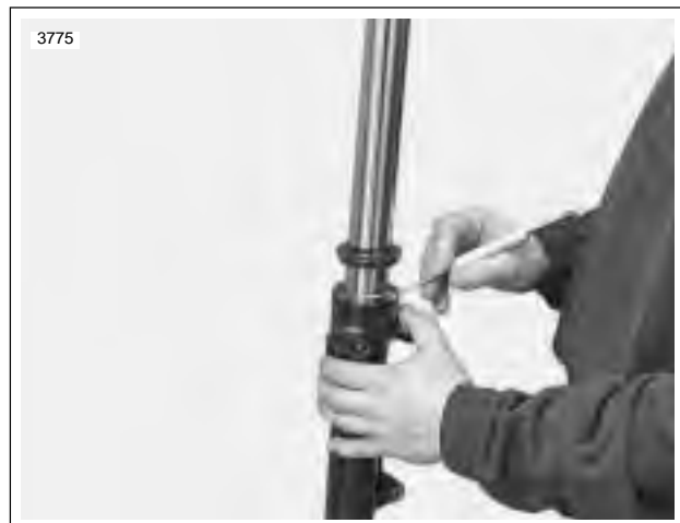
Figure 2-74. Removing Dust Seal
