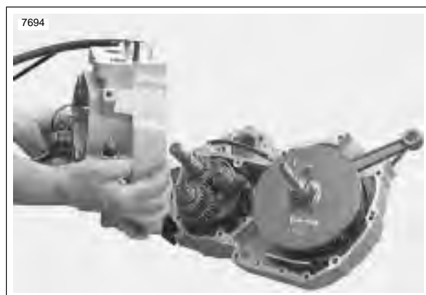
Figure 6-27. Splitting Crankcase Halves
