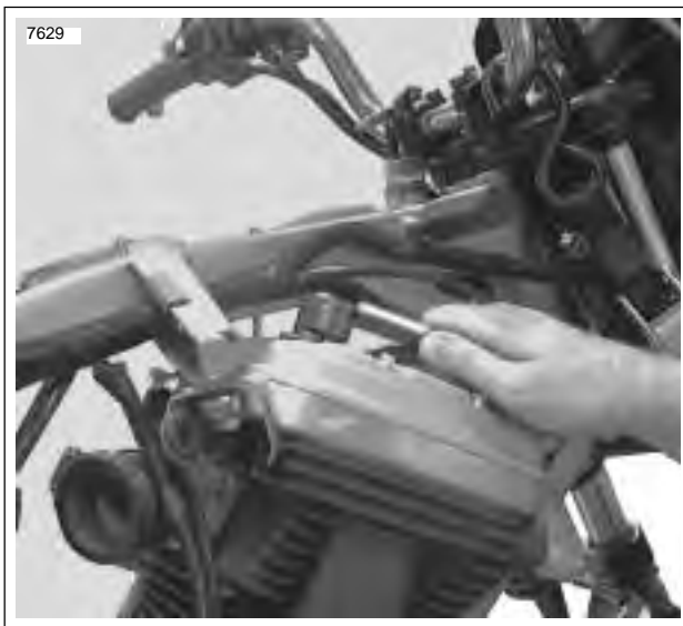
Figure 3-1. Remove Crankcase Breather Hose
