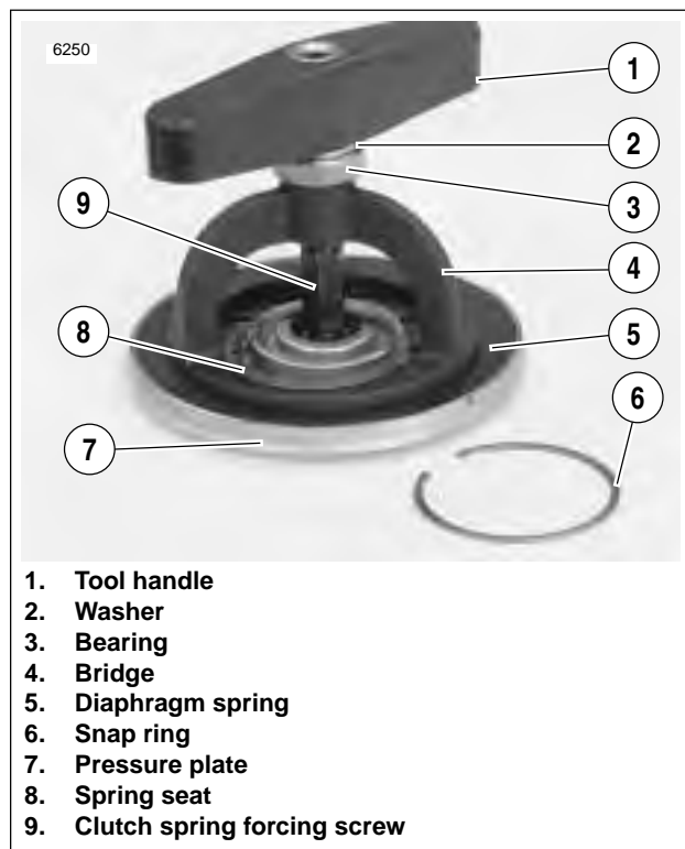
Figure 6-13. Pressure Plate Assembly
