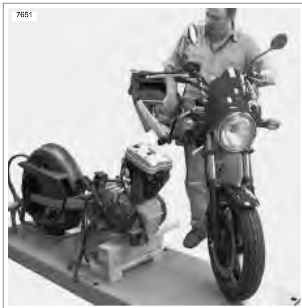
Figure 3-26. Move Chassis to Engine
