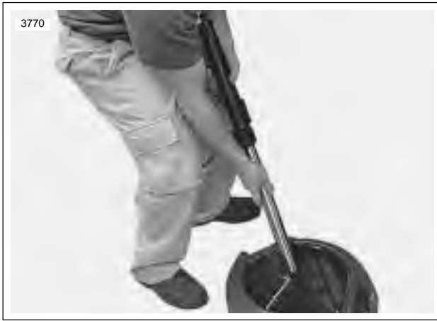
Figure 2-71. Pumping Fork Oil
