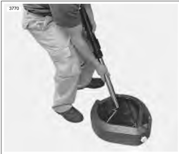
Figure 1-30. Pumping Fork Oil
