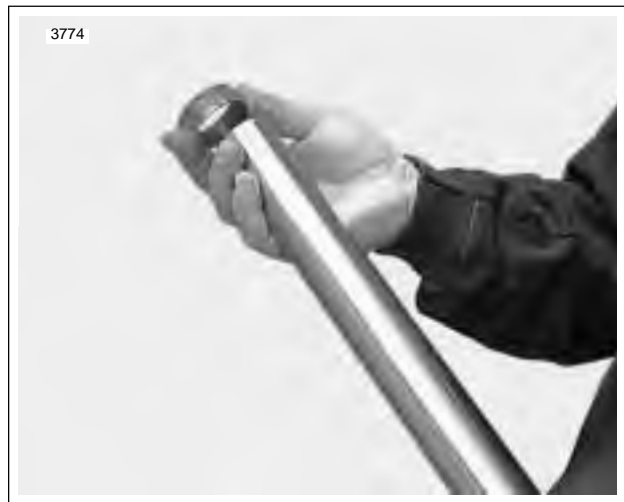
Figure 2-86. Install Guide Bushing
