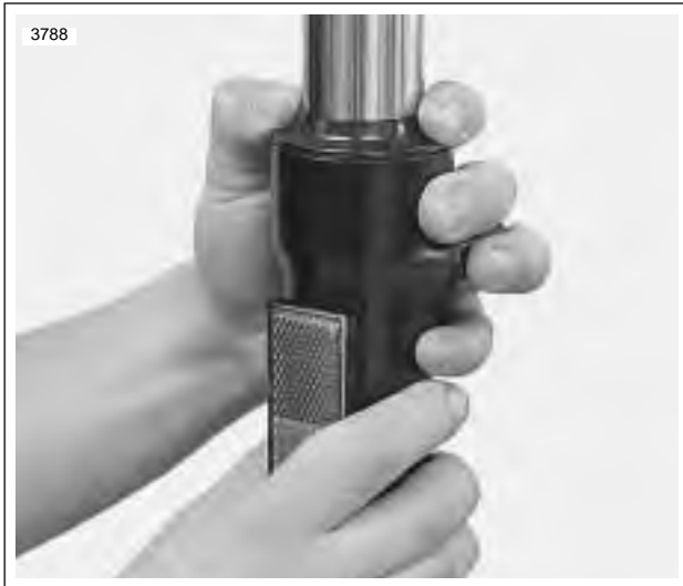
Figure 2-91. Install New Dust Seal
