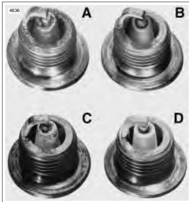
Figure 1-35. Typical Spark Plug Deposits
