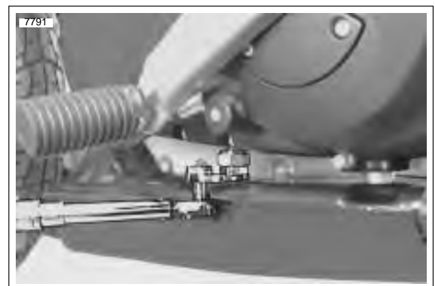
Figure 1-24. Tightening Chain Limiting Screw
