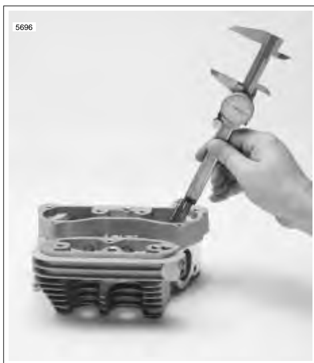
Figure 3-55. Measuring Valve Stem Protrusion
