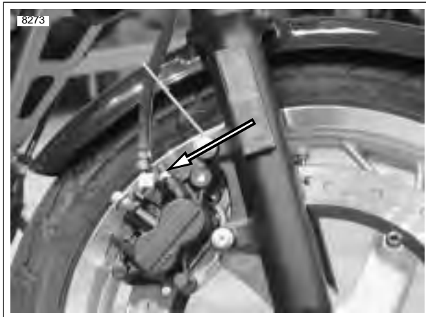
Figure 2-26. Front Brake Caliper Bleeder Valve (Metric) for Draining Front Brake System
