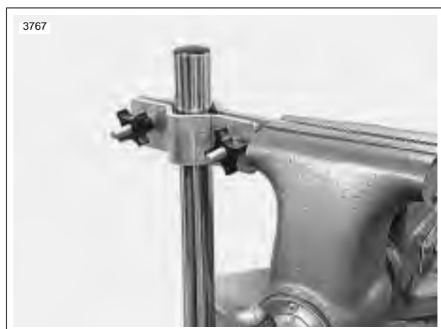
Figure 2-67. Clamping the Fork
