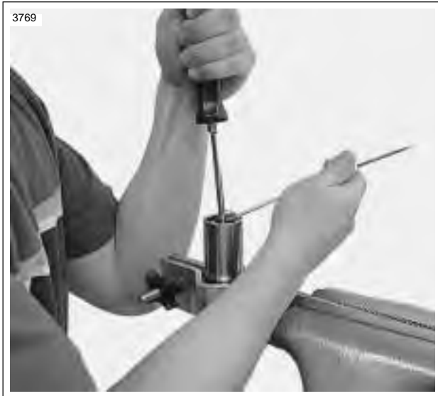
Figure 1-31. Compressing Spring Seat
