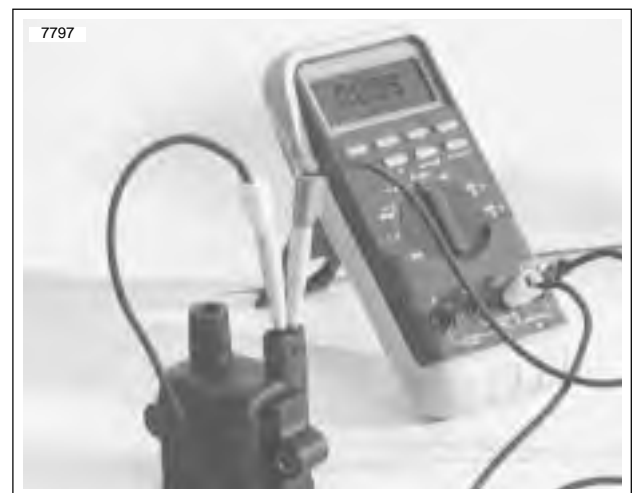
Figure 7-25. Ignition Coil Primary Resistance Test
