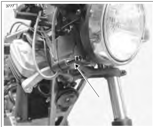
Figure 2-96. Location of Anti-Seize on Triple Clamp Pinch Screws
