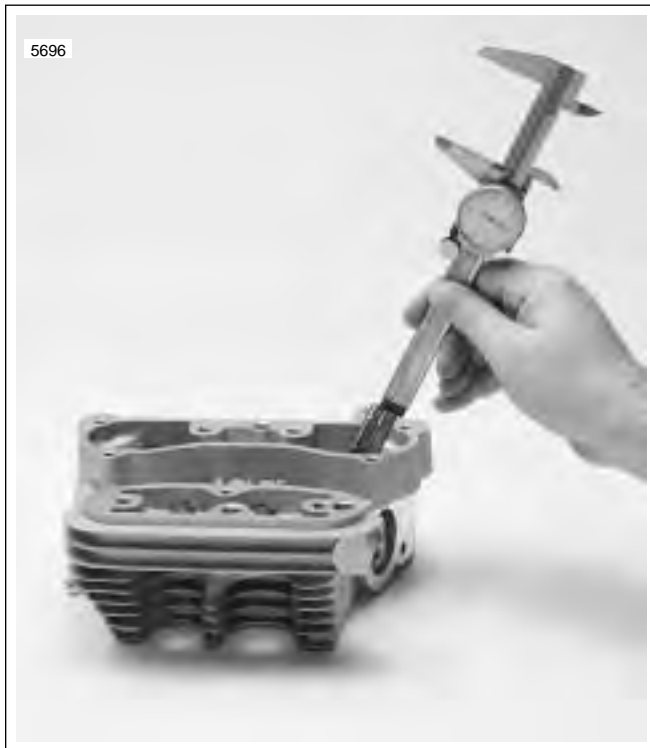
Figure 3-55. Measuring Valve Stem Protrusion
