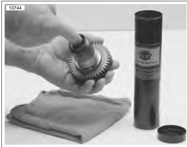
Figure 6-41. Lubricating Main Drive Gear Needle Bearings
