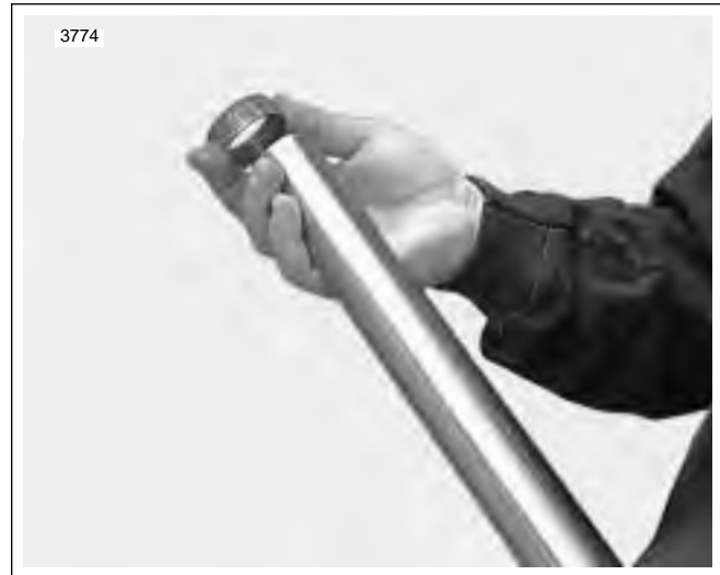
Figure 2-86. Install Guide Bushing
