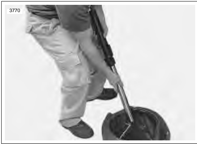
Figure 2-71. Pumping Fork Oil
