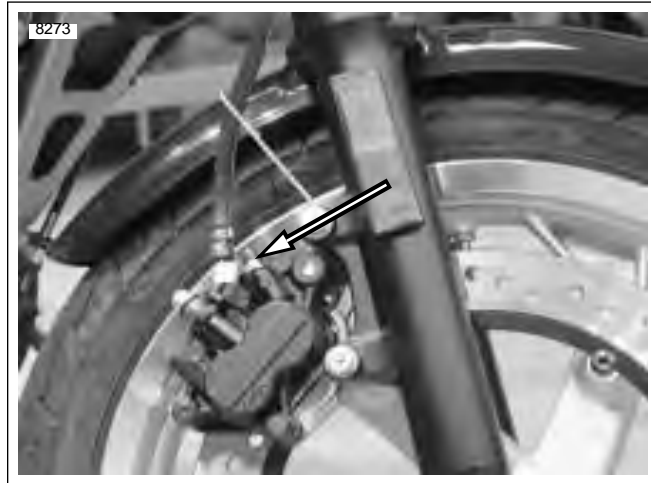
Figure 2-27. Front Brake Caliper Bleeder Valve (Metric) for Draining Front Brake System
