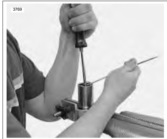
Figure 2-93. Compressing Spring Seat to Install Stopper Ring
