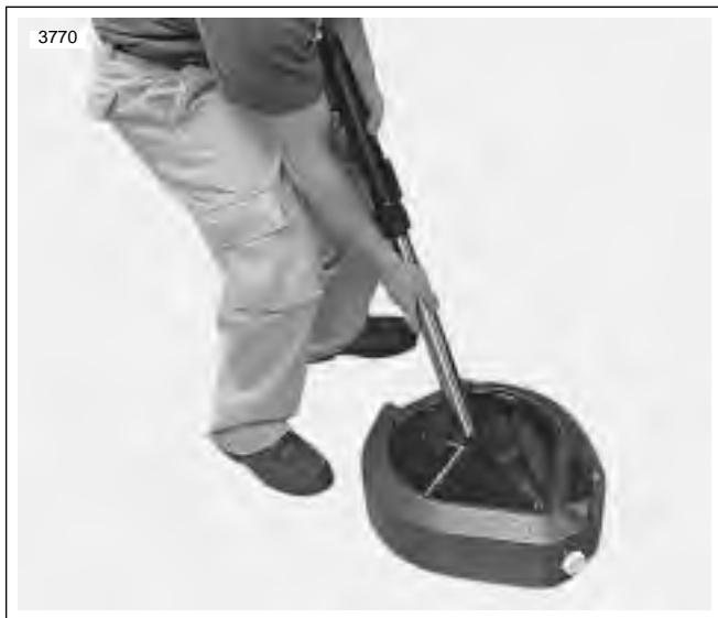
Figure 1-30. Pumping Fork Oil
