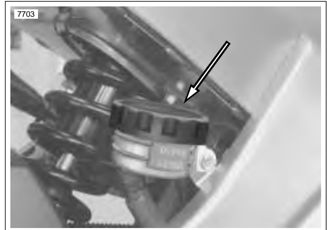
Figure 1-5. Rear Brake Fluid Reservoir
