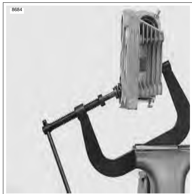
Figure 3-48. Valve Spring Compressor (Part No. HD-34736B)
