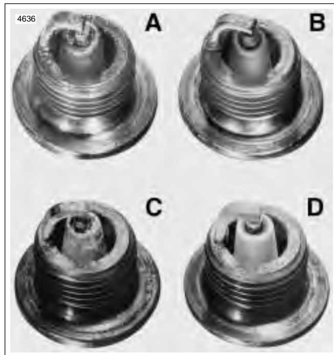
Figure 1-35. Typical Spark Plug Deposits
