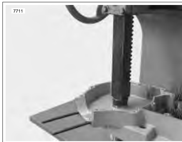
Figure 3-126. Right Outer Bearing Race Installation
