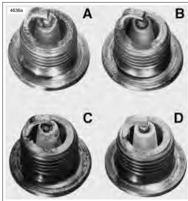
Figure 1-35. Typical Spark Plug Deposits
