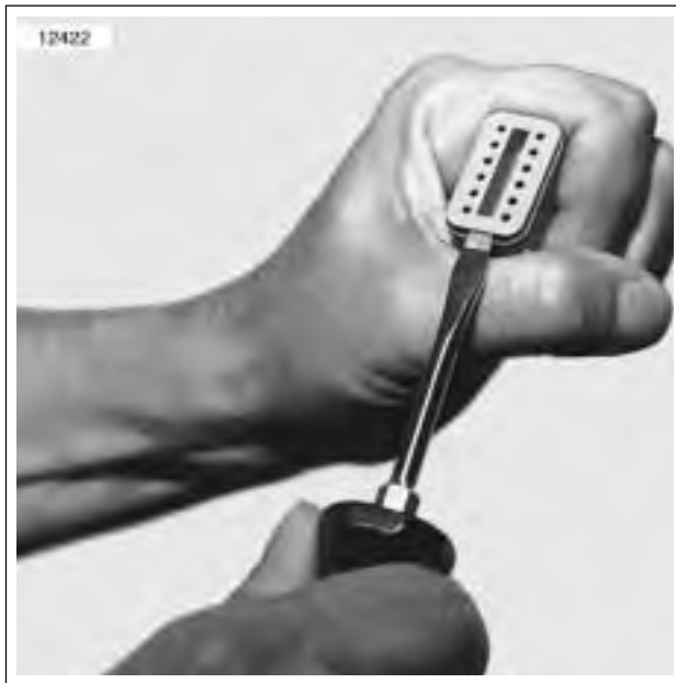
Figure B-9. Remove Secondary Locking Wedge
