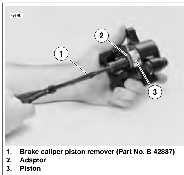
Figure 2-56. Removing Rear Brake Caliper Piston
