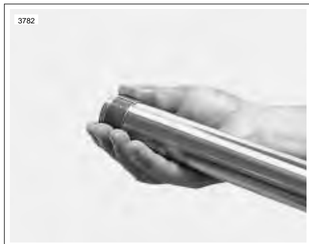
Figure 2-79. Install Slide Bushing
