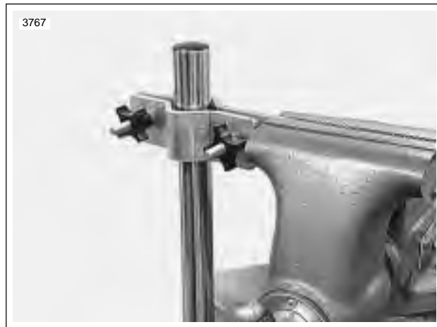
Figure 2-67. Clamping the Fork
