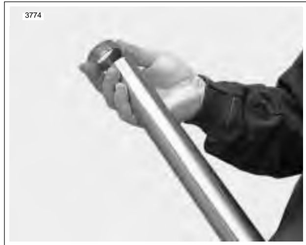
Figure 2-86. Install Guide Bushing
