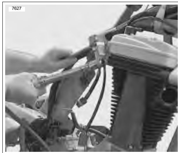
Figure 3-4. Remove Top Rear Tie Bar
