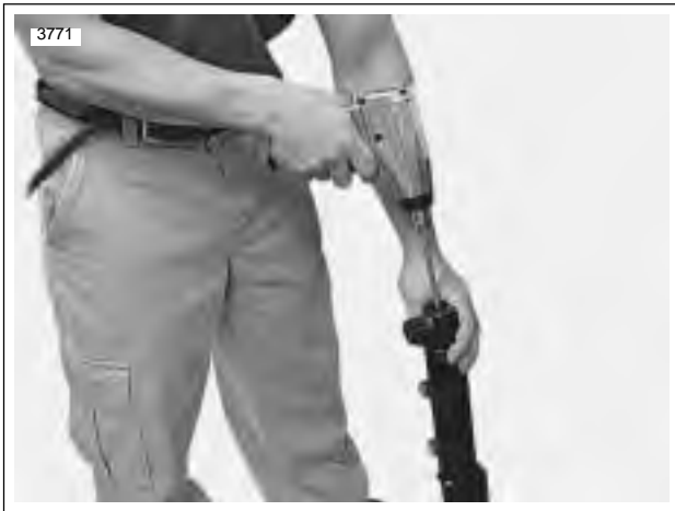
Figure 2-72. Removing Center Bolt
