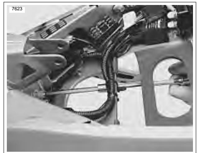
Figure 3-28. Installing Rear Motor Mount Bolts
