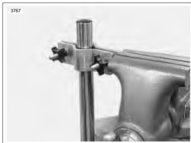
Figure 1-26. Clamping the Fork
