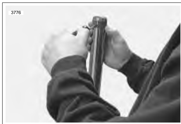
Figure 2-76. Removing Slide Bushing
