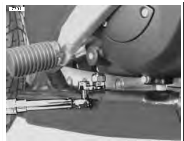
Figure 6-6. Torquing Chain Limiting Screw
