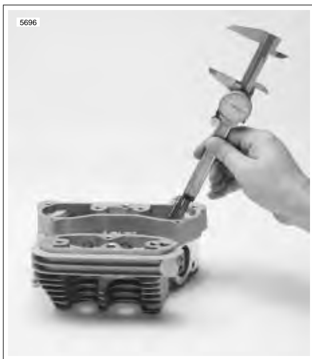
Figure 3-55. Measuring Valve Stem Protrusion
