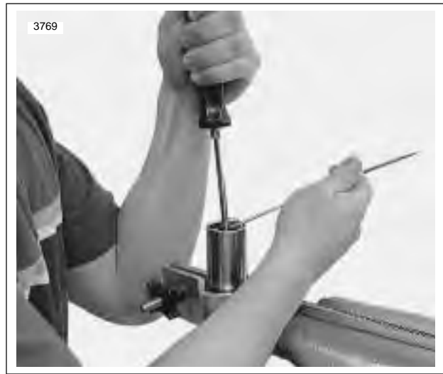
Figure 2-93. Compressing Spring Seat to Install Stopper Ring
