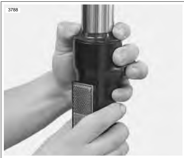
Figure 2-91. Install New Dust Seal
