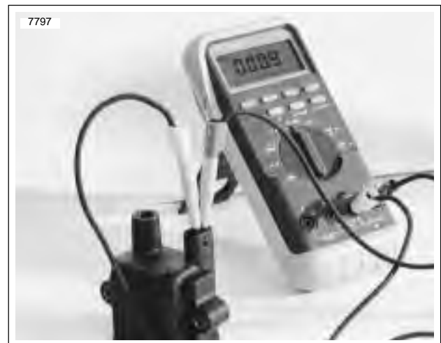
Figure 7-25. Ignition Coil Primary Resistance Test
