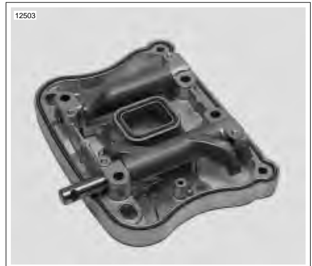
Figure 3-46. Removing Rocker Arm Shafts
