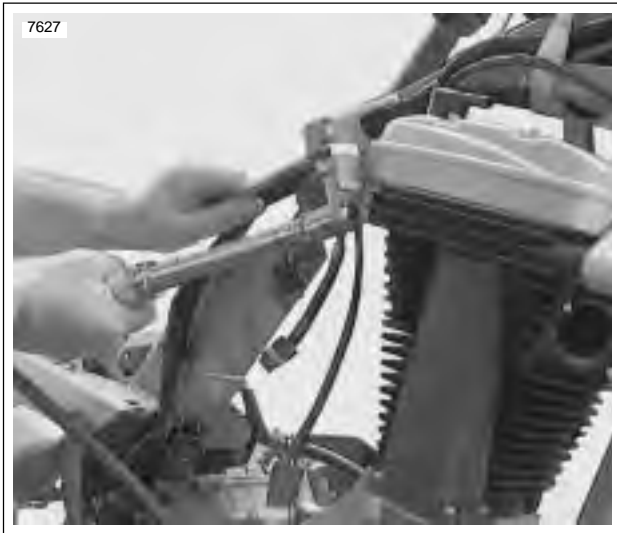
Figure 3-38. Install Top Rear Tie Bar
