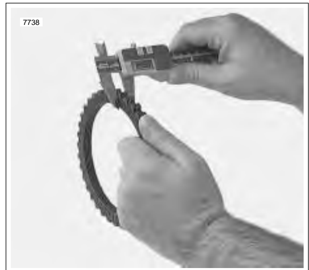
Figure 6-18. Measuring Friction Plates
