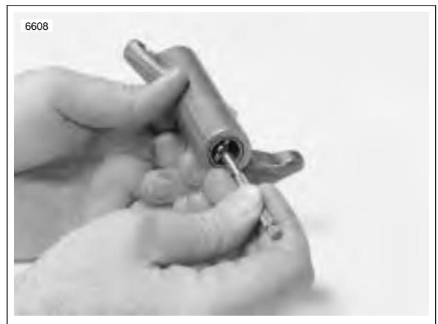
Figure 3-54. Measuring Rocker Arm Bushing Inner Diameter
