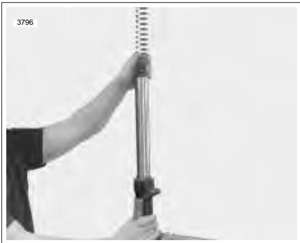
Figure 2-84. Install Rebound Spring
