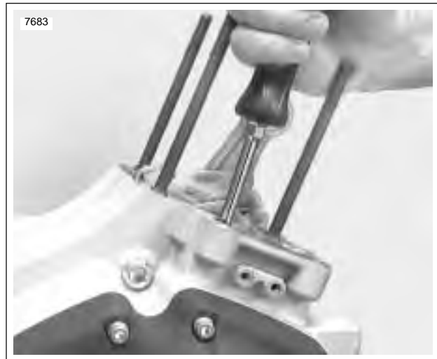
Figure 3-108. Checking Cam Gear End Play
