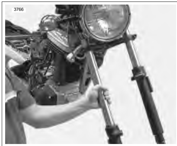
Figure 2-95. Installing Fork Assemblies
