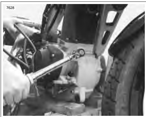
Figure 3-39. Install Front Tie Bar
