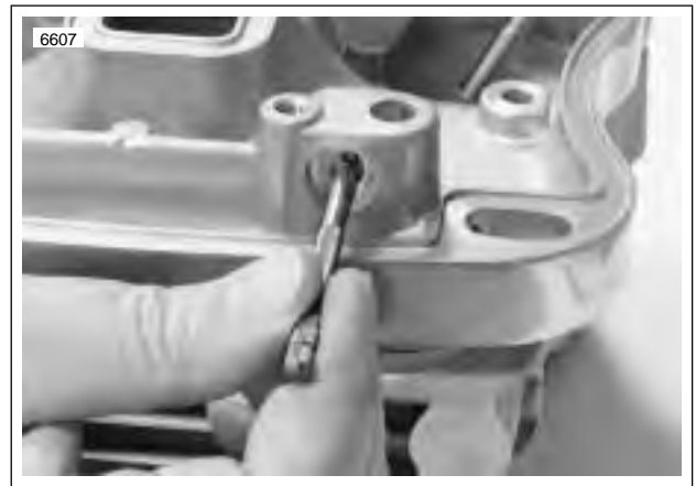
Figure 3-53. Measuring Rocker Arm Shaft Bore Diameter in Lower Rocker Cover
