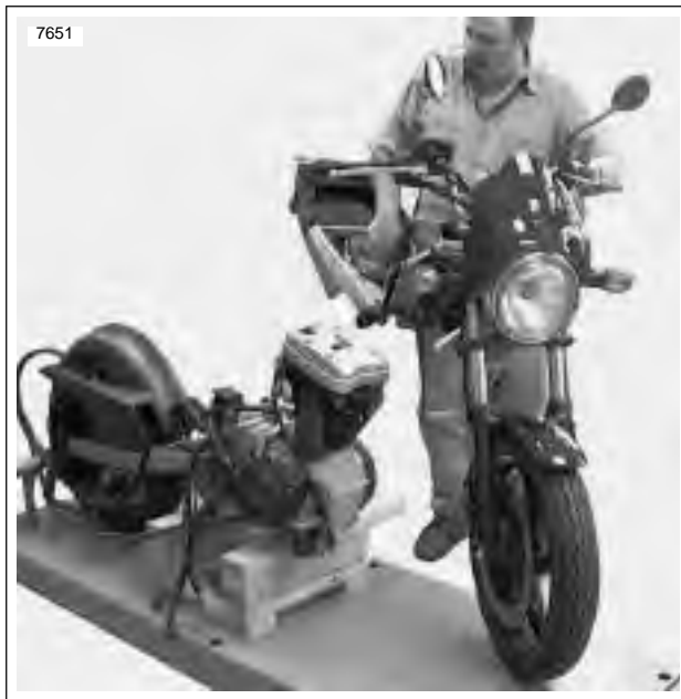
Figure 3-26. Move Chassis to Engine
