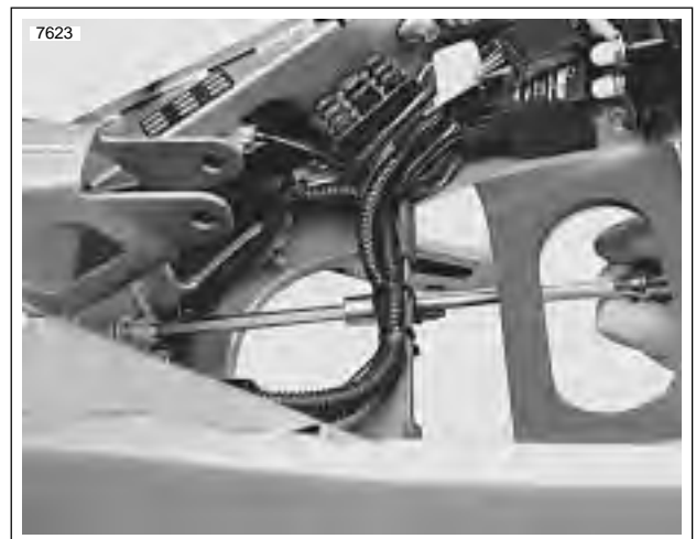
Figure 3-14. Removing Rear Motor Mount Bolts
