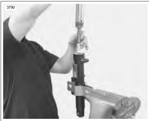
Figure 2-83. Installing Slider Tube
