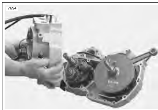
Figure 6-27. Splitting Crankcase Halves
