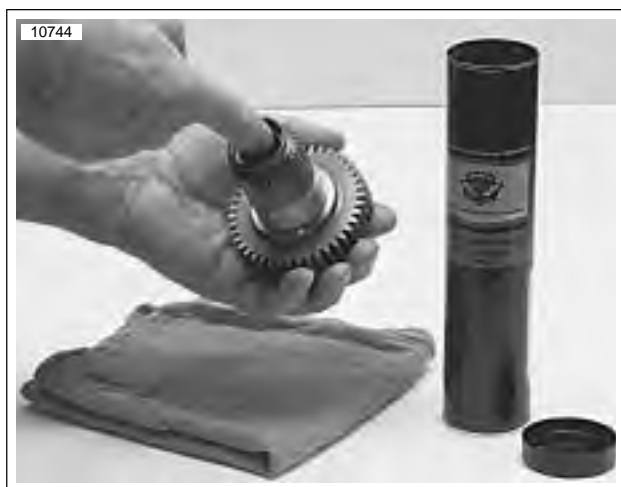
Figure 6-41. Lubricating Main Drive Gear Needle Bearings
