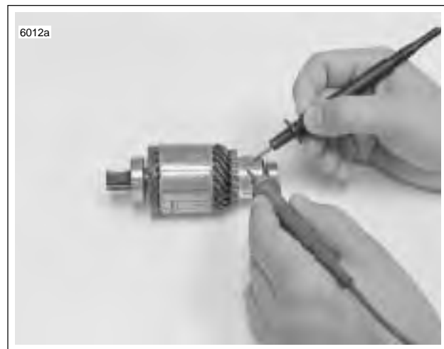
Figure 5-22. Open Armature Test
