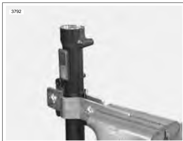
Figure 2-82. Clamping the Slider Assembly
