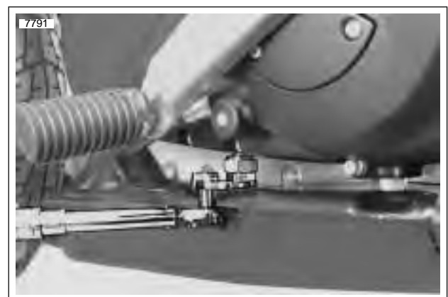
Figure 1-24. Tightening Chain Limiting Screw
