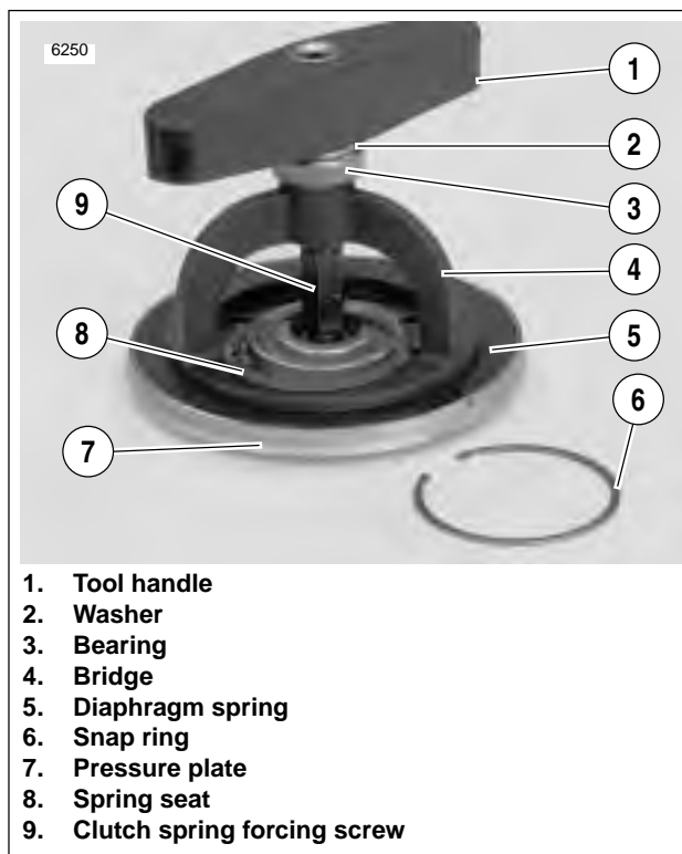
Figure 6-13. Pressure Plate Assembly
