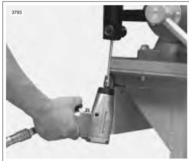
Figure 2-85. Install Center Bolt
