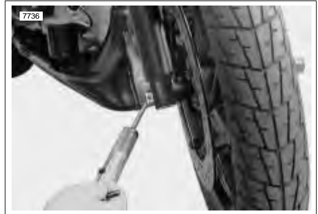
Figure 1-33. Steering Head Bearing Check
