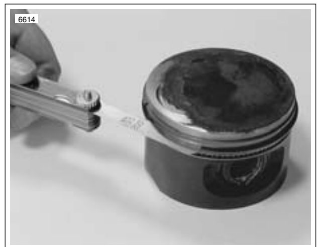
Figure 3-39. Measuring Ring Clearance in Groove
