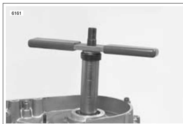
Figure 3-94. Installing Flywheel Spacer and Outer Bearing
