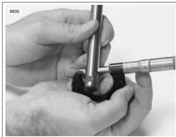
Figure 3-13. Measuring Rocker Arm Shaft Diameter (Rocker Arm Bushing Position)
