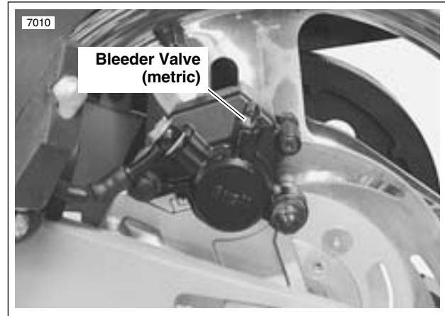
Figure 2-35. Rear Caliper Bleeder Valve (Metric-Typical)
