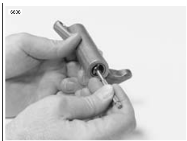
Figure 3-15. Measuring Rocker Arm Bushing Inner Diameter
