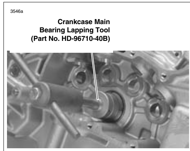
Figure 3-90. Lapping Pinion Shaft Main Bearing
