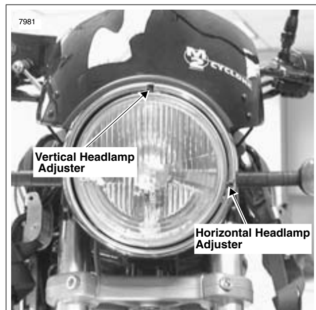
Figure 1-58. Headlamp Height Adjustment
