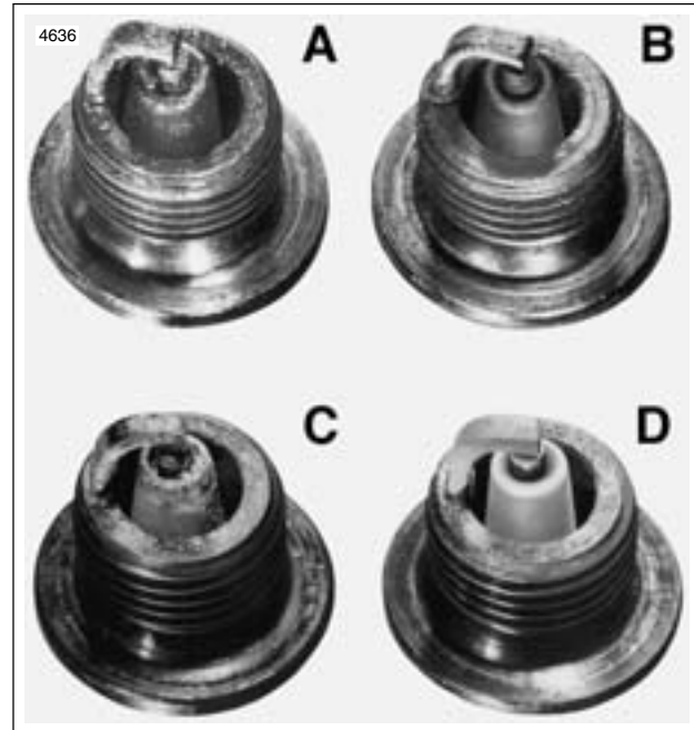
Figure 1-39. Typical Spark Plug Deposits
