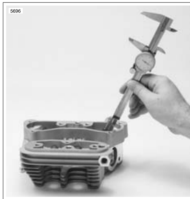
Figure 3-23. Measuring Valve Stem Protrusion
