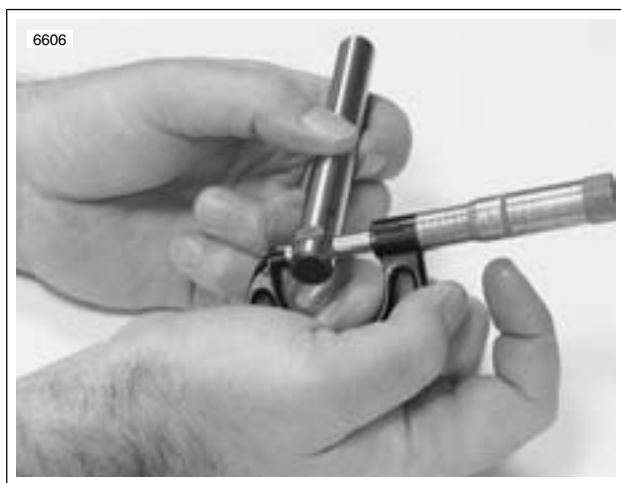
Figure 3-12. Measuring Rocker Arm Shaft Diameter (Rocker Cover Position)
