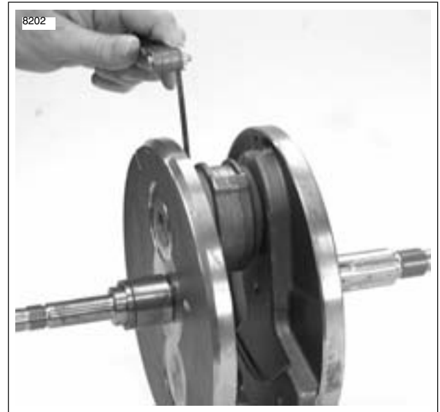
Figure 3-83. Checking Connecting Rod Side Play
