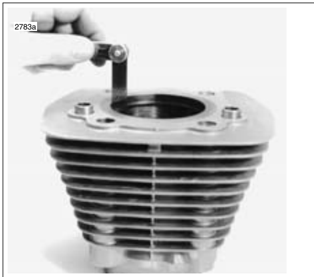
Figure 3-36. Measuring Ring End Gap
