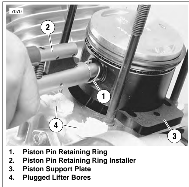
Figure 3-40. Installing Piston Retaining Rings
