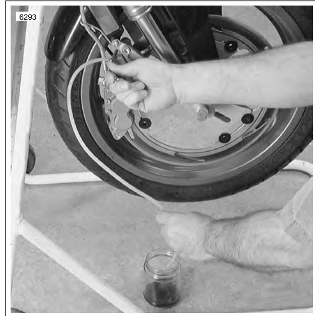
Figure 2-20. Draining Front Brake System (Typical)
