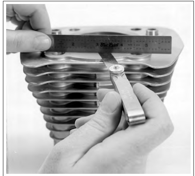
Figure 3-31. Checking Gasket Surfaces
