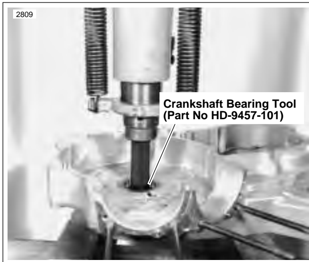
Figure 3-77. Sprocket Shaft Outer Race Removal
