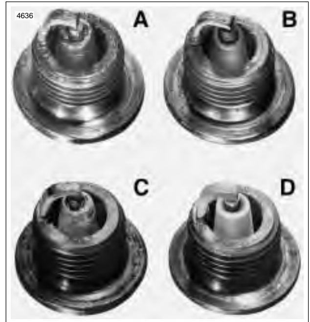
Figure 1-40. Typical Spark Plug Deposits
