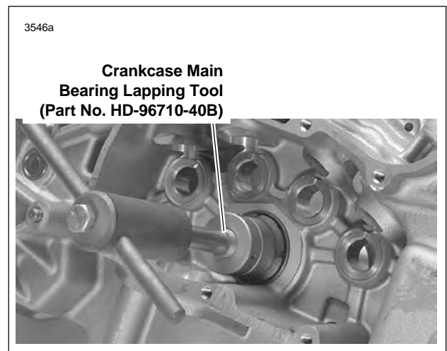
Figure 3-132. Lapping Pinion Shaft Main Bearing
