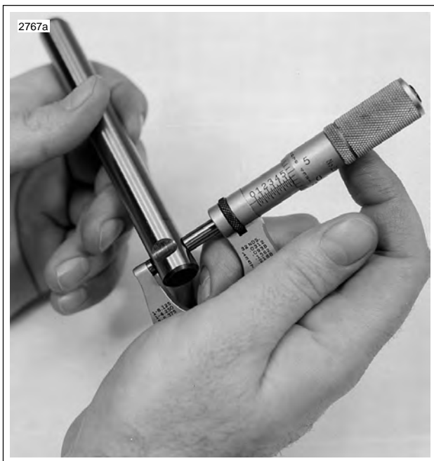
Figure 3-12. Measuring Rocker Arm Shaft Diameter (Rocker Cover Position)
