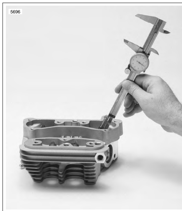
Figure 3-23. Measuring Valve Stem Protrusion
