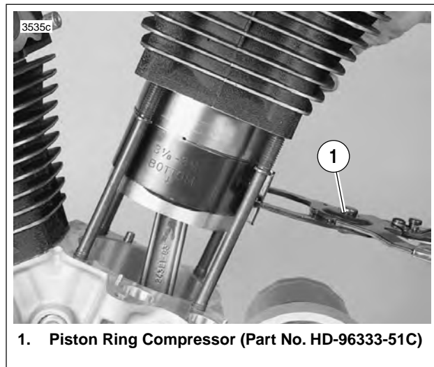
Figure 3-42. Compressing Piston Rings
