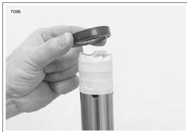
Figure 2-54. Slide Pipe Protection
