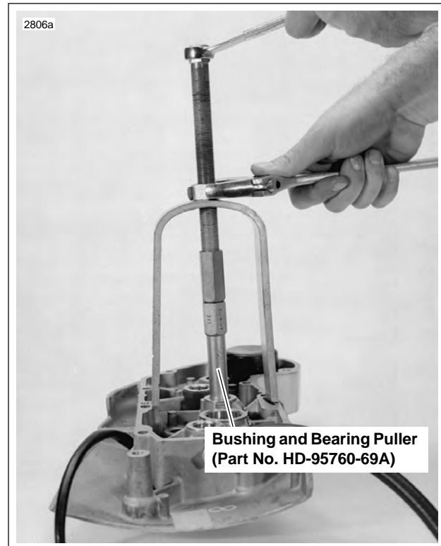
Figure 3-61. Removing Bushing
