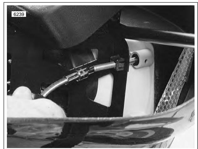
Figure 1-55. Headlamp Lateral Adjustment
