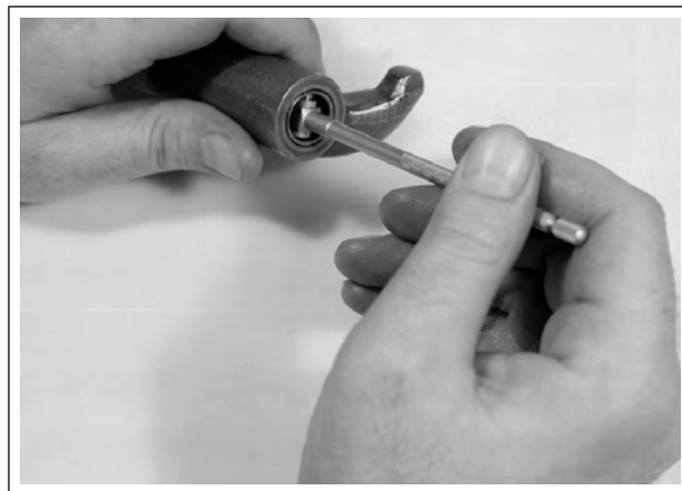
Figure 3-15. Measuring Rocker Arm Bushing Inner Diameter
