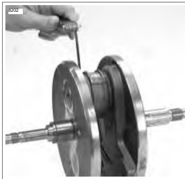
Figure 3-80. Checking Connecting Rod Side Play
