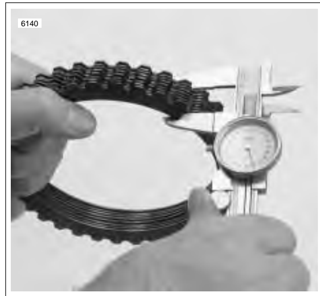
Figure 6-19. Measuring Friction Plates
