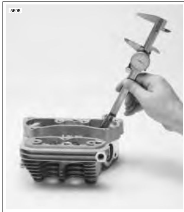
Figure 3-23. Measuring Valve Stem Protrusion
