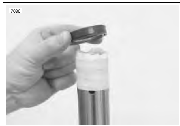
Figure 2-51. Slide Pipe Protection
