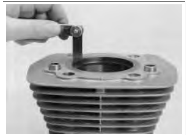
Figure 3-34. Measuring Ring End Gap
