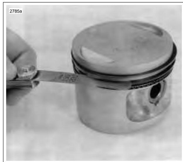
Figure 3-37. Measuring Ring Clearance in Groove
