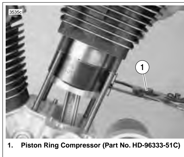
Figure 3-42. Compressing Piston Rings
