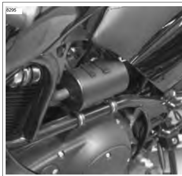
Figure 4-110. Carbon Canister Installed
