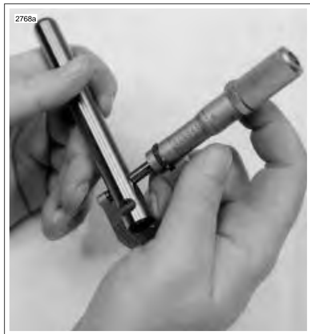
Figure 3-13. Measuring Rocker Arm Shaft Diameter (Rocker Arm Bushing Position)
