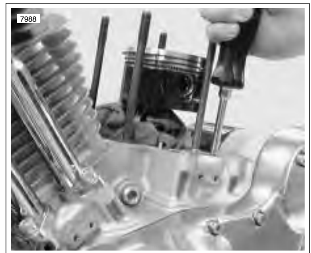
Figure 3-71. Checking Cam Gear End Play
