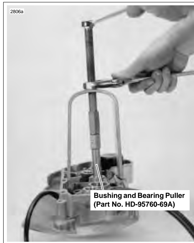
Figure 3-61. Removing Bushing
