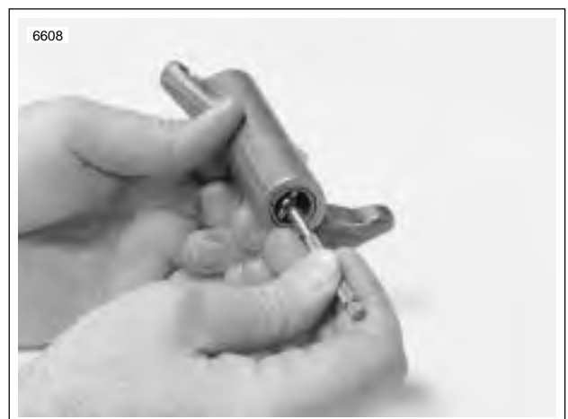
Figure 3-15. Measuring Rocker Arm Bushing Inner Diameter
