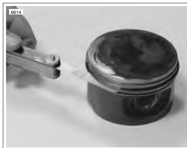
Figure 3-39. Measuring Ring Clearance in Groove
