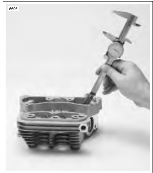
Figure 3-23. Measuring Valve Stem Protrusion
