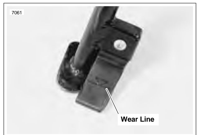
Figure 2-139. Side Stand Dragger Wear Limit
