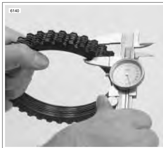
Figure 6-19. Measuring Friction Plates
