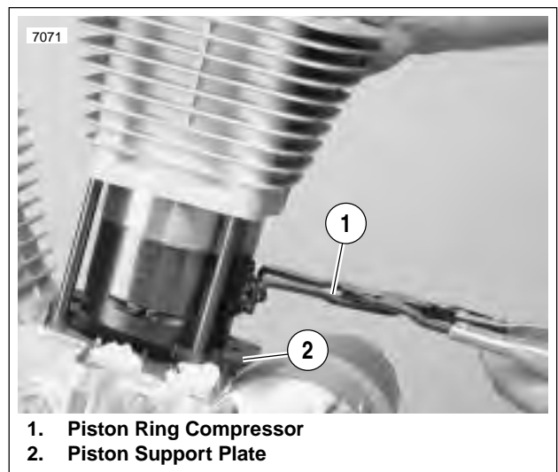
Figure 3-44. Compressing Piston Rings
