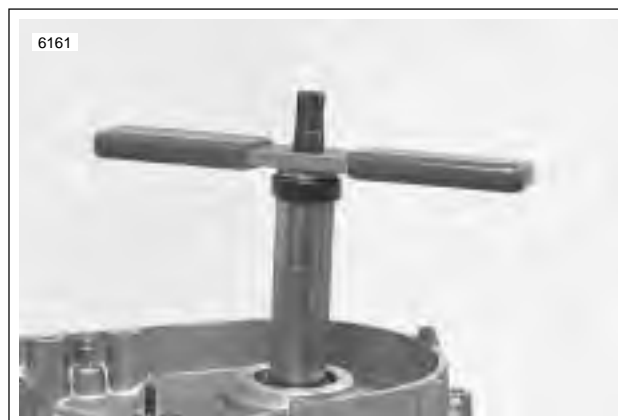
Figure 3-94. Installing Flywheel Spacer and Outer Bearing
