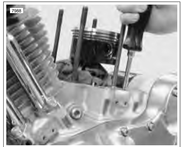
Figure 3-74. Checking Cam Gear End Play
