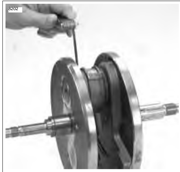
Figure 3-83. Checking Connecting Rod Side Play
