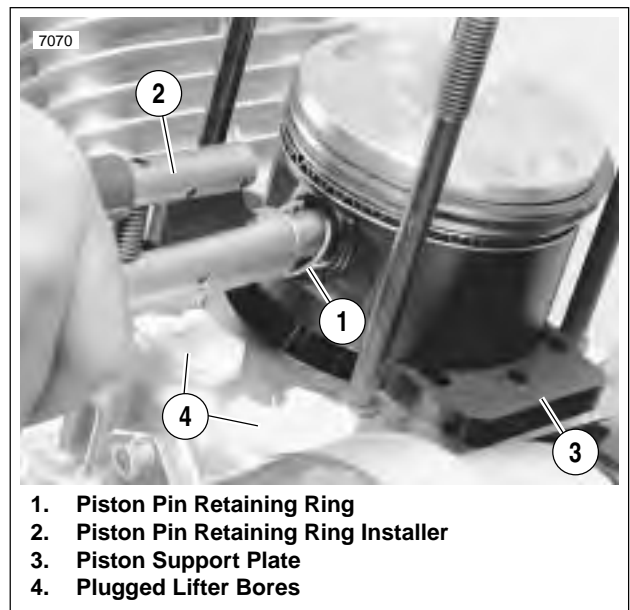
Figure 3-42. Installing Piston Retaining Rings
