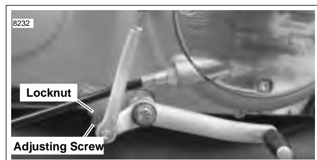
Figure 1-28. Measuring Primary Chain Adjustment
