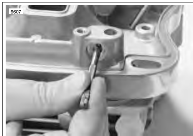
Figure 3-71. Measuring Rocker Arm Shaft Bore Diameter in Lower Rocker Cover
