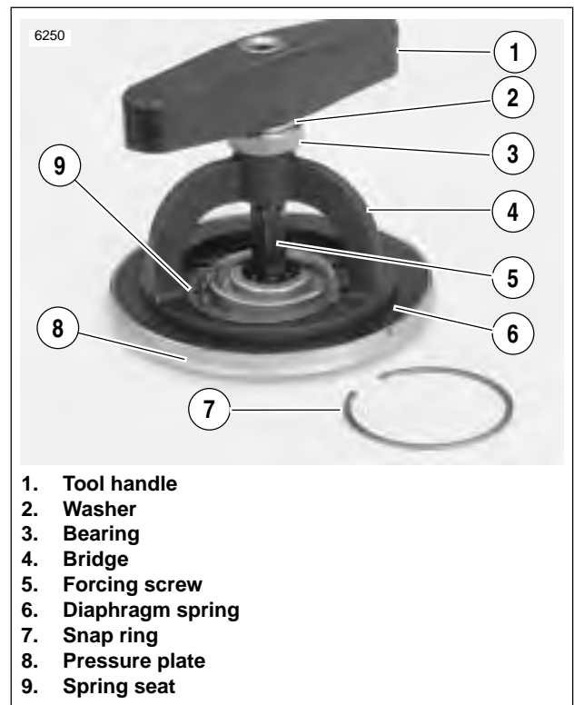
Figure 6-14. Pressure Plate Assembly
