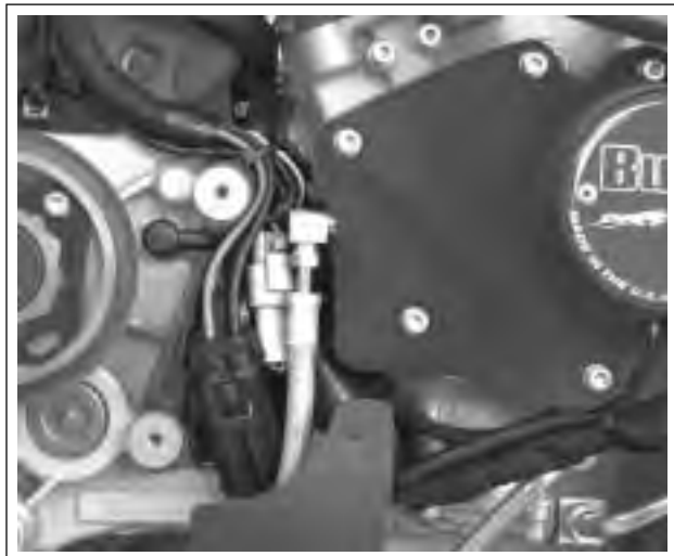
Figure 3-56. Correct Routing of Wiring Harnesses
