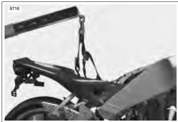
Figure 3-25. Supporting Vehicle for Disassembly
