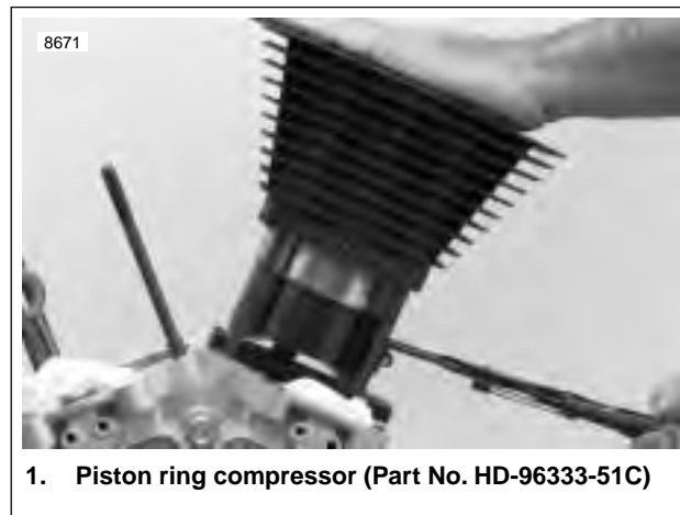
Figure 3-111. Compressing Piston Rings
