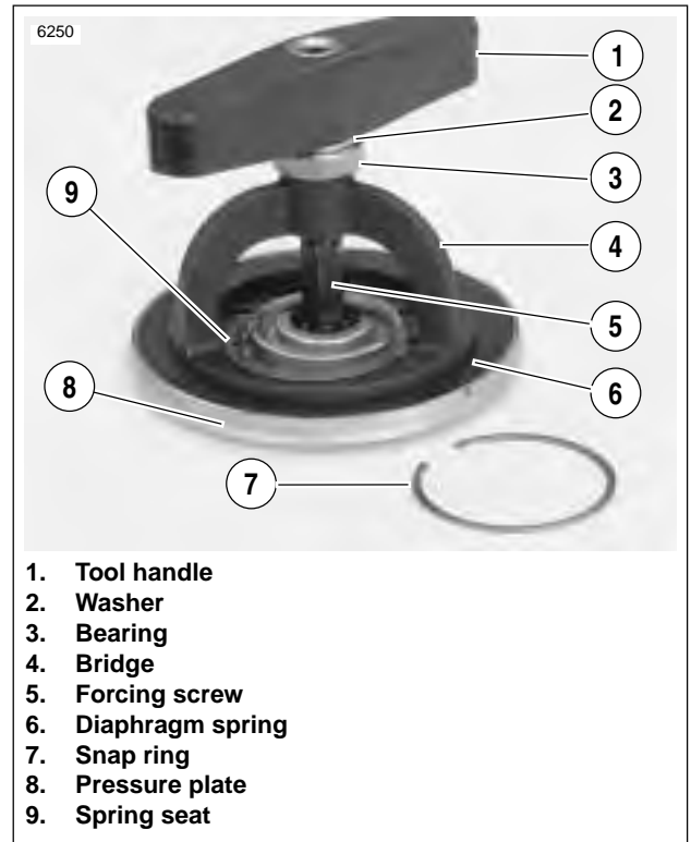
Figure 6-34. Pressure Plate Assembly
