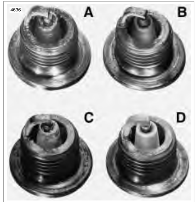
Figure 1-44. Typical Spark Plug Deposits
