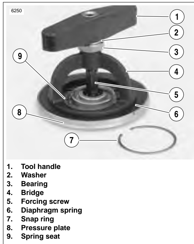
Figure 6-19. Pressure Plate Assembly
