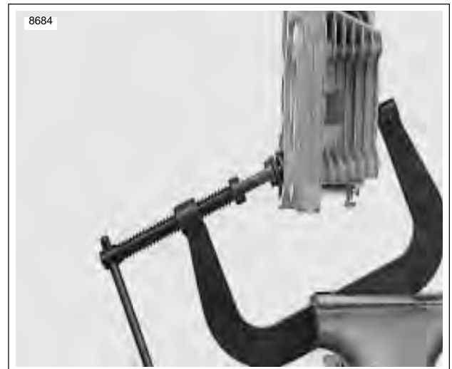
Figure 3-64. Valve Spring Compressor (Part No. HD-34736B)
