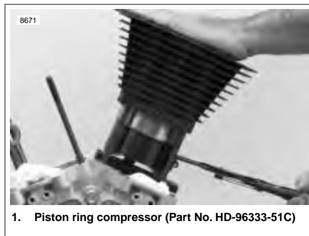
Figure 3-109. Compressing Piston Rings
