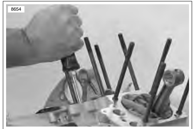
Figure 3-132. Checking Cam Gear End Play
