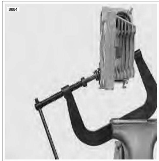
Figure 3-82. Valve Spring Compressor (Part No. HD-34736B)
