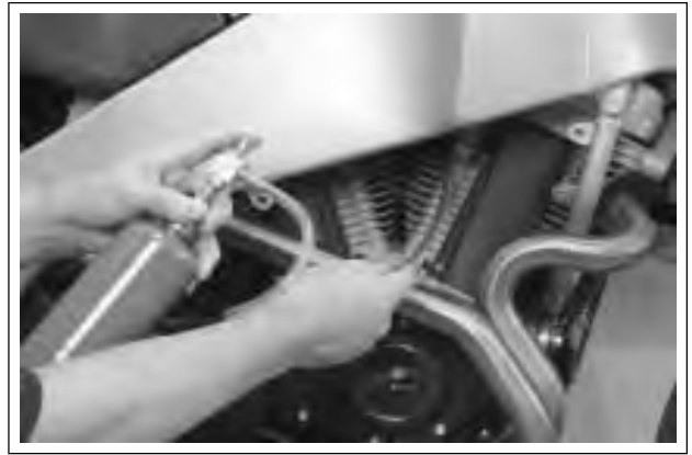
Figure 4-118. Checking for Intake Leak
