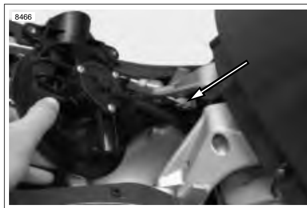
Figure 4-84. Cooling Fan Connector [97]
