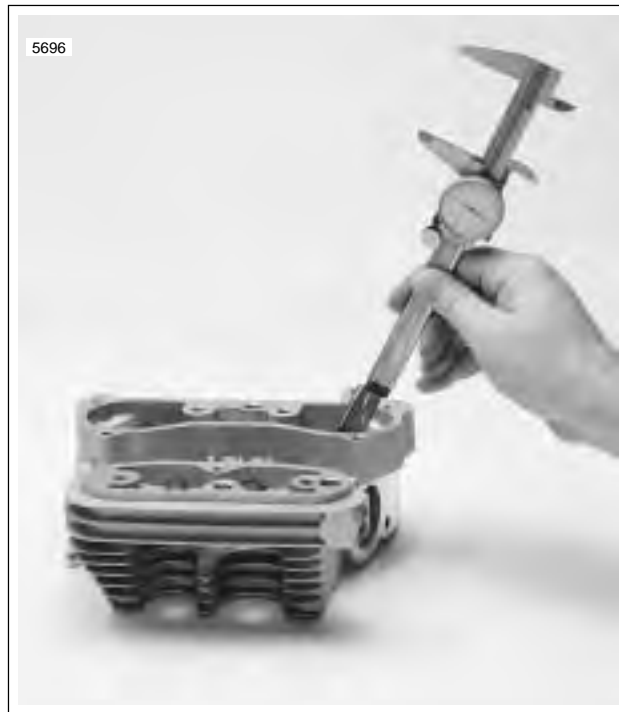
Figure 3-71. Measuring Valve Stem Protrusion
