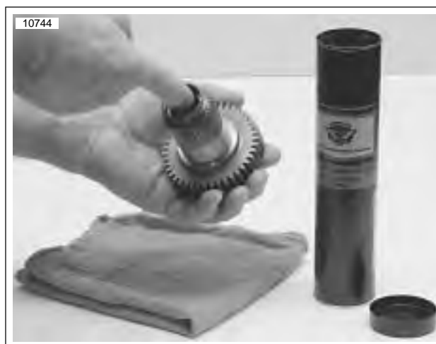
Figure 6-74. Lubricating Main Drive Gear Needle Bearings
