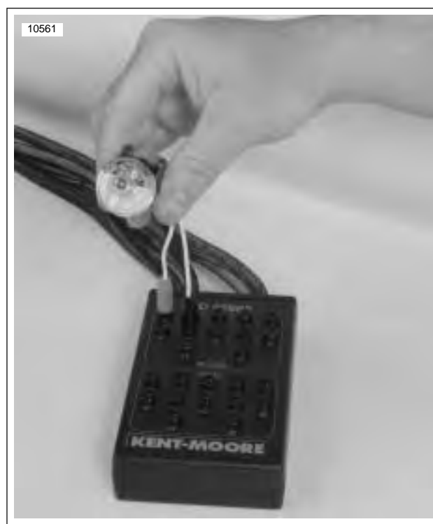
Figure 4-49. Testing Ignition Coil Connectors
