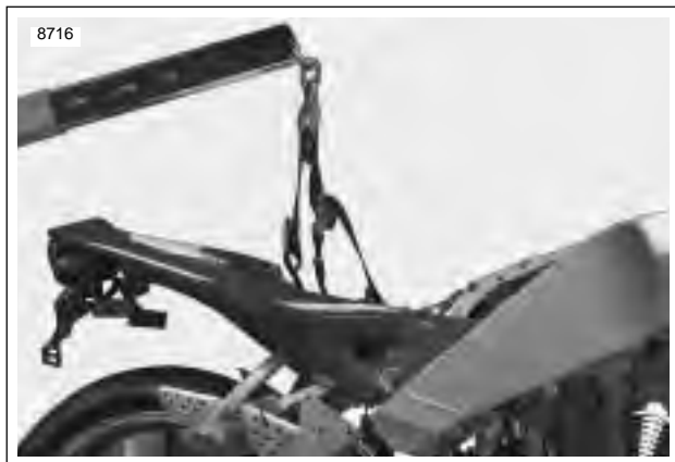
Figure 3-24. Supporting Vehicle for Disassembly
