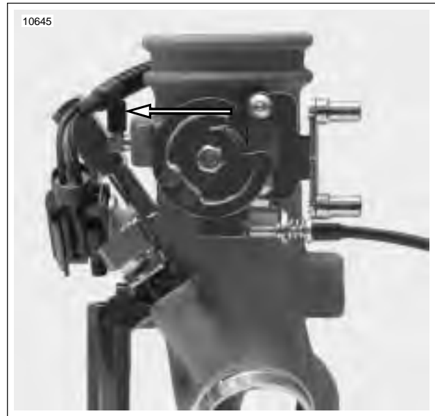
Figure 4-128. Emissions Hose Attachment, California Models Only
