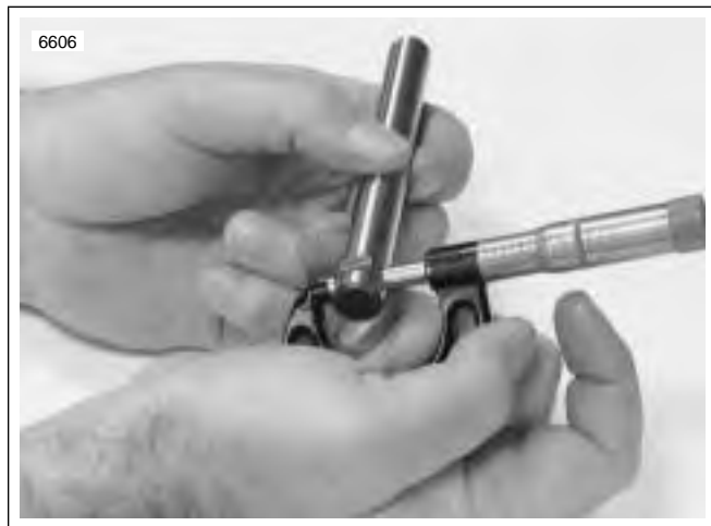
Figure 3-64. Measuring Rocker Arm Shaft Diameter (Rocker Cover Position)
