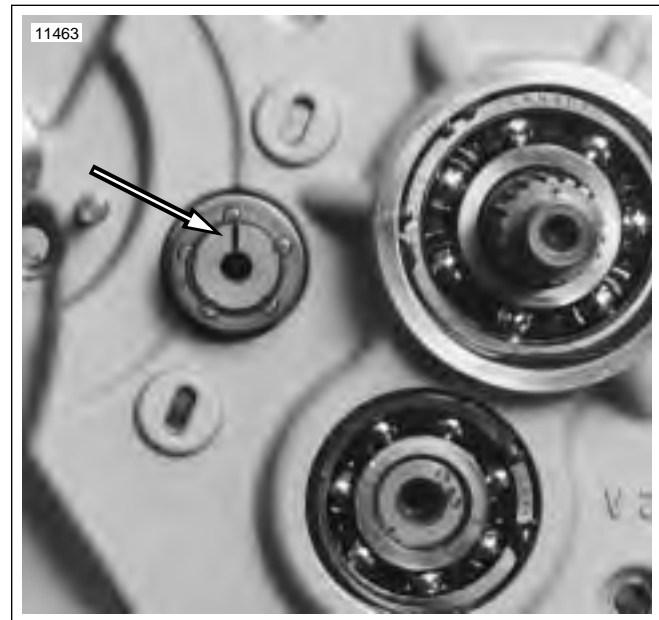
Figure 6-48. Shifter Drum and Mainshaft (Transmission in Neutral)
