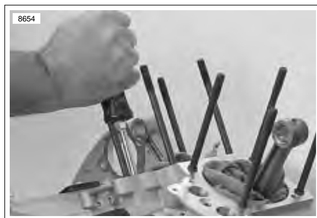
Figure 3-132. Checking Cam Gear End Play
