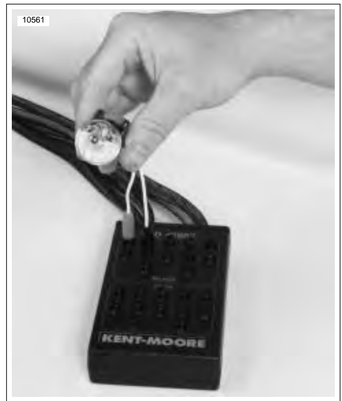
Figure 4-50. Testing Ignition Coil Connectors
