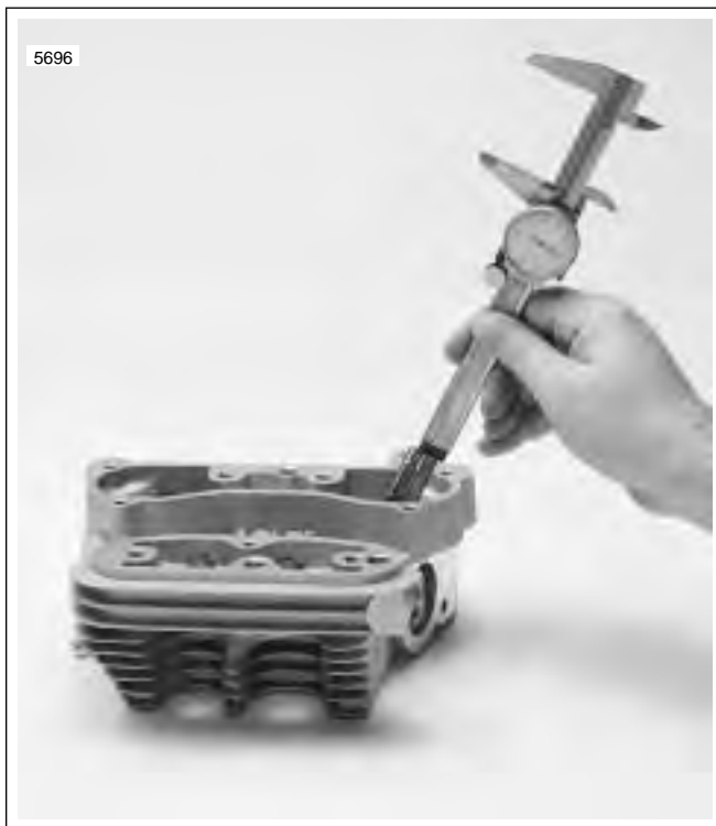
Figure 3-68. Measuring Valve Stem Protrusion
