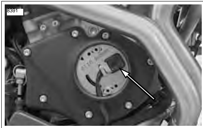
Figure 1-52. Cam Position Sensor (Timing Plate)
