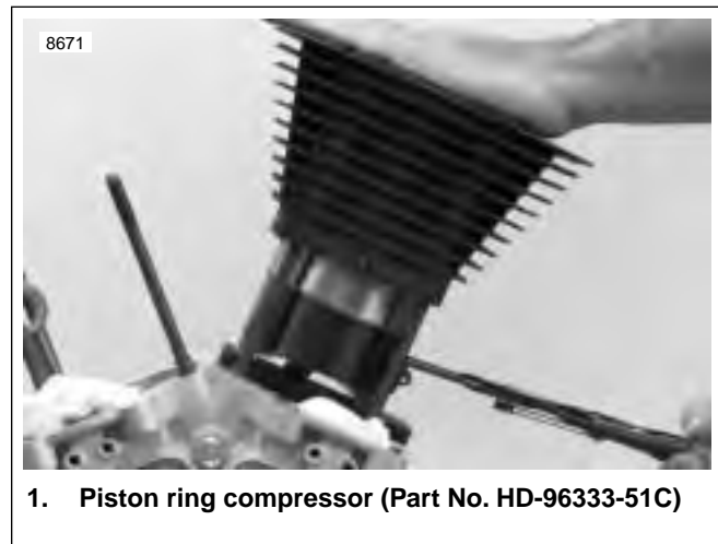
Figure 3-106. Compressing Piston Rings
