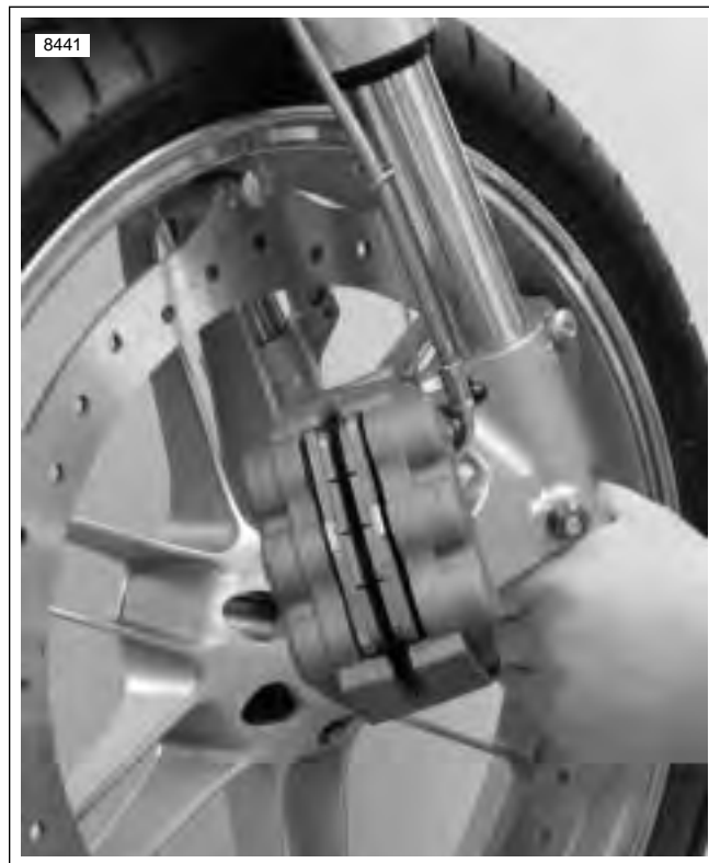
Figure 2-19. Front Wheel Installation
