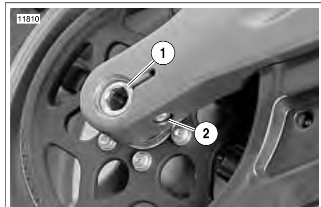
Figure 6-41. Rear Wheel Mounting, Right Side
