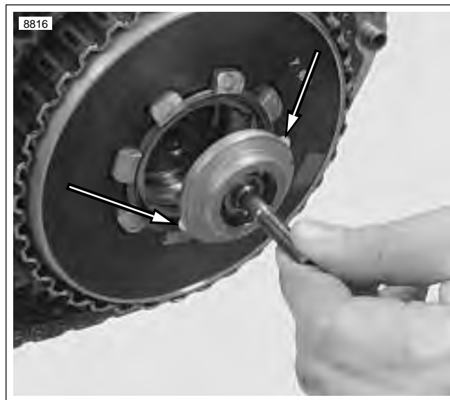
Figure 6-36. Adjusting Screw Assembly Aligning Tabs
