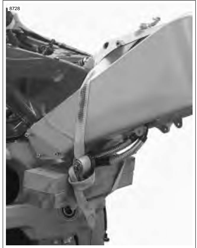
Figure 3-32. Securing Vehicle for Relocation (Typical)
