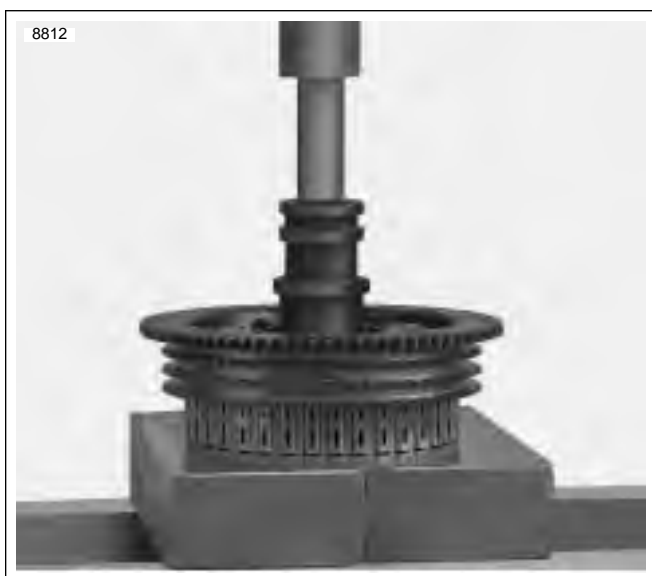
Figure 6-30. Removing Clutch Shell Needle Bearing
