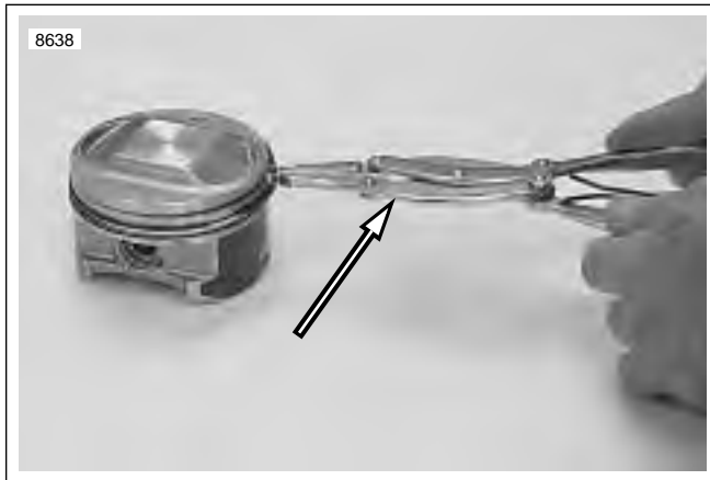
Figure 3-94. Installing Piston Rings Transmission Shaft Retaining Ring Pliers (Part No. J-5586)
