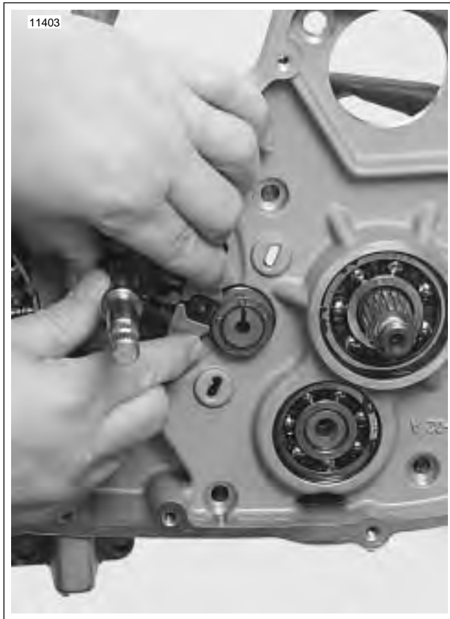
Figure 6-97. Installing Shifter Shaft Assembly
