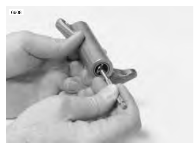
Figure 3-67. Measuring Rocker Arm Bushing Inner Diameter
