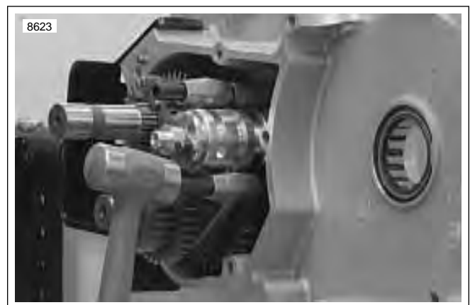
Figure 6-89. Installing Shift Fork Shafts
