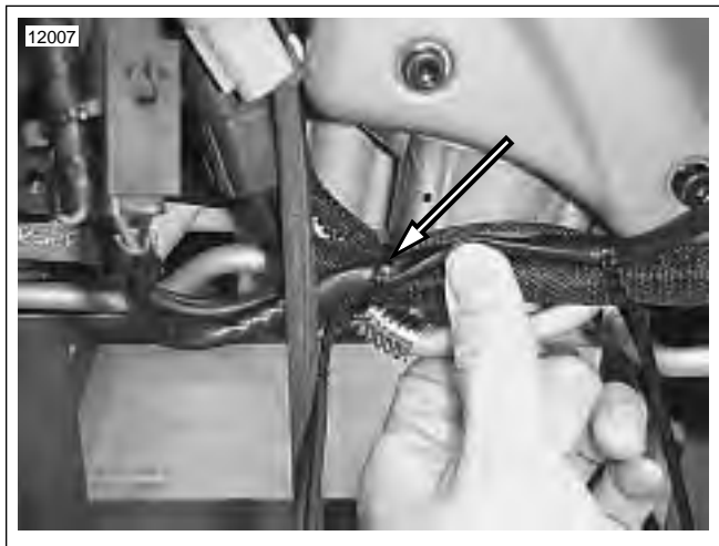
Figure 7-92. Cable Strap Wire Bundle to Return Oil Line
