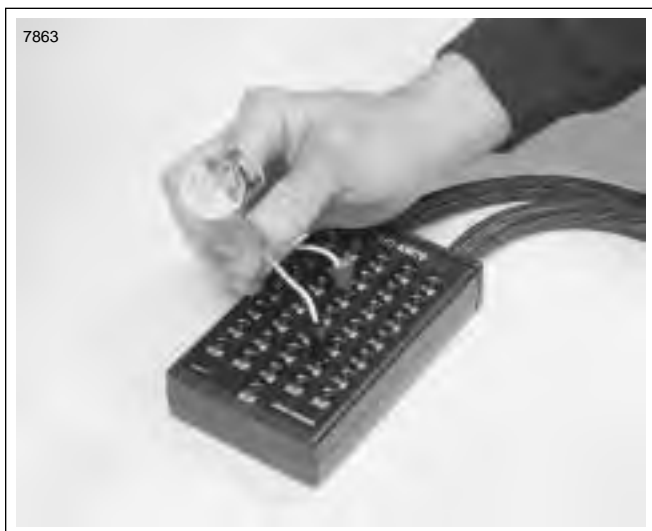
Figure 4-20. Ignition Coil Circuit Test
