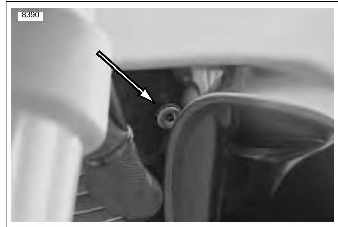
Figure 1-58. Idle Adjuster (behind left fork)
