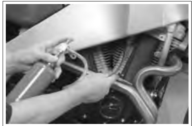
Figure 4-110. Checking for Intake Leak
