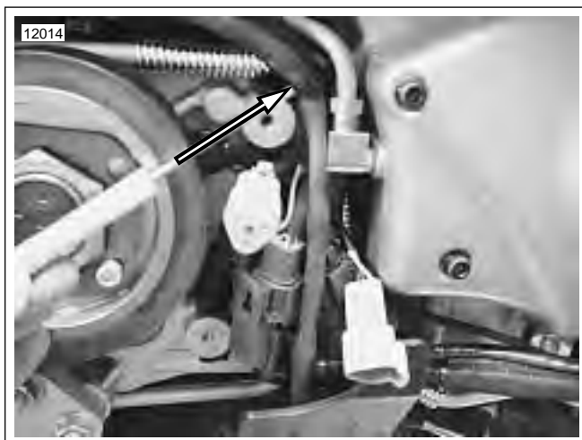
Figure 7-93. Cable Strap Wire Bundle to Return Oil Line, Upper Part of Sprocket Cover
