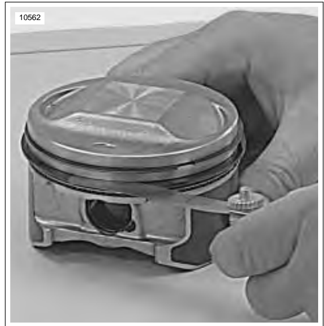
Figure 3-96. Measuring Ring Clearance in Groove
