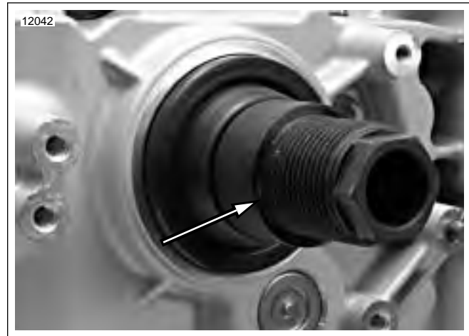
Figure 6-79. Install Adapter (Part No. HD-47856-4) (Typical)
