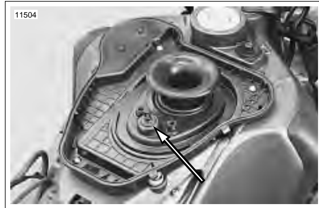
Figure 4-80. Intake Air Temperature Sensor Installed
