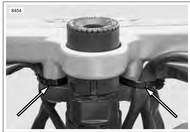
Figure 7-3. Cable Straps On Upper Fork Clamp
