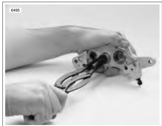
Figure 2-47. Removing Pistons (B-42887)
