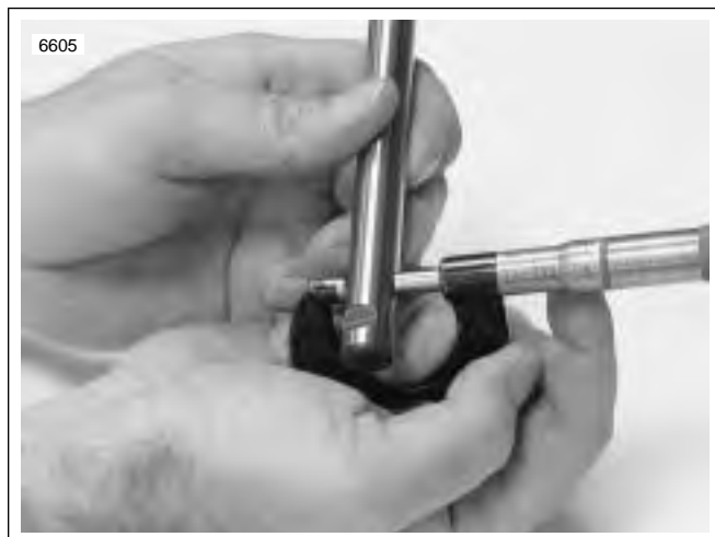
Figure 3-65. Measuring Rocker Arm Shaft Diameter (Rocker Arm Bushing Position)
