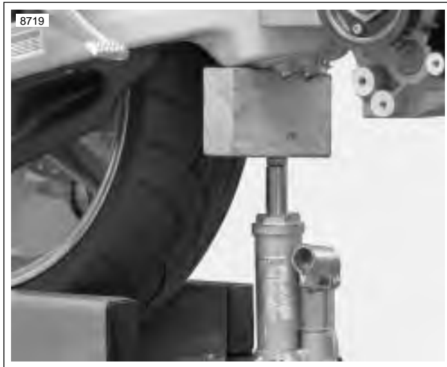
Figure 3-38. Supporting the Swingarm (Typical)
