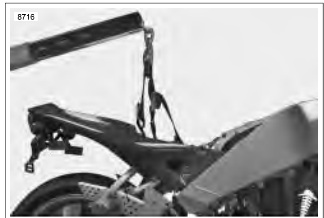
Figure 3-41. Supporting Vehicle for Assembly (Typical)
