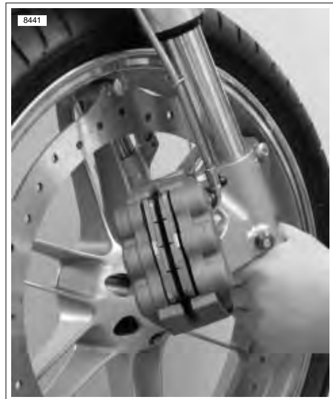
Figure 2-6. Front Wheel Removal
