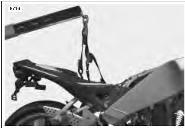
Figure 3-23. Supporting Vehicle for Disassembly (Typical)
