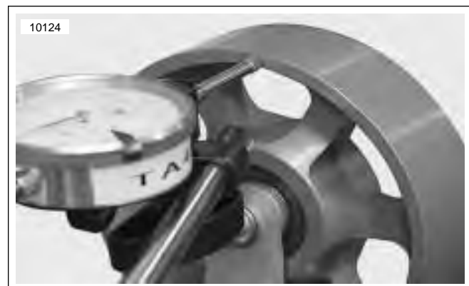
Figure 1-26. Checking Lateral Sideplay on Idler Pulley with a Dial Indicator
