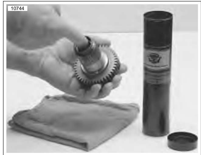
Figure 6-75. Lubricating Main Drive Gear Needle Bearings
