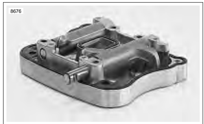
Figure 3-59. Removing Rocker Arm Shafts
