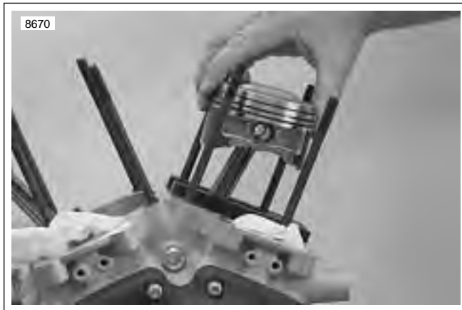
Figure 3-101. Piston Support Plate (Part No. HD-42322)
