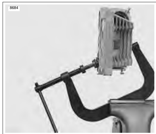
Figure 3-61. Valve Spring Compressor (Part No. HD-34736B)
