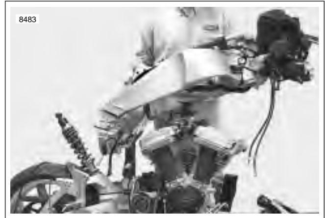
Figure 2-88. Lift Frame Off Motorcycle
