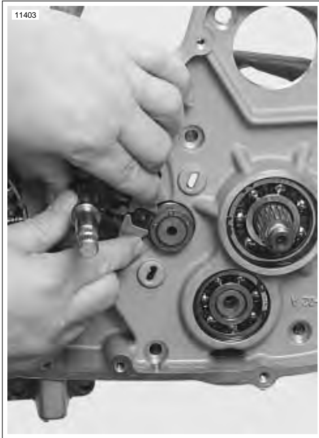
Figure 6-49. Removing Shifter Shaft Assembly
