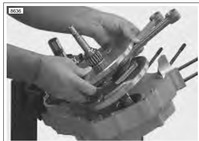
Figure 6-54. Removing Flywheels from Left Case Half
