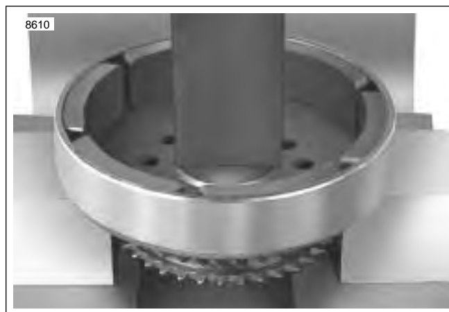
Figure 7-33. Removing Rotor From Sprocket
