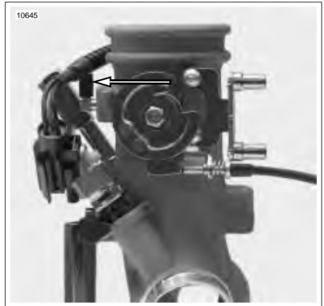
Figure 4-119. Emissions Hose Attachment, California Models Only
