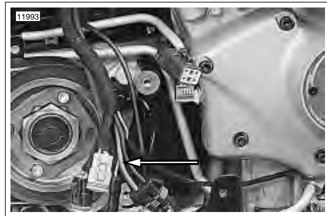
Figure 7-28. Positive Regulator Cable (red wire)
