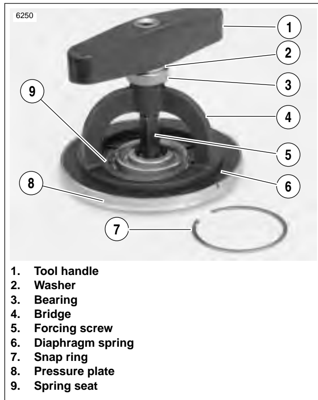
Figure 6-22. Pressure Plate Assembly
