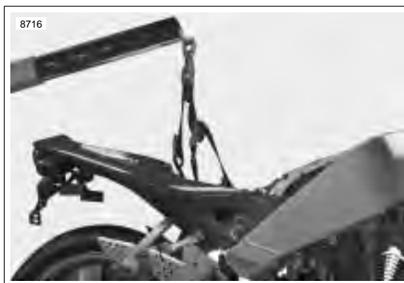
Figure 3-40. Supporting Vehicle for Assembly (Typical)
