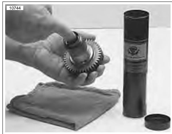
Figure 6-76. Lubricating Main Drive Gear Needle Bearings
