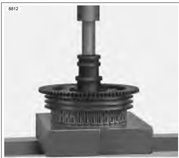
Figure 6-30. Removing Clutch Shell Needle Bearing
