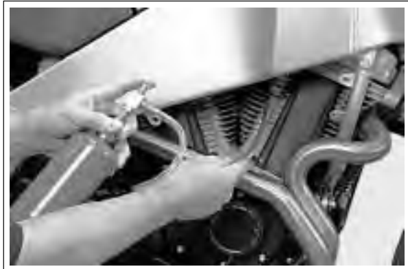
Figure 4-112. Checking for Intake Leak
