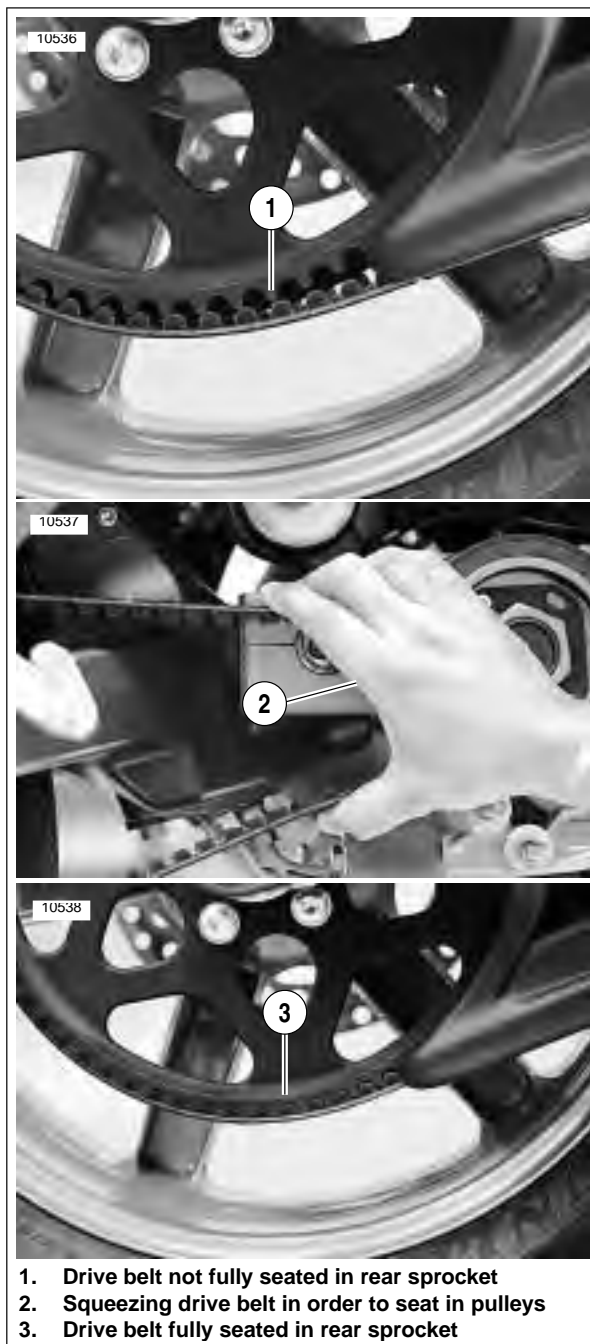
Figure 6-42. Seating Drive Belt Into Pulley Teeth
