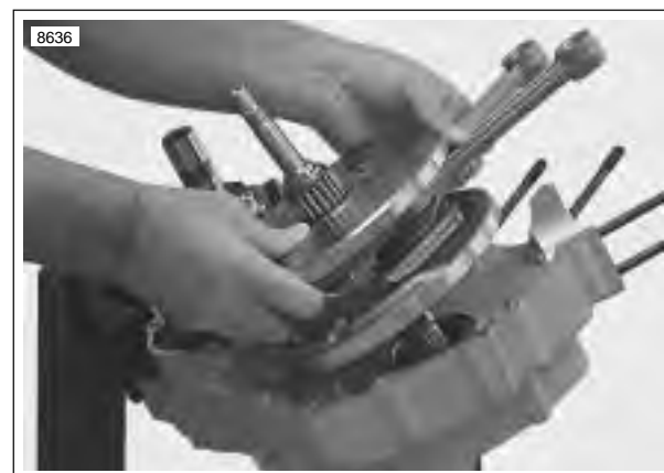
Figure 6-54. Removing Flywheels from Left Case Half
