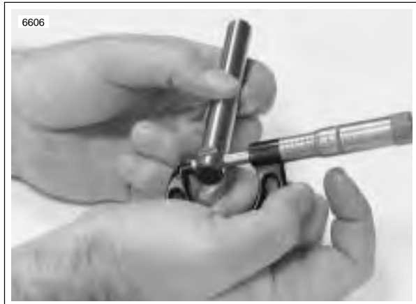
Figure 3-63. Measuring Rocker Arm Shaft Diameter (Rocker Cover Position)
