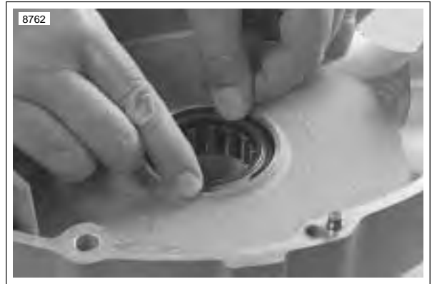
Figure 3-140. Removing Sprocket Shaft Bearing Retaining Ring
