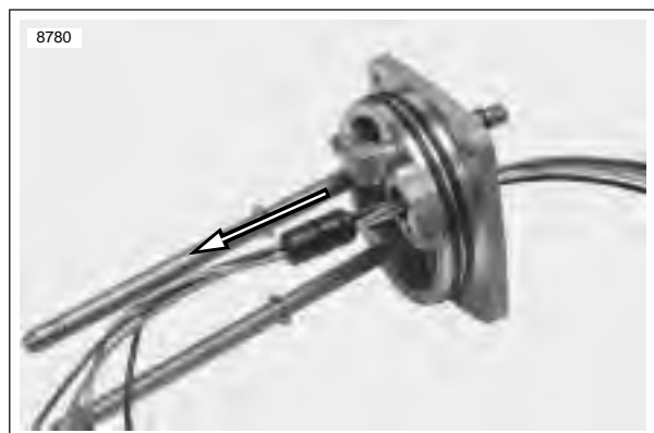
Figure 4-95. Wire Harness Removal Direction
