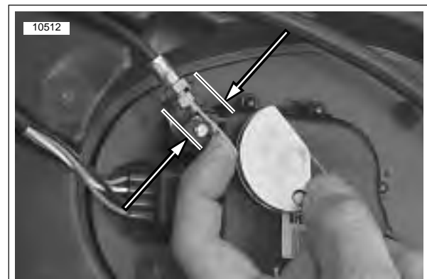
Figure 1-47. Checking For 1/8 in. (3.18) Maximum Free Play In Either Direction For Proper Adjustment
