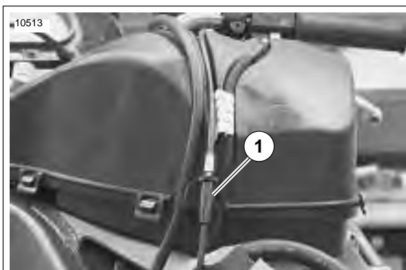
Figure 1-47. Checking For 1/8 in. (3.18) Maximum Free Play In Either Direction For Proper Adjustment
