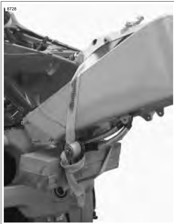
Figure 3-31. Securing Vehicle for Relocation (Typical)
