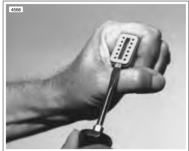
Figure B-6. Remove Secondary Locking Wedge
