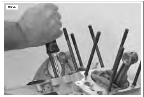
Figure 3-132. Checking Cam Gear End Play
