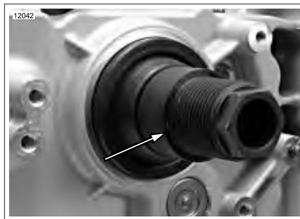
Figure 6-80. Install Adapter (Part No. HD-47856-4) (Typical)
