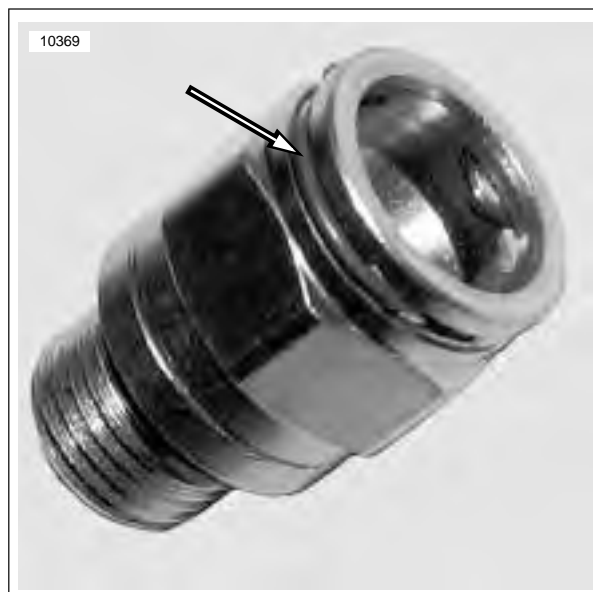
Figure 3-108. Oil Line Fitting with Spring Clip
