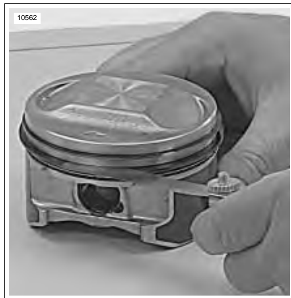
Figure 3-95. Measuring Ring Clearance in Groove
