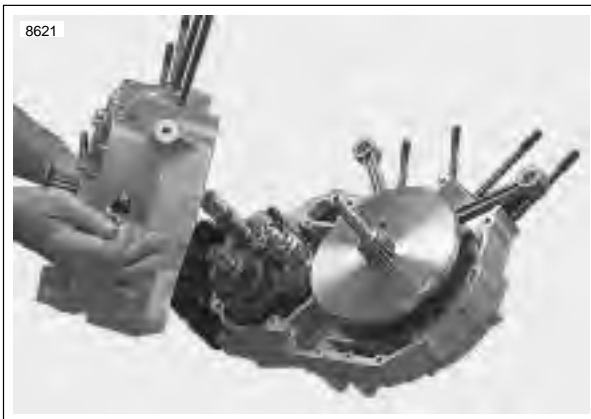
Figure 6-53. Separating Crankcase Halves
