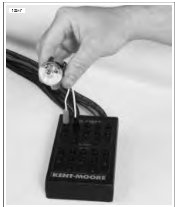
Figure 4-50. Testing Ignition Coil Connectors
