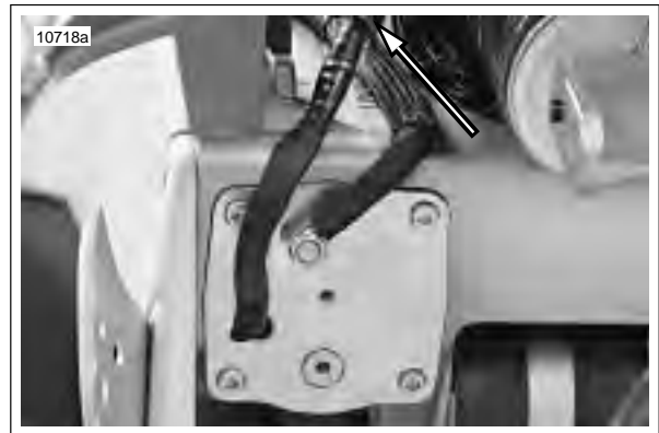
Figure 4-99. Fuel Pump Connector [86] (swingarm removed for illustration)
