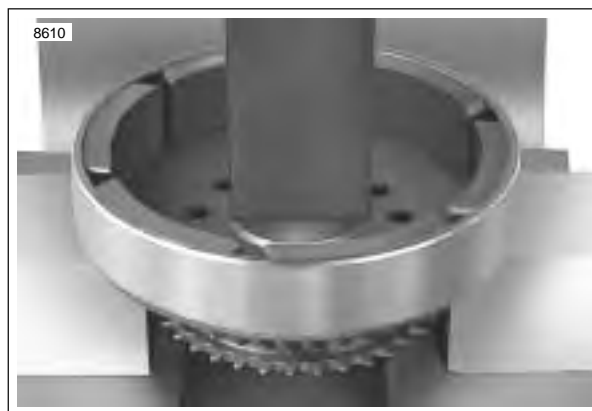
Figure 7-33. Removing Rotor From Sprocket
