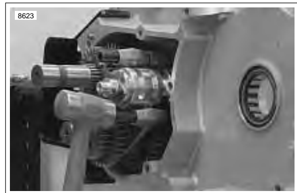
Figure 6-90. Installing Shift Fork Shafts
