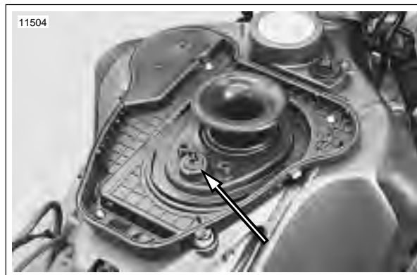
Figure 4-80. Intake Air Temperature Sensor Installed
