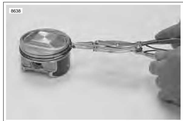
Figure 3-88. Removing Piston Rings
