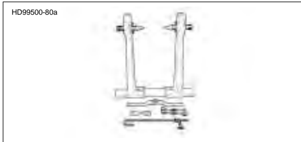
Part No. HD-99500-80 Wheel Truing & Balancing Stand
