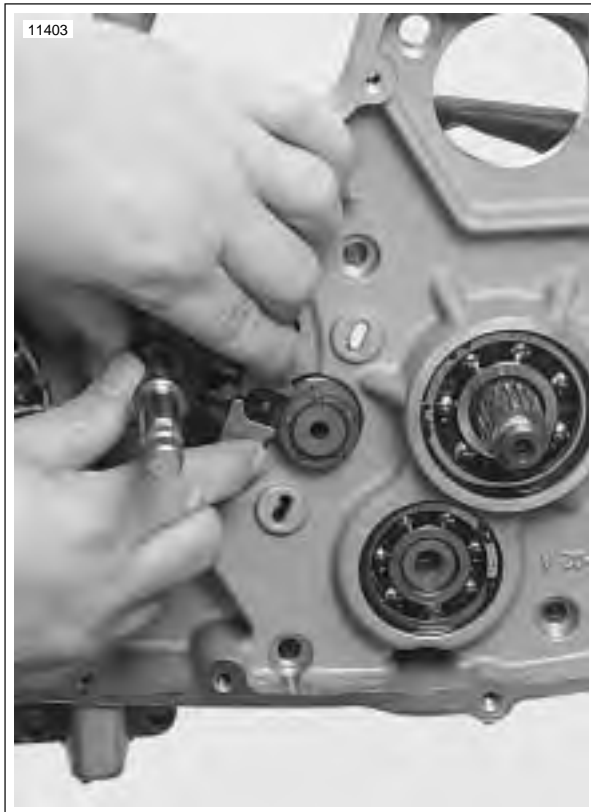
Figure 6-49. Removing Shifter Shaft Assembly
