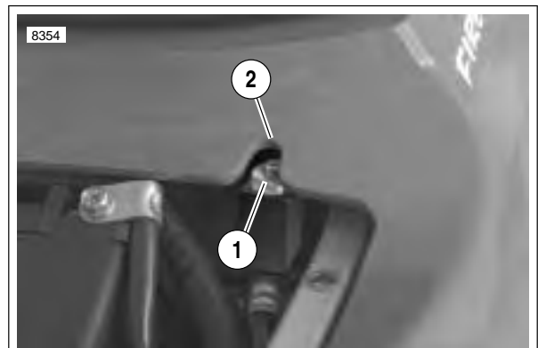
Figure 2-89. Cable Strap, Left Side Subframe Tail Assembly
