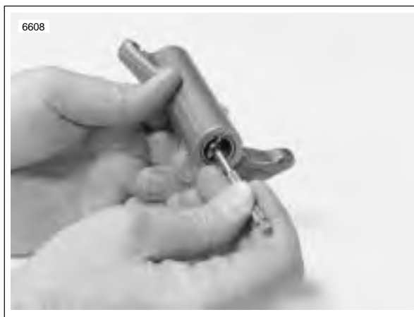
Figure 3-66. Measuring Rocker Arm Bushing Inner Diameter
