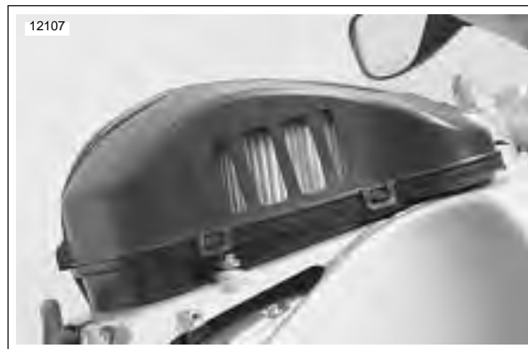
Figure 1-39. Air Intake For Functional Air Cleaner Cover
