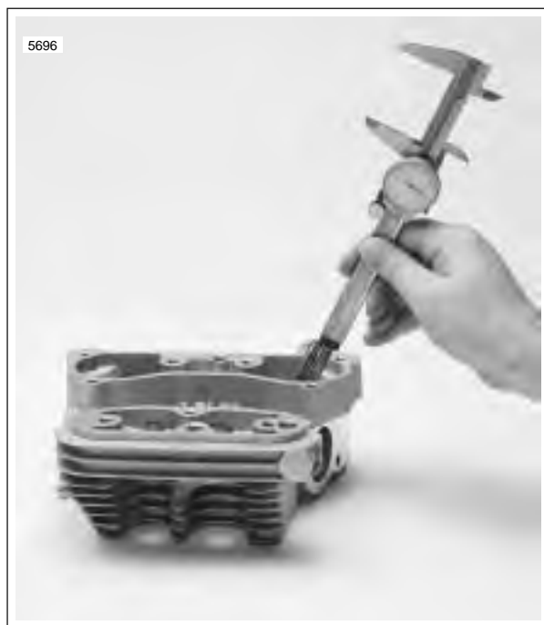
Figure 3-67. Measuring Valve Stem Protrusion
