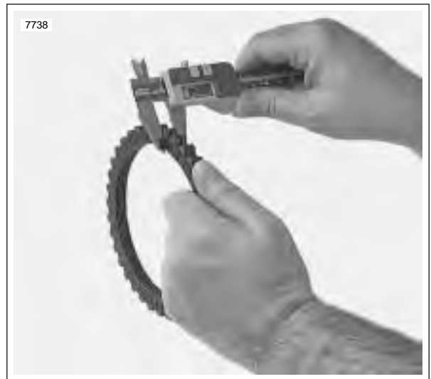
Figure 6-17. Measuring Friction Plates
