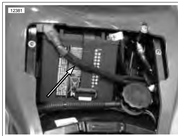
Figure 7-45. Positive Battery Cable 45° to Top of Battery
