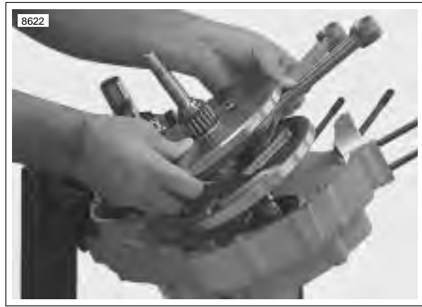
Figure 3-136. Removing Flywheels from Left Crankcase
