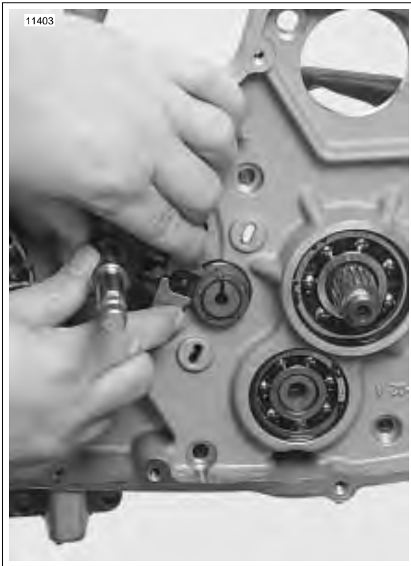
Figure 6-98. Installing Shifter Shaft Assembly
