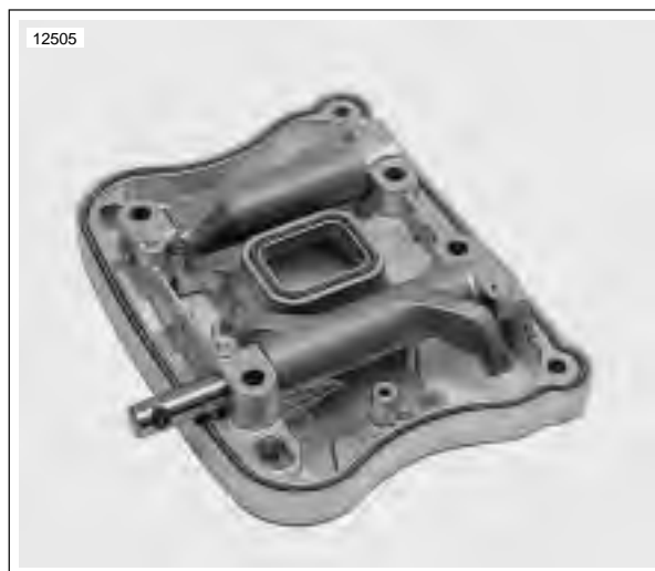
Figure 3-58. Removing Rocker Arm Shafts
