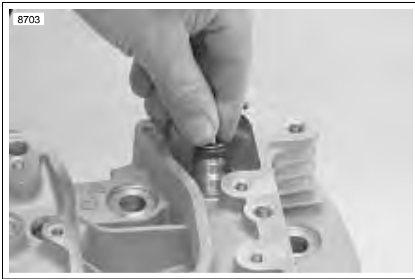
Figure 3-77. Valve Seal and Lower Collar Assembly Installation
