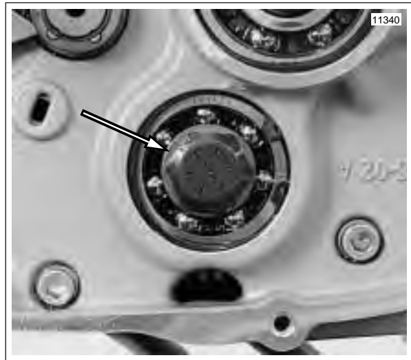
Figure 6-99. Hex Fastener Countershaft Retainer
