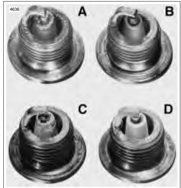
Figure 1-37. Typical Spark Plug Deposits
