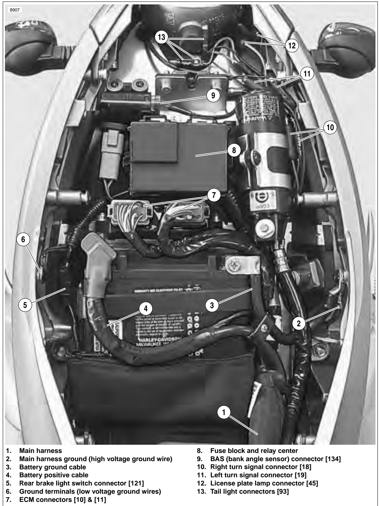
Figure 7-78. Main Harness and Electrical Connectors Under Seat
