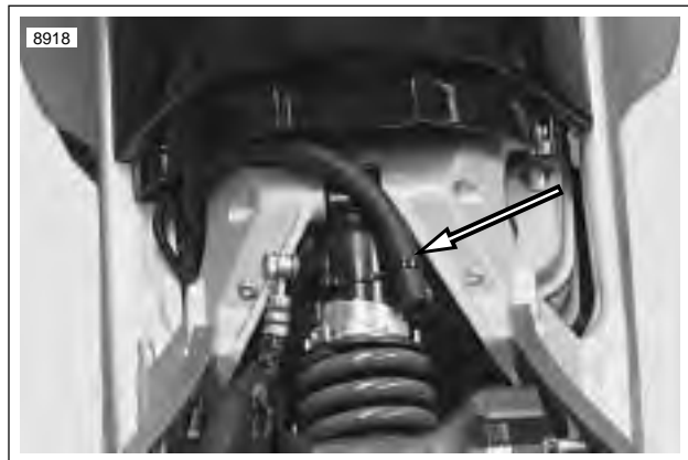
Figure 3-28. Transmission Vent Line
