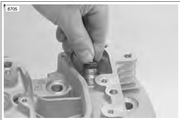
Figure 3-83. Valve Seal and Lower Collar Assembly Installation
