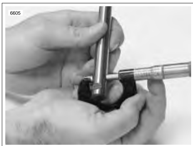
Figure 3-70. Measuring Rocker Arm Shaft Diameter (Rocker Arm Bushing Position)
