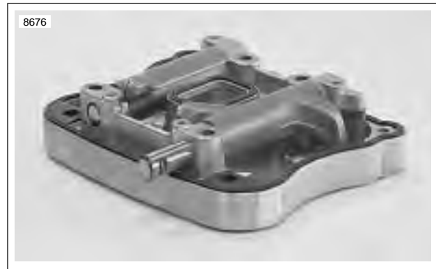
Figure 3-64. Removing Rocker Arm Shafts
