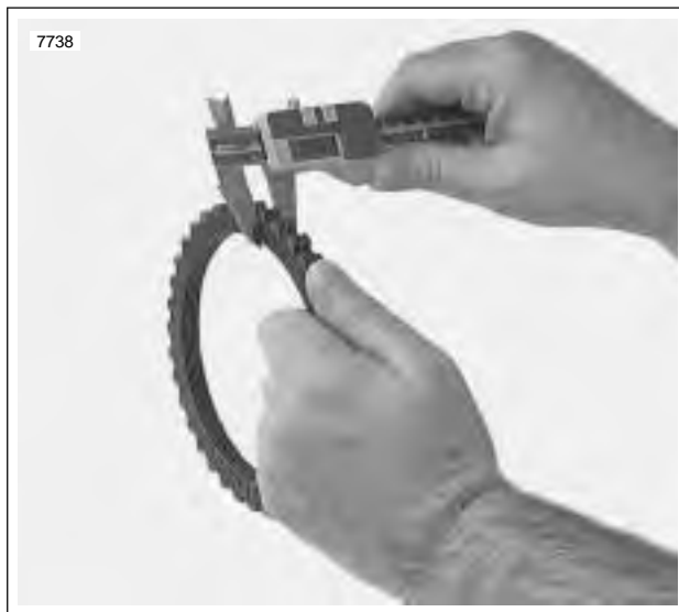
Figure 6-22. Measuring Friction Plates
