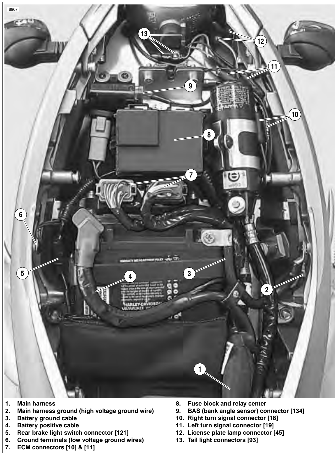
Figure 7-83. Main Harness and Electrical Connectors Under Seat
