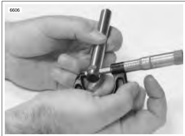
Figure 3-69. Measuring Rocker Arm Shaft Diameter (Rocker Cover Position)
