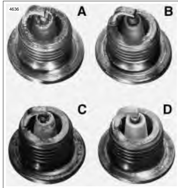
Figure 1-35. Typical Spark Plug Deposits
