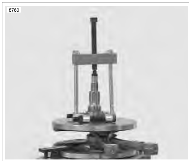
Figure 3-138. Removing Sprocket Shaft Inner Bearing Race
