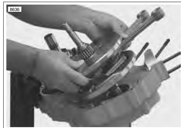
Figure 6-54. Removing Flywheels from Left Case Half
