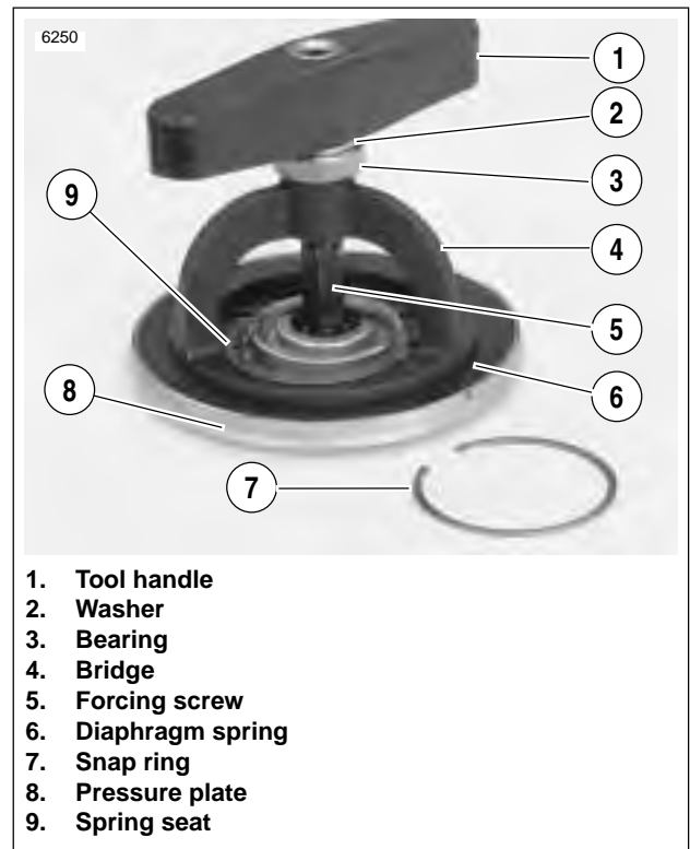
Figure 6-19. Pressure Plate Assembly
