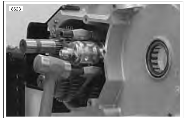
Figure 6-83. Installing Shift Fork Shafts
