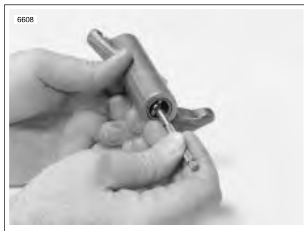
Figure 3-72. Measuring Rocker Arm Bushing Inner Diameter
