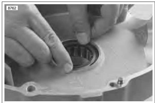
Figure 3-140. Removing Left Main Bearing Retaining Ring
