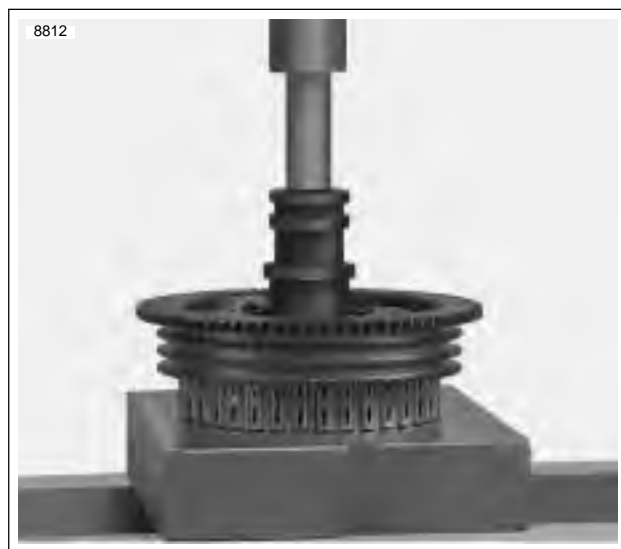
Figure 6-27. Removing Clutch Shell Needle Bearing
