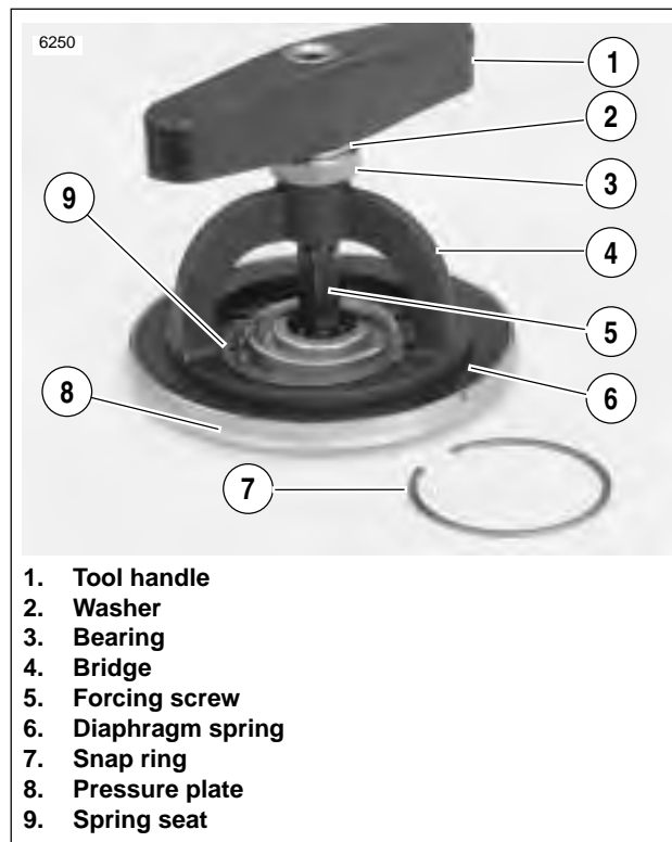
Figure 6-14. Pressure Plate Assembly
