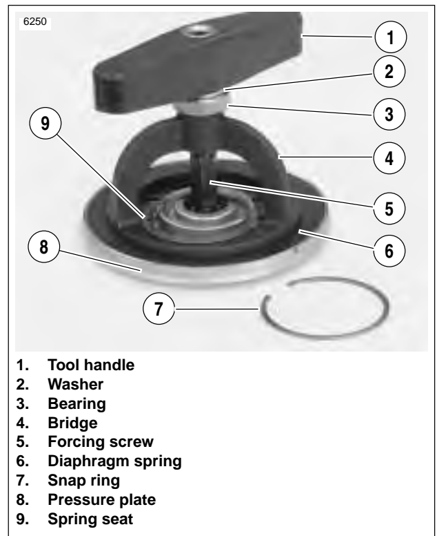
Figure 6-34. Pressure Plate Assembly
