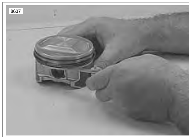
Figure 3-101. Measuring Ring Clearance in Groove
