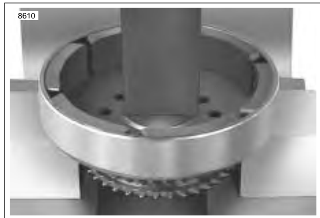
Figure 7-30. Removing Rotor From Sprocket
