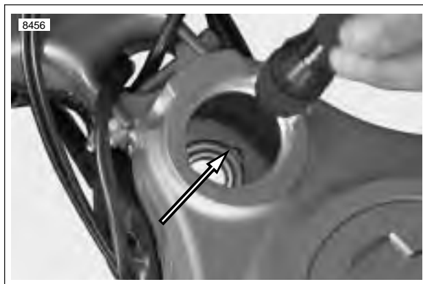
Figure 2-73. Lower Steering Head Bearing Notches (upper bearing removed for clarity)
