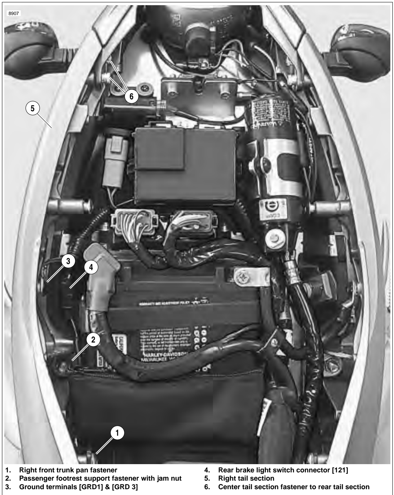
Figure 2-112. Right Side Frame Section
