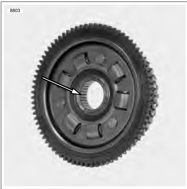
Figure 6-24. New Needle Bearing in Clutch Shell
