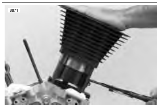
Figure 3-111. Compressing Piston Rings Using Piston Ring Compressor (Part No. HD-96333-51C)
