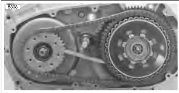
Figure 6-15. Sprocket Locking Link Tool (Part No. HD-38362)
