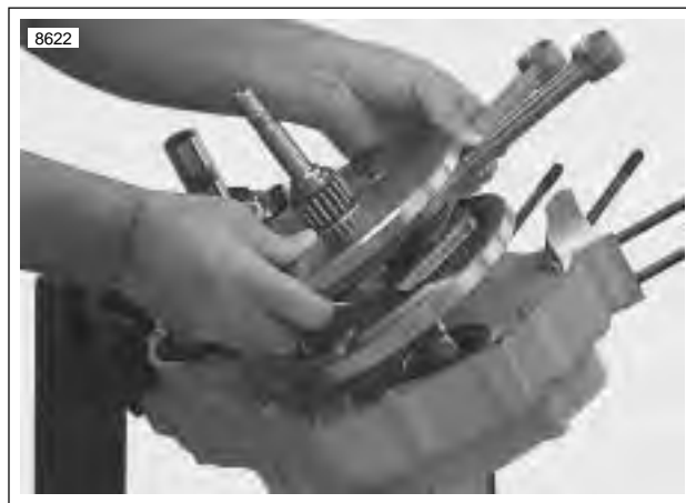
Figure 3-136. Removing Flywheels from Left Crankcase
