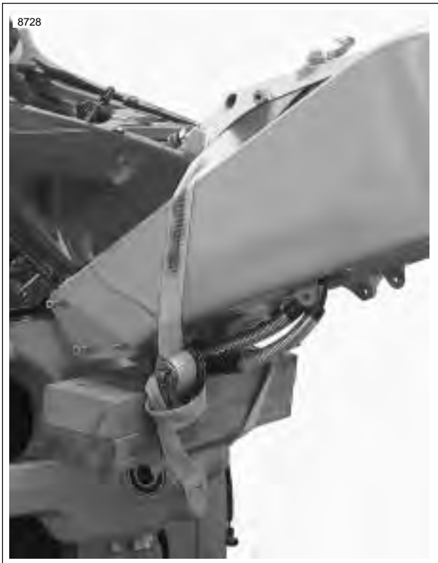
Figure 3-33. Securing Vehicle for Relocation (Typical)
