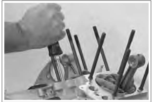
Figure 3-132. Checking Cam Gear End Play
