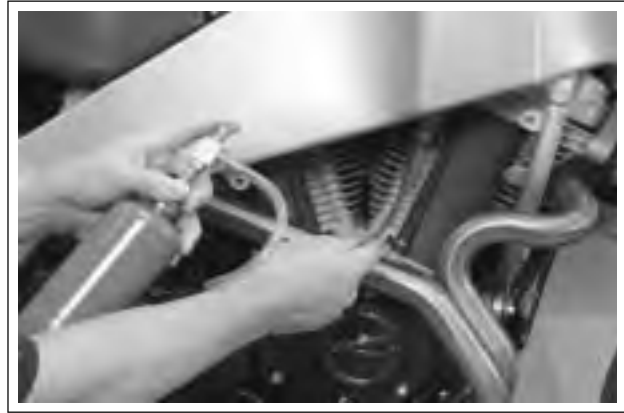
Figure 4-108. Checking for Intake Leak
