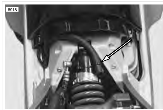
Figure 3-41. Transmission Vent Line
