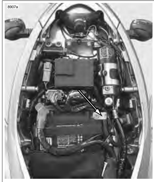
Figure 7-41. Negative Battery Cable
