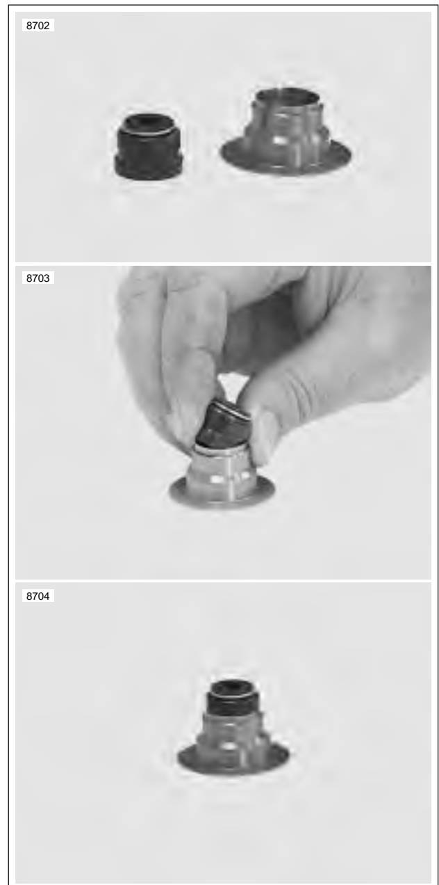
Figure 3-82. Valve Seal and Lower Collar Assembly (seal and lower collar replaced as assembly only)
