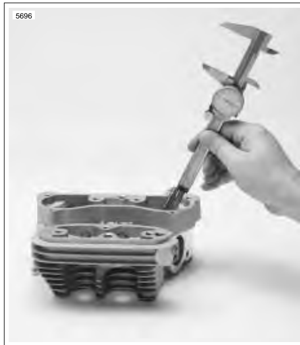
Figure 3-73. Measuring Valve Stem Protrusion
