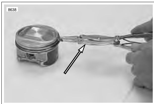
Figure 3-97. Installing Piston Rings Transmission Shaft Retaining Ring Pliers (Part No. J-5586)
