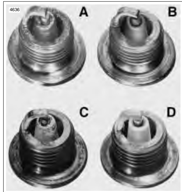
Figure 1-35. Typical Spark Plug Deposits
