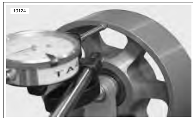
Figure 1-25. Checking Lateral Side Play on Idler Pulley with a Dial Indicator
