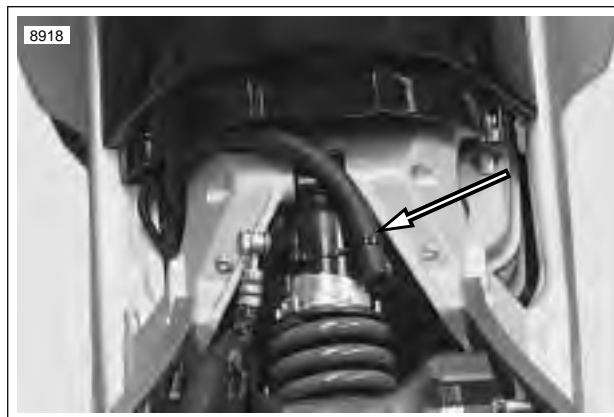
Figure 3-27. Transmission Vent Line
