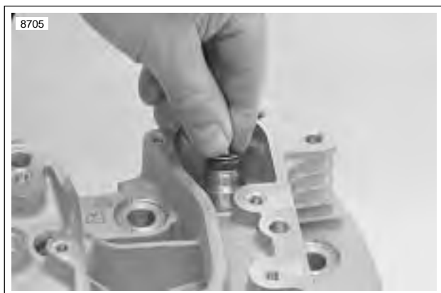
Figure 3-81. Valve Seal and Lower Collar Assembly Installation
