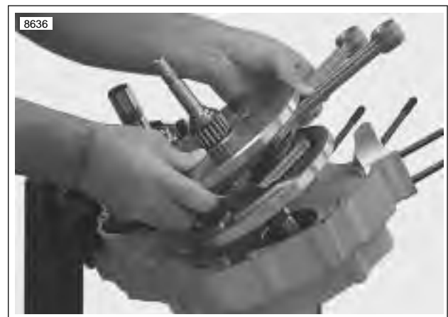
Figure 6-53. Removing Flywheels from Left Case Half
