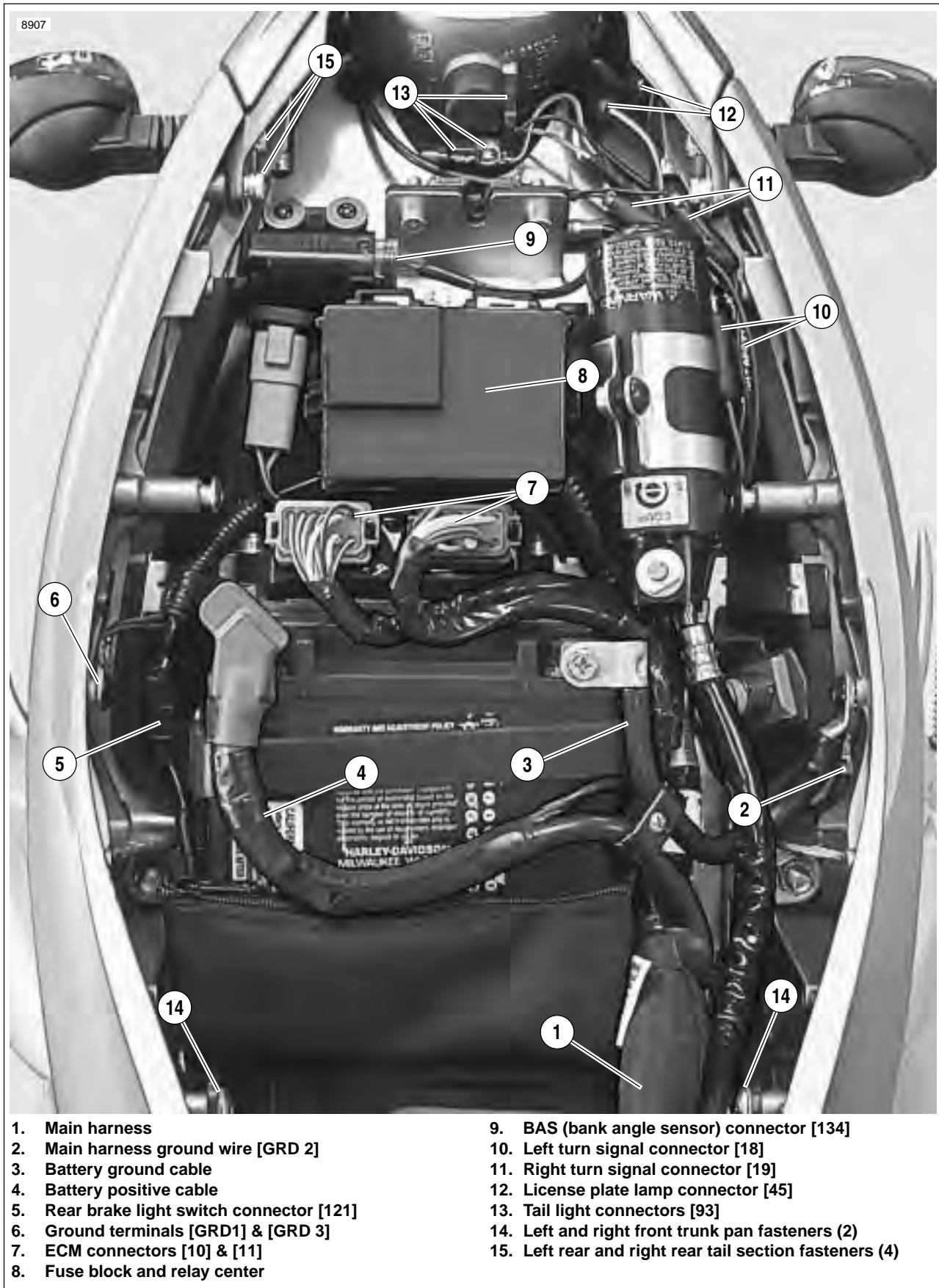
Figure 2-113. Main Harness and Electrical Connectors Under Seat
