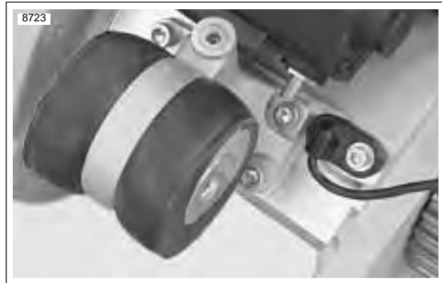
Figure 3-131. Rear Isolator Assembly
