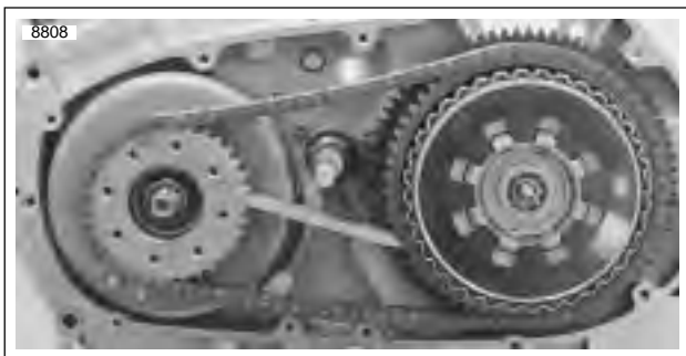
Figure 6-21. Sprocket Locking Link Tool (Part No. HD-38362) for XB9S models and (Part No. HD-46283) for XB12S models.
