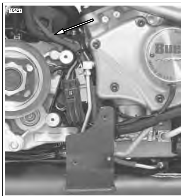
Figure 3-55. Correct Routing of Wiring Harnesses and Interactive Muffler Cable
