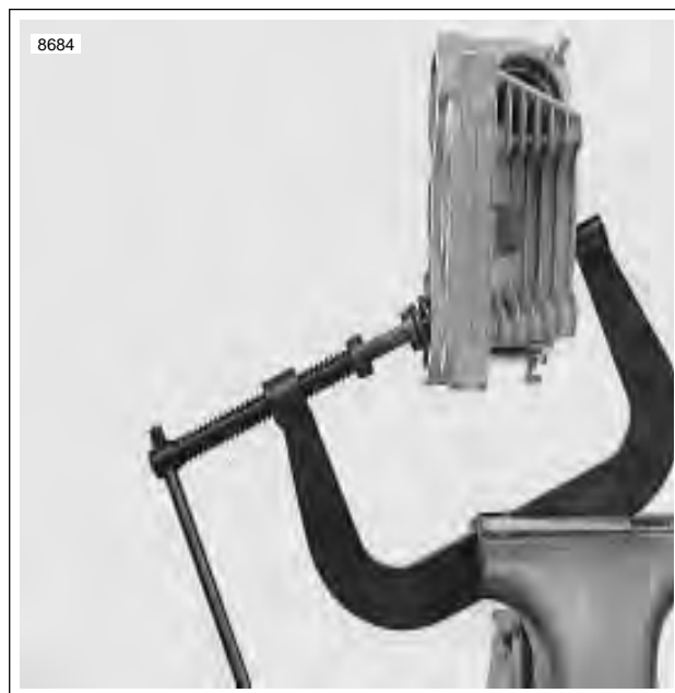
Figure 3-82. Valve Spring Compressor (Part No. HD-34736B)
