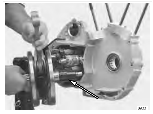
Figure 3-150. Installing Flywheel Assembly with CRANKSHAFT GUIDE (Part No. HD-42326)
