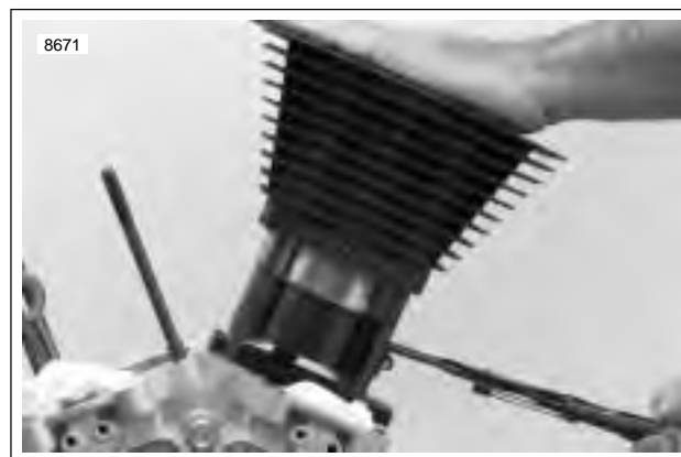
Figure 3-109. Compressing Piston Rings Using Piston Ring Compressor (Part No. HD-96333-51C)
