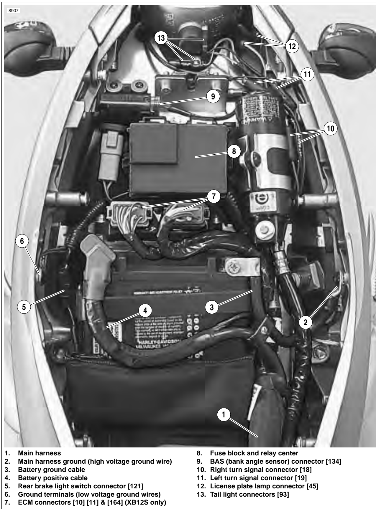
Figure 7-85. Main Harness and Electrical Connectors Under Seat
