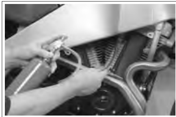
Figure 4-108. Checking for Intake Leak
