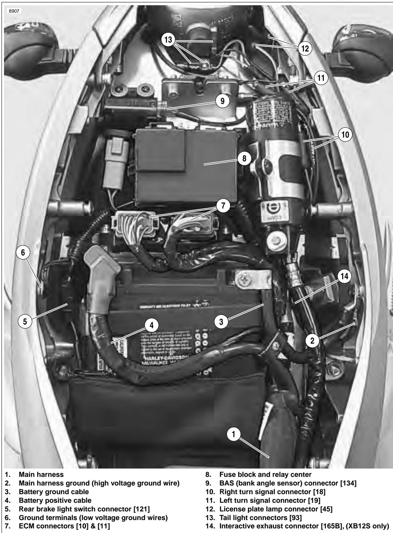
Figure 7-80. Main Harness and Electrical Connectors Under Seat
