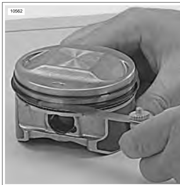
Figure 3-99. Measuring Ring Clearance in Groove
