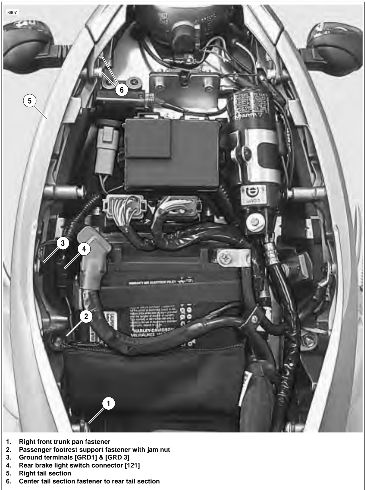
Figure 2-115. Right Side Frame Section
