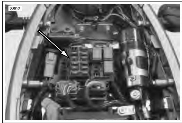
Figure 7-17. Fuse Block (contains diodes)
