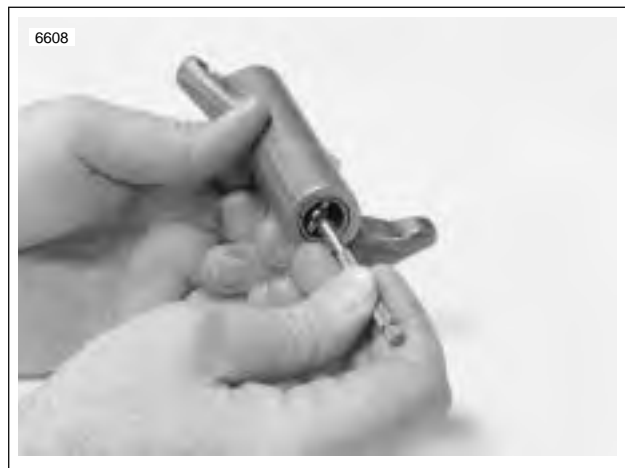
Figure 3-70. Measuring Rocker Arm Bushing Inner Diameter
