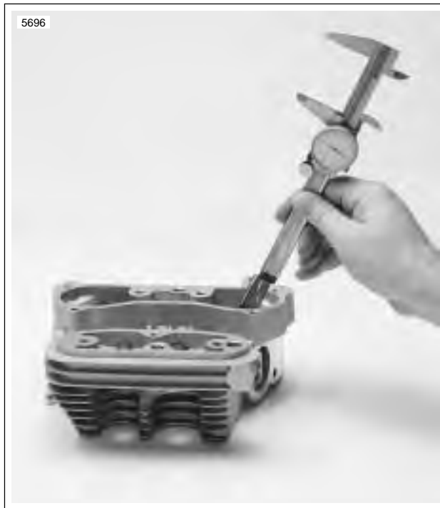
Figure 3-71. Measuring Valve Stem Protrusion
