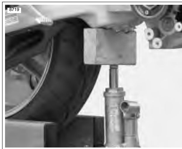
Figure 3-26. Supporting the Swingarm
