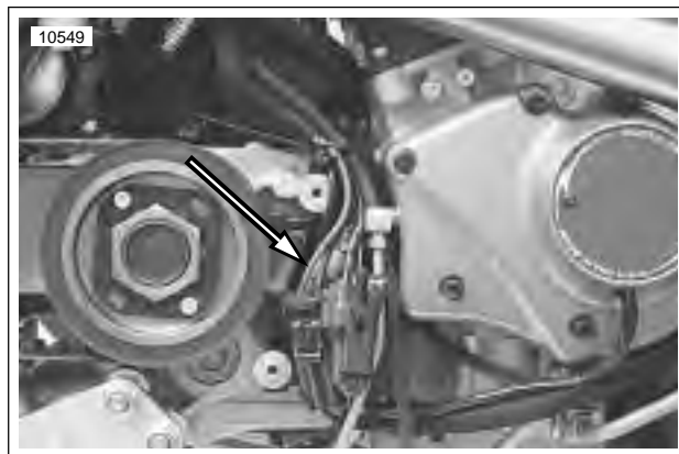
Figure 7-28. Positive Regulator Cable (red wire)
