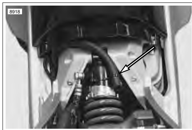
Figure 3-40. Transmission Vent Line
