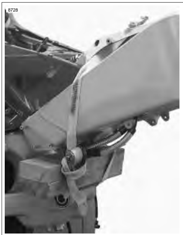
Figure 3-32. Securing Vehicle for Relocation (Typical)
