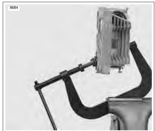
Figure 3-64. Valve Spring Compressor (Part No. HD-34736B)
