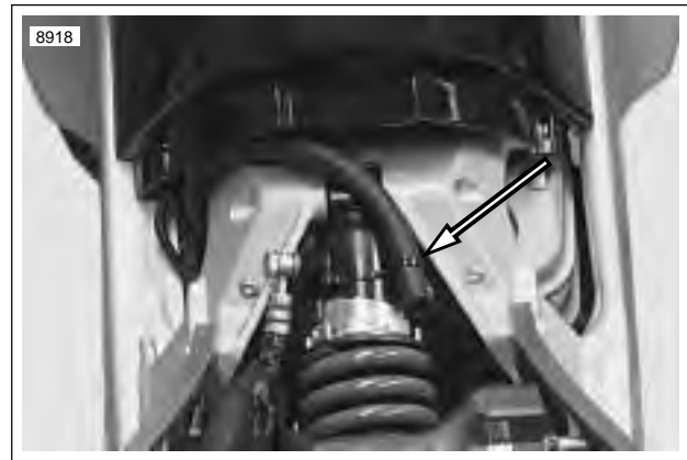
Figure 3-40. Transmission Vent Line
