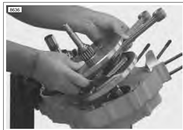
Figure 6-56. Removing Flywheels from Left Case Half
