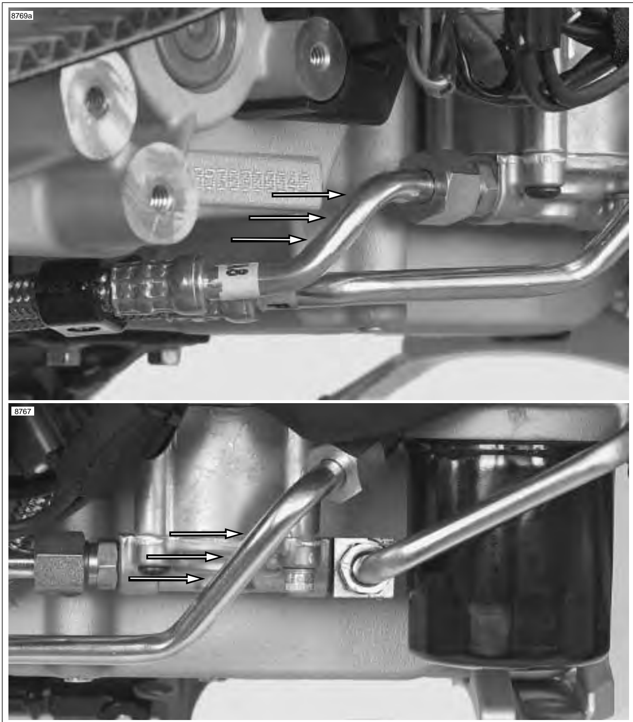
Figure 3-49. Approximate Seven O’Clock Orientation of Oil Feed Line and Oil Return Line at the Oil Pump
