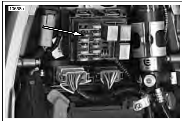
Figure 7-17. Fuse Block (contains diodes)
