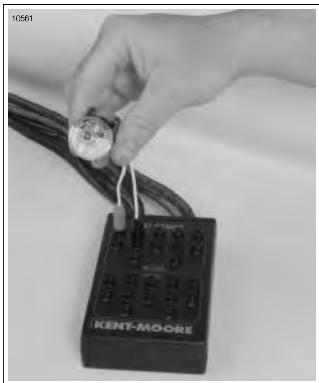
Figure 4-19. Ignition Coil Circuit Test
