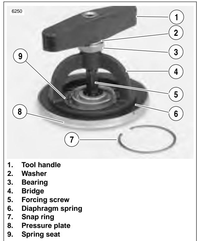
Figure 6-14. Pressure Plate Assembly
