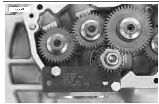
Figure 3-130. Crankshaft Locking Tool (Part No. HD-43984)
