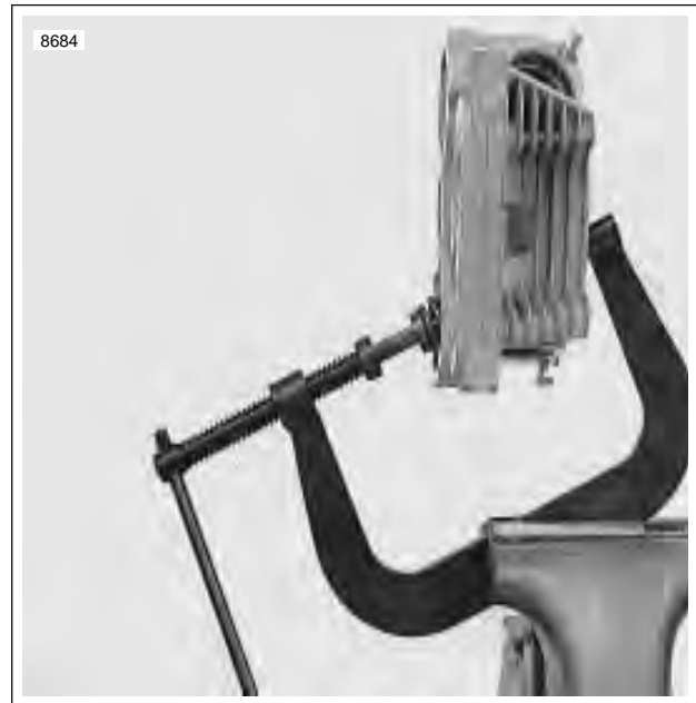
Figure 3-82. Valve Spring Compressor (Part No. HD-34736B)
