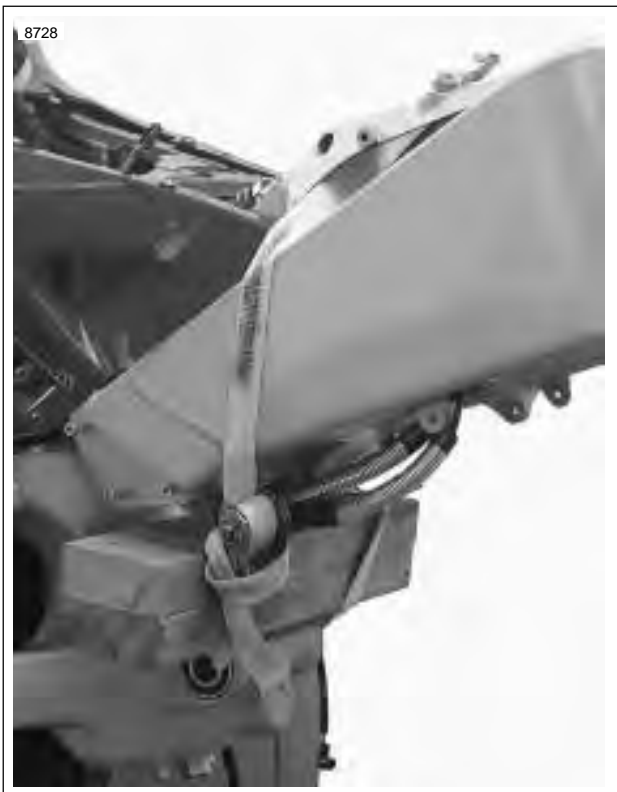
Figure 3-32. Securing Vehicle for Relocation (Typical)
