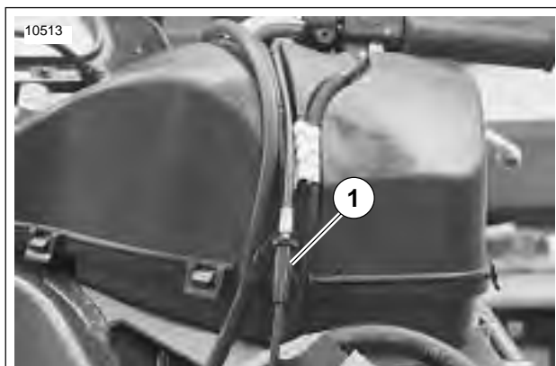
Figure 1-45. Checking For 1/8 in. (3.2 mm) Maximum Free Play In Either Direction For Proper Adjustment
