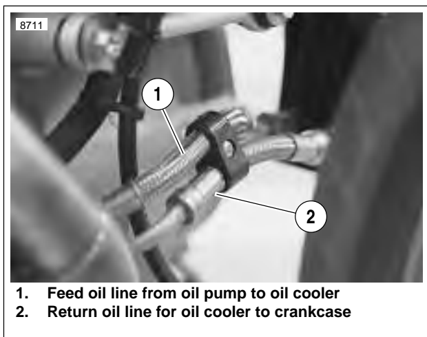
Figure 3-4. Oil Line Connections at Oil Cooler
