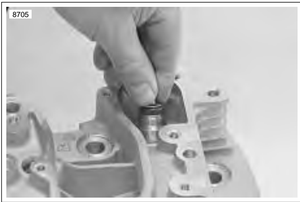
Figure 3-81. Valve Seal and Lower Collar Assembly Installation
