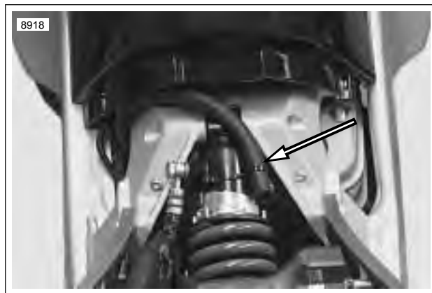
Figure 3-27. Transmission Vent Line
