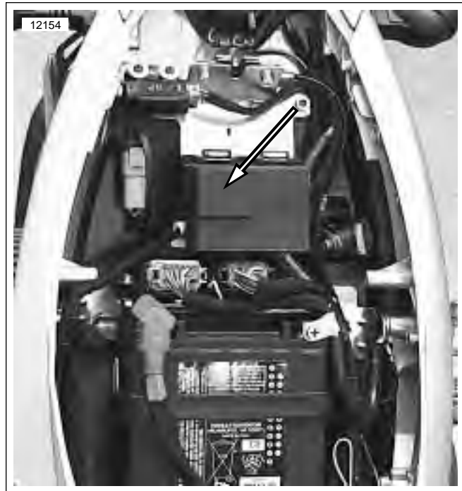
Figure 7-19. Fuse Block (XB12Ss) (contains diode)
