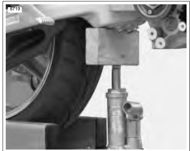
Figure 3-25. Supporting the Swingarm (Typical)
