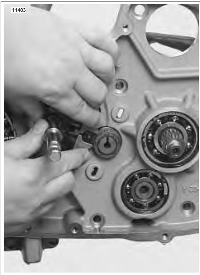
Figure 6-98. Installing Shifter Shaft Assembly
