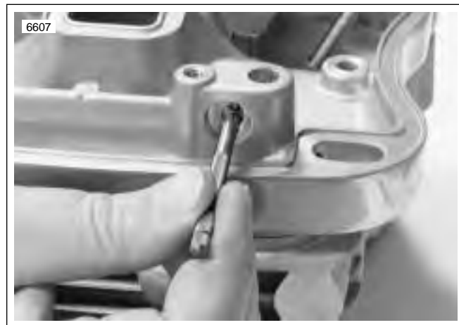
Figure 3-66. Measuring Rocker Arm Shaft Bore Diameter in Lower Rocker Cover
