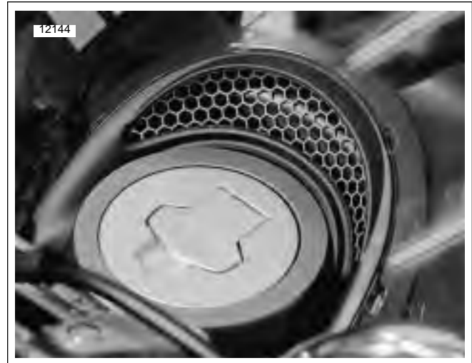
Figure 1-39. Air Intake Screen
