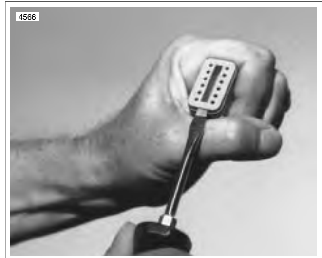
Figure B-6. Remove Secondary Locking Wedge
