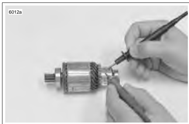
Figure 5-20. Open Armature Test
