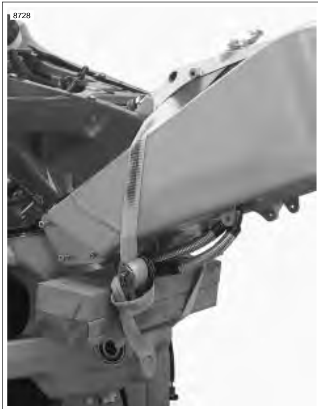
Figure 3-32. Securing Vehicle for Relocation (Typical)
