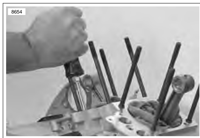
Figure 3-132. Checking Cam Gear End Play
