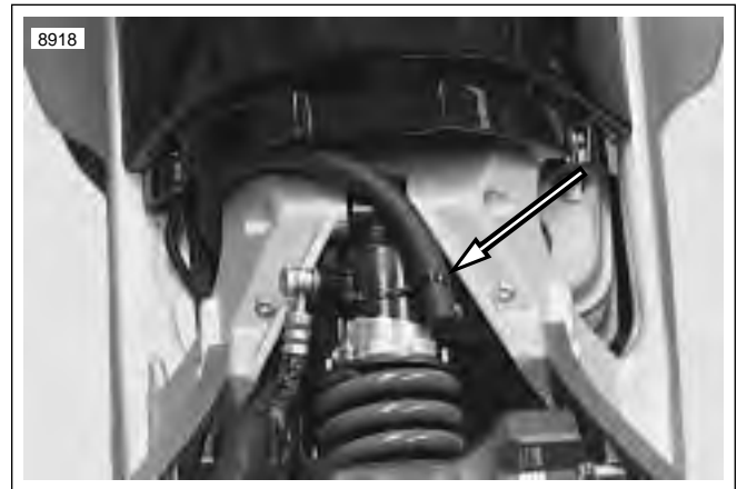
Figure 3-40. Transmission Vent Line
