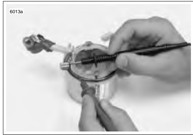
Figure 5-21. Grounded Field Test
