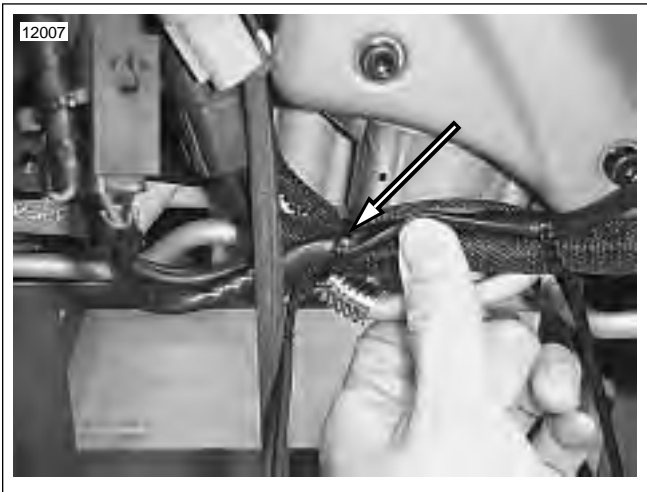
Figure 7-105. Cable Strap Wire Bundle to Return Oil Line
