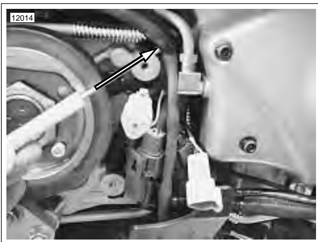
Figure 7-106. Cable Strap Wire Bundle to Return Oil Line, Upper Part of Sprocket Cover
