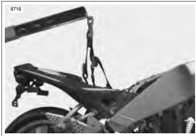
Figure 3-23. Supporting Vehicle for Disassembly (Typical)
