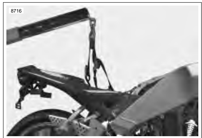
Figure 3-41. Supporting Vehicle for Assembly (Typical)
