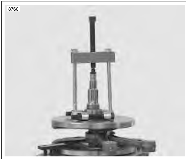
Figure 3-138. Removing Sprocket Shaft Inner Bearing Race
