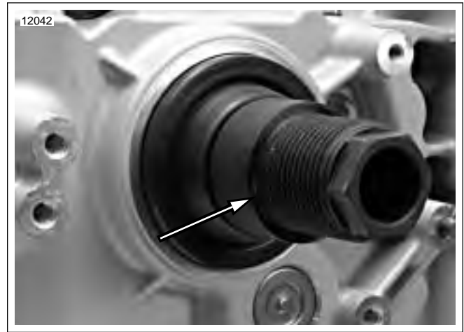
Figure 6-80. Install ADAPTER (Part No. HD-47856-4) (Typical)
