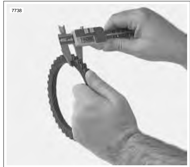
Figure 6-17. Measuring Friction Plates
