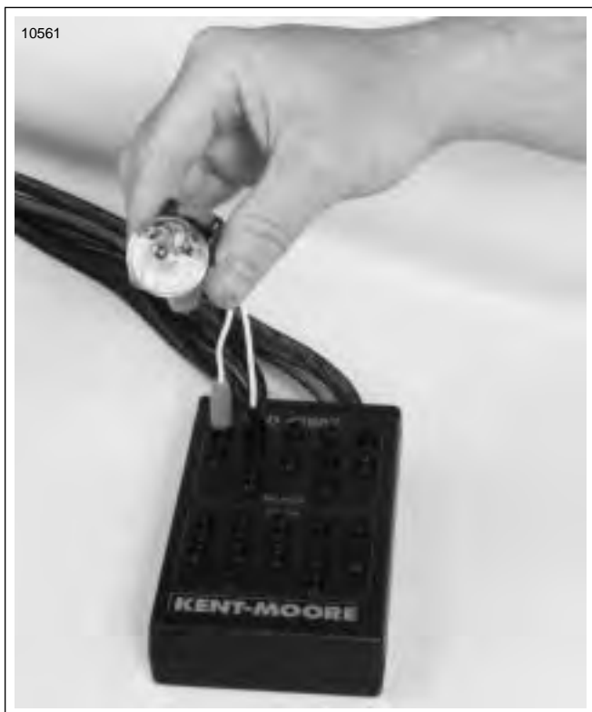
Figure 4-21. Ignition Coil Circuit Test
