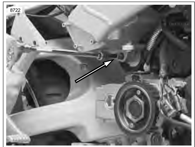
Figure 3-42. Installing Rear Isolator Bolt (Typical)
