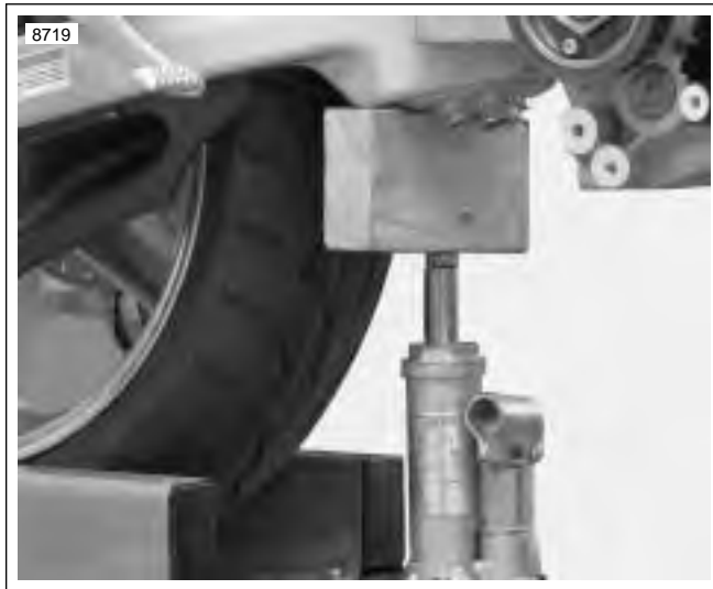
Figure 3-38. Supporting the Swingarm (Typical)
