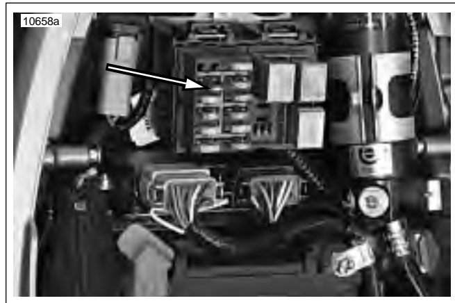
Figure 7-18. Fuse Block (contains diode)
