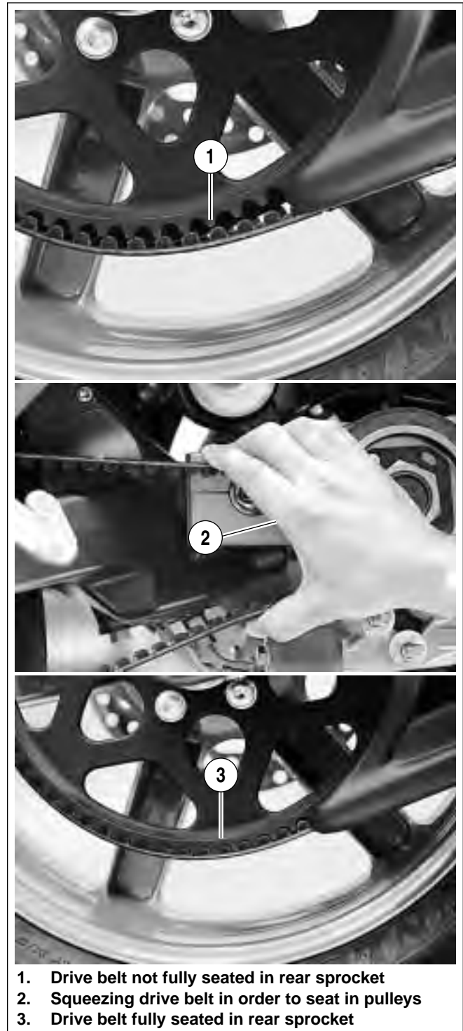
Figure 6-42. Seating Drive Belt Into Pulley Teeth
