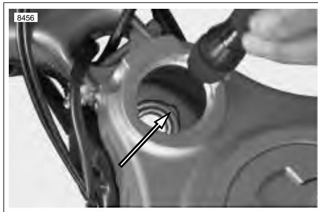
Figure 2-77. Lower Steering Head Bearing Notches (upper bearing removed for clarity)
