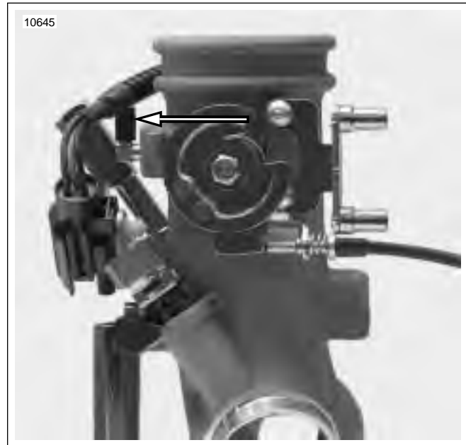
Figure 4-123. Emissions Hose Attachment, California Models Only
