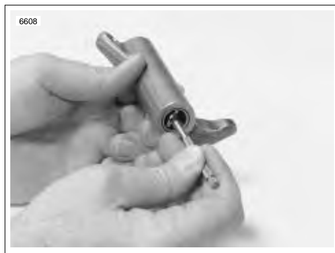
Figure 3-67. Measuring Rocker Arm Bushing Inner Diameter
