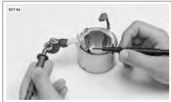
Figure 5-22. Open Field Test
