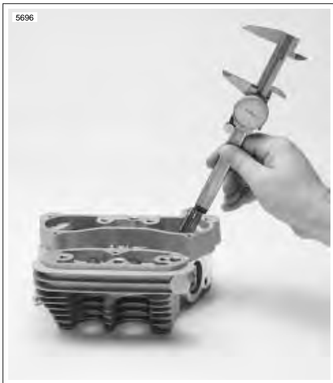
Figure 3-68. Measuring Valve Stem Protrusion
