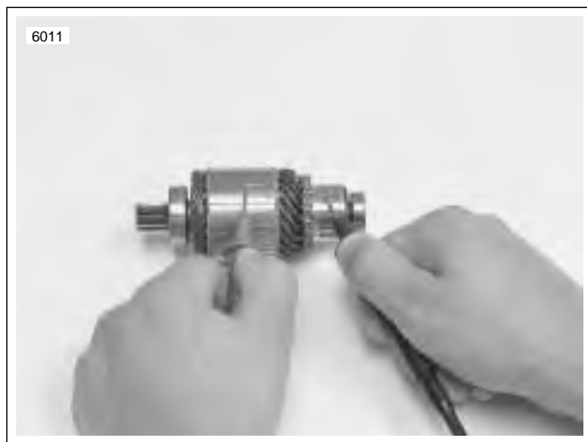
Figure 5-19. Grounded Armature Test
