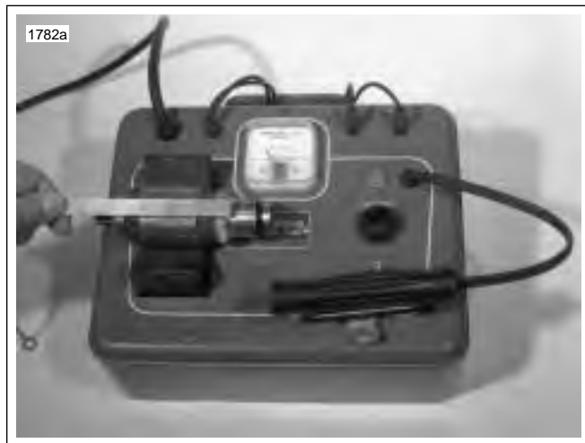
Figure 5-18. Shorted Armature Test Using Growler
