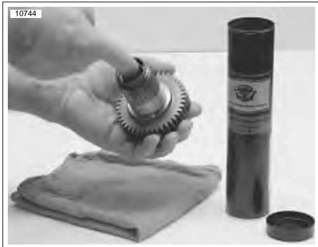
Figure 6-76. Lubricating Main Drive Gear Needle Bearings
