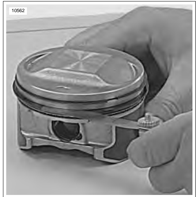
Figure 3-96. Measuring Ring Clearance in Groove
