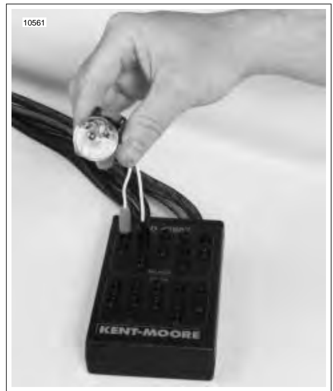
Figure 4-51. Testing Ignition Coil Connectors
