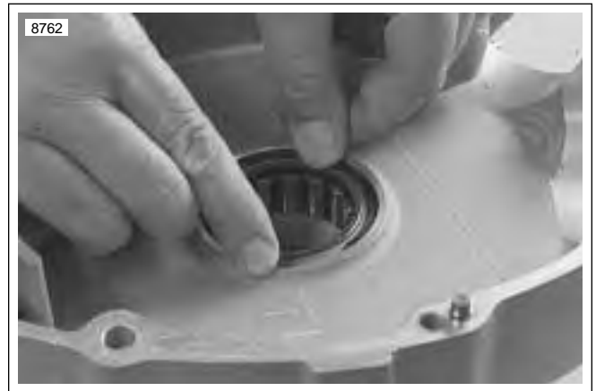
Figure 3-140. Removing Sprocket Shaft Bearing Retaining Ring
