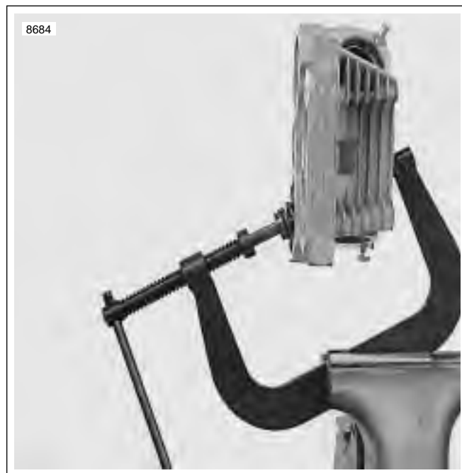
Figure 3-79. Valve Spring Compressor (Part No. HD-34736B)
