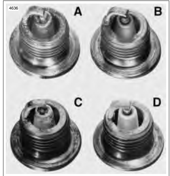
Figure 1-37. Typical Spark Plug Deposits
