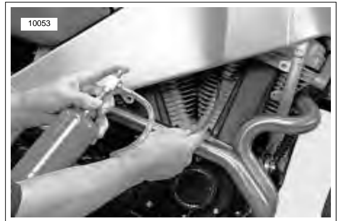
Figure 4-113. Checking for Intake Leak
