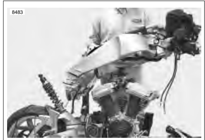
Figure 2-89. Lift Frame Off Motorcycle (Typical)
