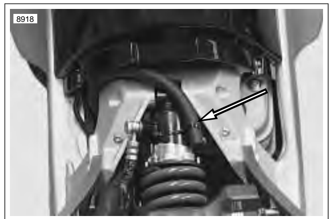
Figure 3-26. Transmission Vent Line
