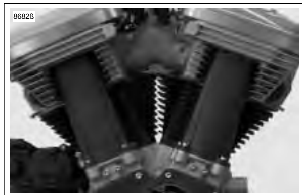
Figure 3-79. Push Rod Locations
