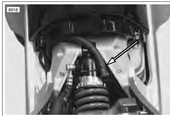
Figure 3-39. Transmission Vent Line
