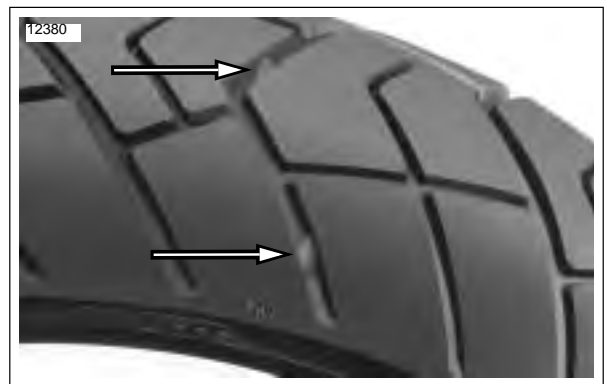
Figure 1-18. Tire Wear Indicators (TWI) Pirelli Scorpion Sync (City Cross only)
