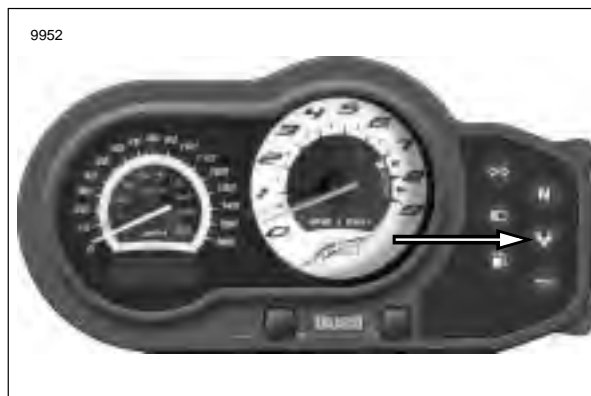
Figure 4-16. Check Engine Lamp
