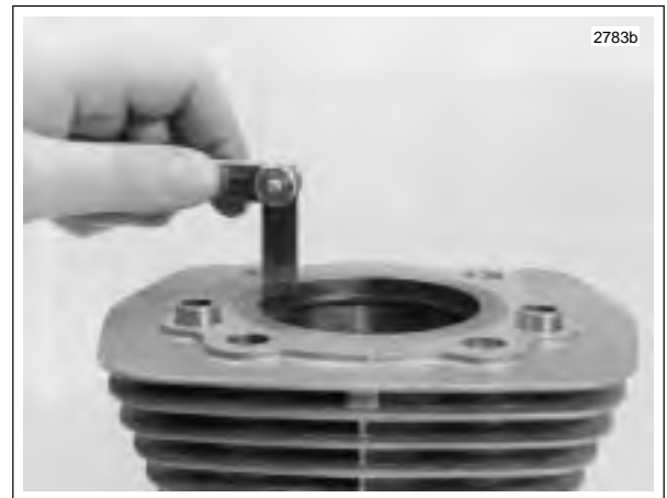
Figure 3-92. Measuring Ring End Gap
