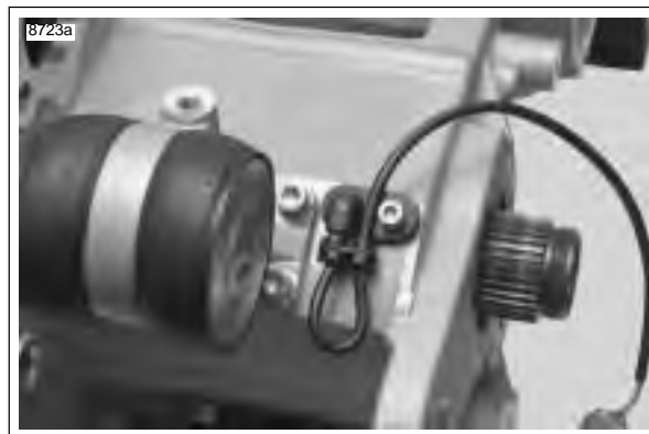
Figure 3-133. Rear Isolator Assembly
