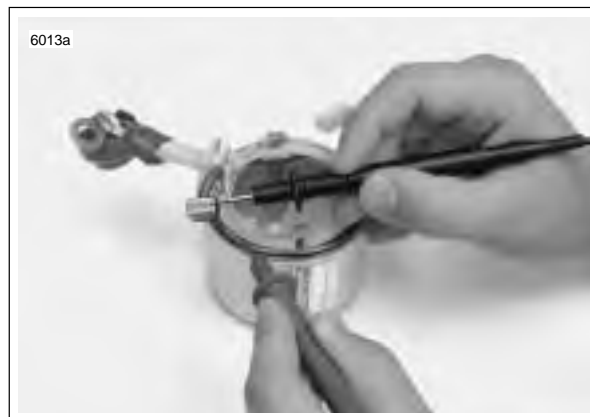
Figure 5-21. Grounded Field Test
