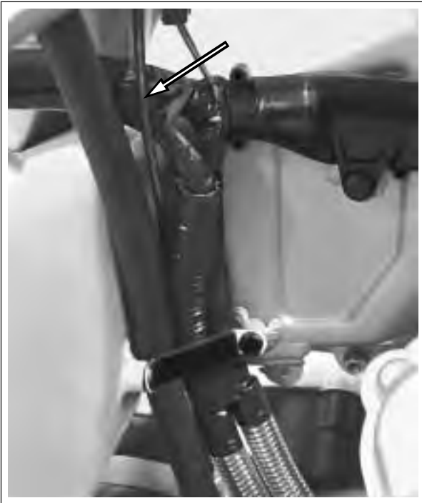
Figure 7-24. Interactive Exhaust Cable Behind Wire Harness Strap and Guide
