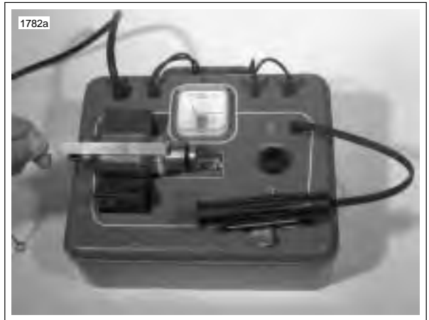
Figure 5-18. Shorted Armature Test Using Growler
