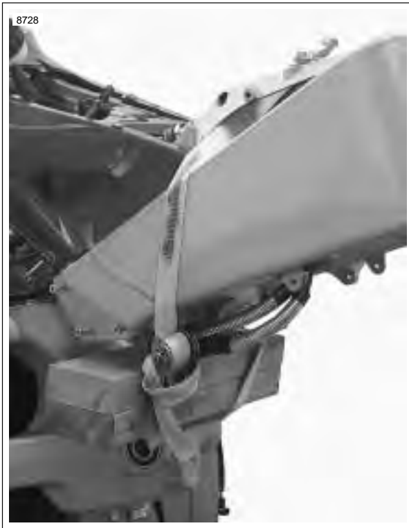
Figure 3-31. Securing Vehicle for Relocation (Typical)
