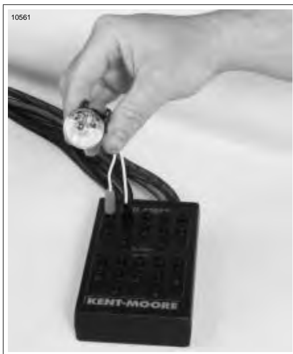
Figure 4-21. Ignition Coil Circuit Test
