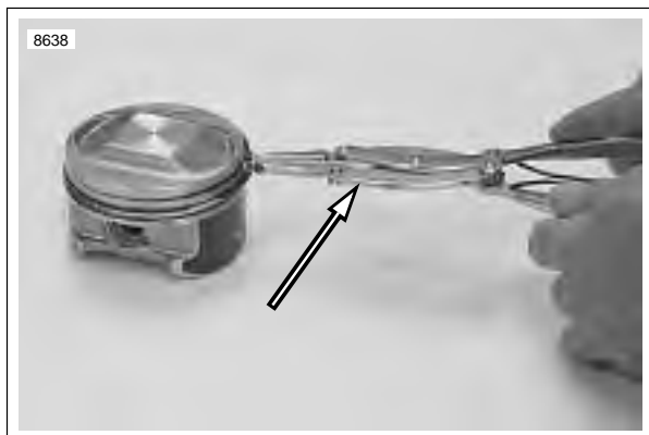
Figure 3-93. Installing Piston Rings Transmission Shaft Retaining Ring Pliers (Part No. J-5586)
