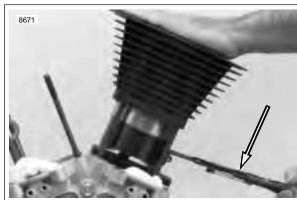
Figure 3-105. Compressing Piston Rings Using Piston Ring Compressor (Part No. HD-96333-51C)
