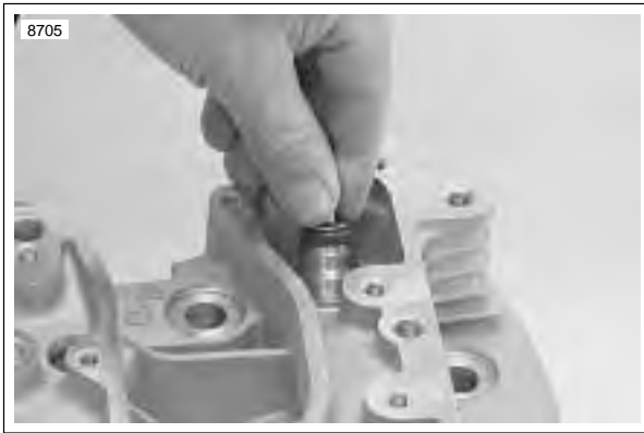
Figure 3-77. Valve Seal and Lower Collar Assembly Installation
