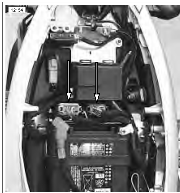
Figure 4-56. ECM Connections (XB12Ss)
