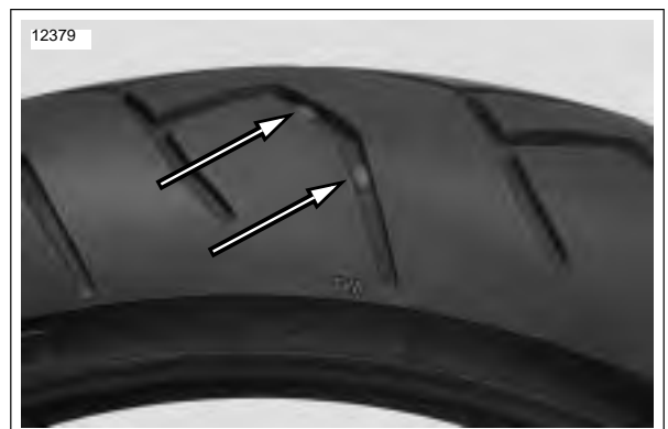
Figure 1-19. Tire Wear Indicator Bars (TWI) Pirelli Diablo T
