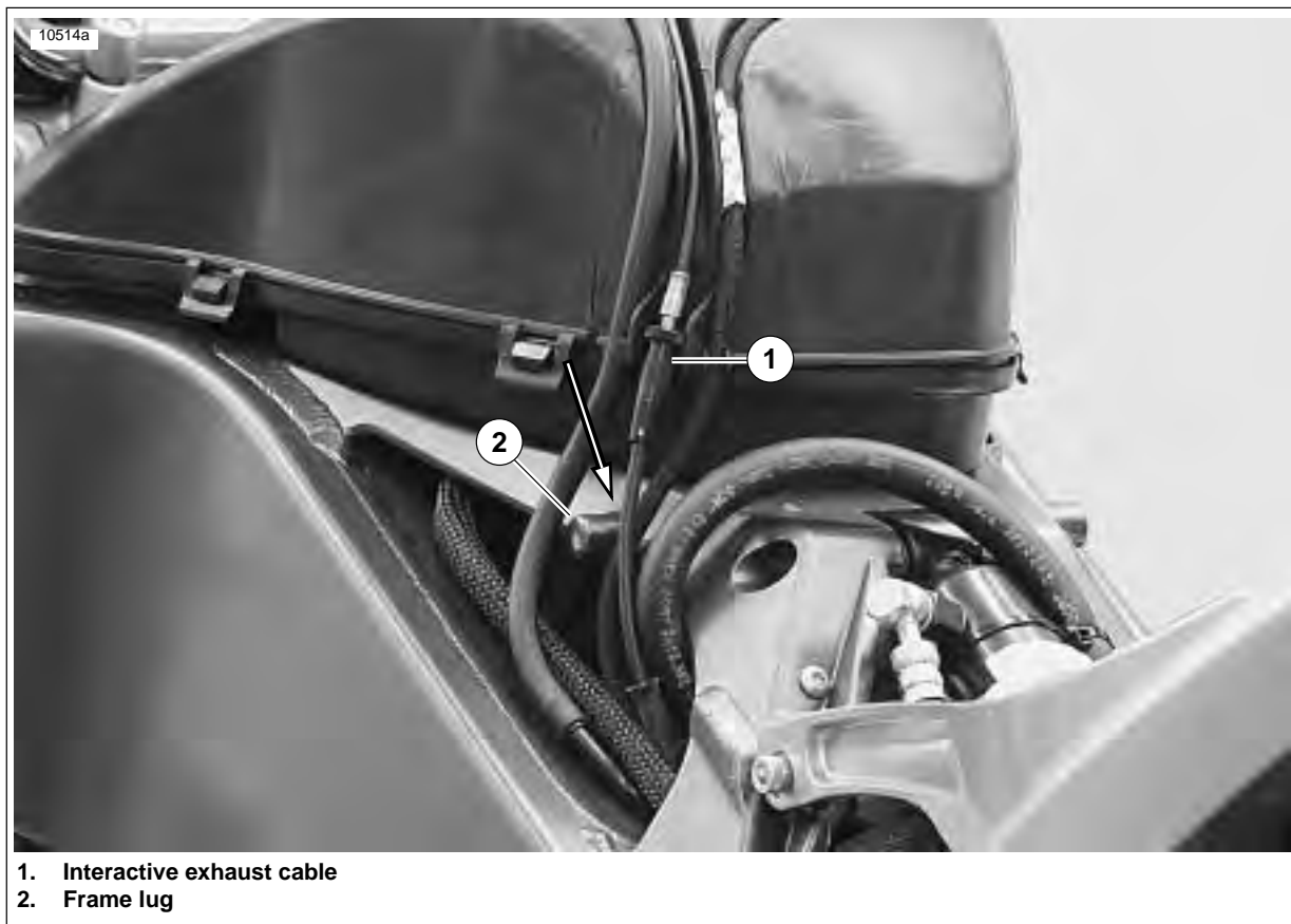
Figure 1-50. Correct Cable Routing Behind Frame Lug
