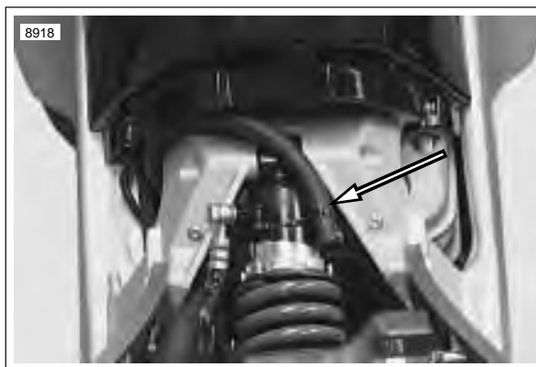
Figure 3-25. Transmission Vent Line
