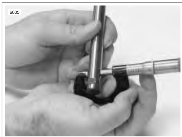
Figure 3-64. Measuring Rocker Arm Shaft Diameter (Rocker Arm Bushing Position)
