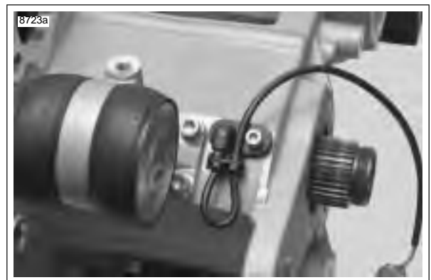
Figure 6-51. Rear Isolator Assembly
