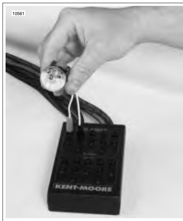
Figure 4-51. Testing Ignition Coil Connectors
