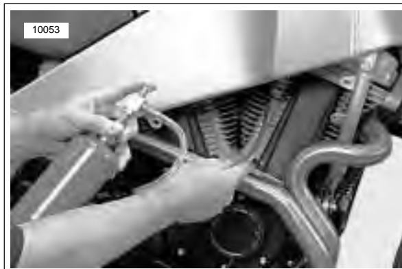
Figure 4-116. Checking for Intake Leak
