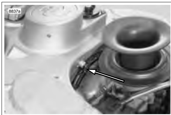
Figure 7-90. Wire Harness Clip
