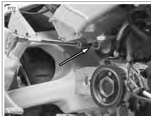
Figure 3-41. Installing Rear Isolator Bolt (Typical)
