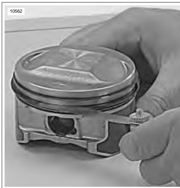
Figure 3-95. Measuring Ring Clearance in Groove
