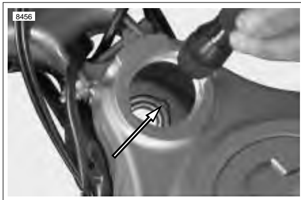
Figure 2-76. Lower Steering Head Bearing Notches (upper bearing removed for clarity)
