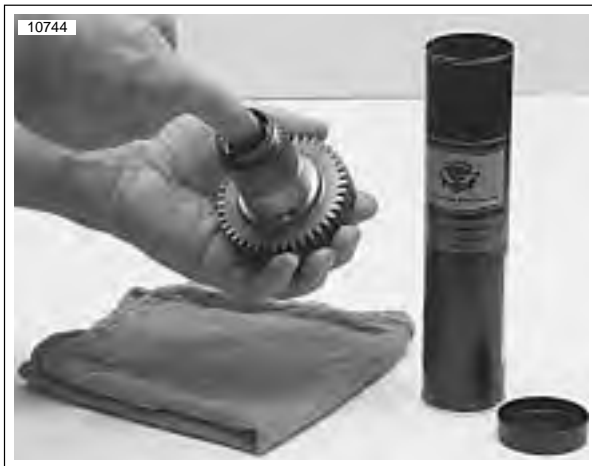
Figure 6-76. Lubricating Main Drive Gear Needle Bearings
