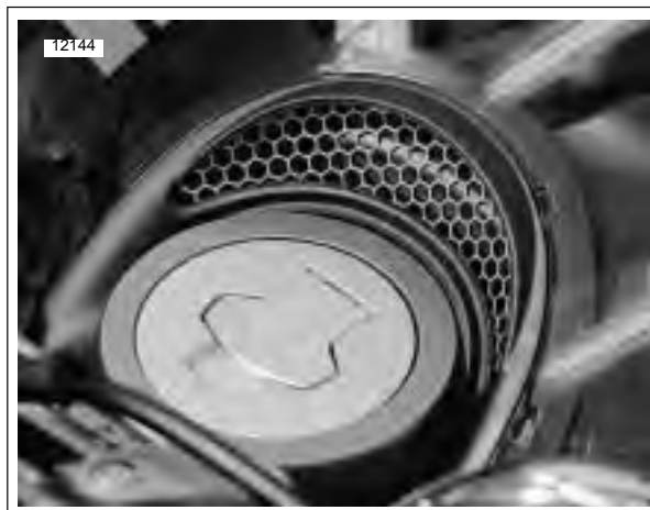
Figure 1-39. Air Intake Screen
