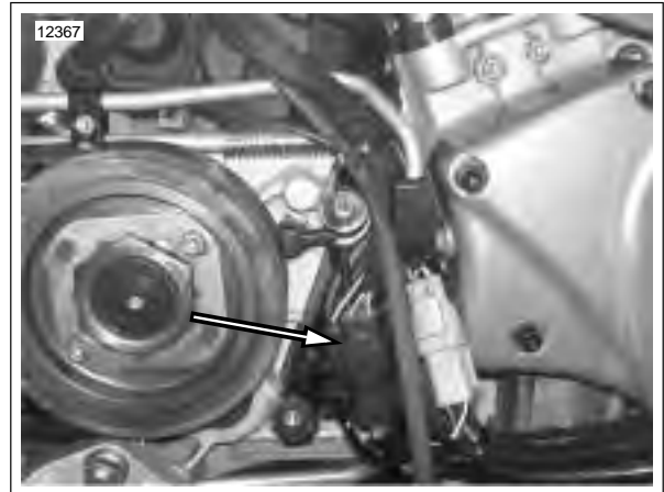
Figure 4-72. Cam Position Sensor Connector [14]
