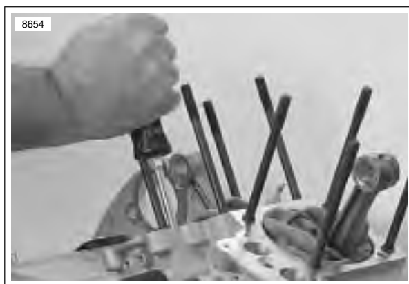
Figure 3-132. Checking Cam Gear End Play
