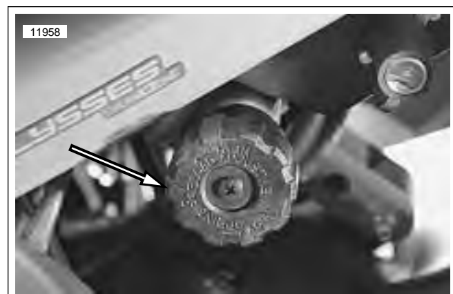
Figure 2-95. Rear Shock Absorber Preload Adjuster Knob
