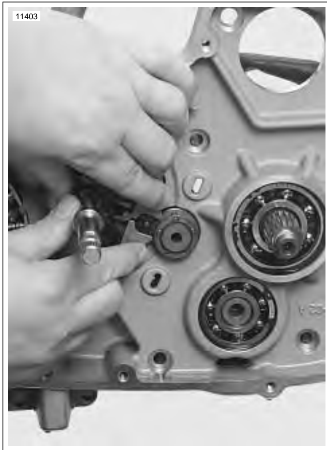
Figure 6-49. Removing Shifter Shaft Assembly
