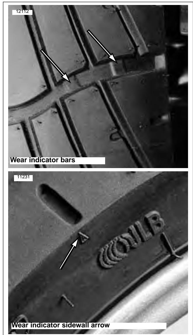
Figure 1-24. Tire Wear Indicators
