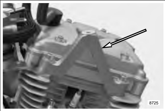
Figure 3-27. Center Tie Bar Mount
