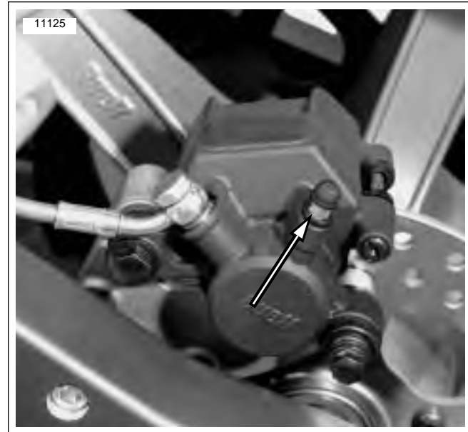
Figure 2-51. Brake Bleeder Valve, Rear Caliper
