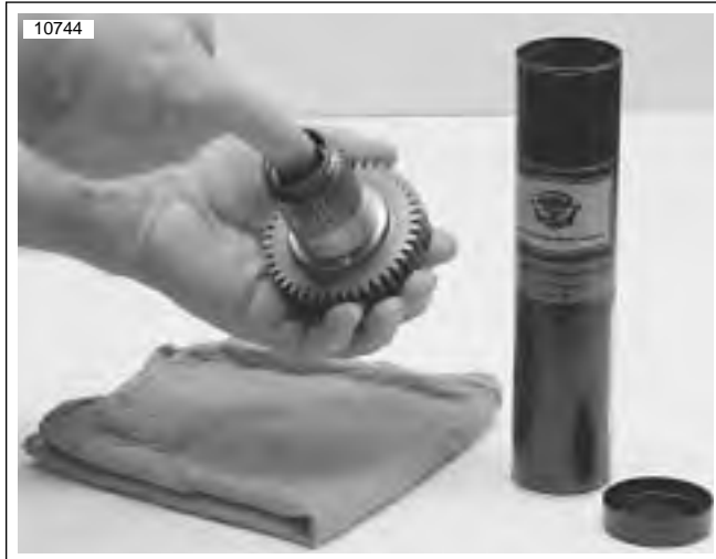
Figure 6-75. Lubricating Main Drive Gear Needle Bearings
