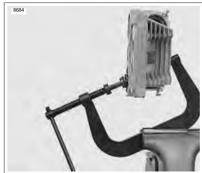
Figure 3-61. Valve Spring Compressor (Part No. HD-34736B)
