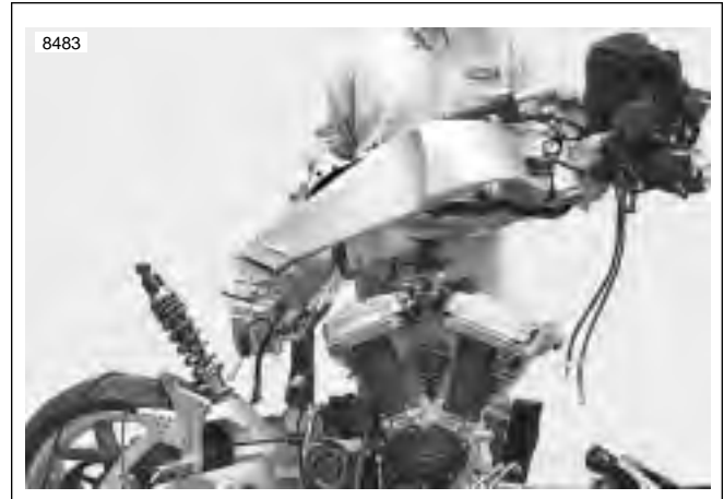
Figure 2-90. Lift Frame Off Motorcycle (Typical)
