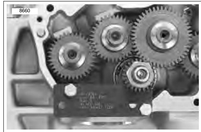
Figure 3-132. Crankshaft Locking Tool (Part No. HD-43984)
