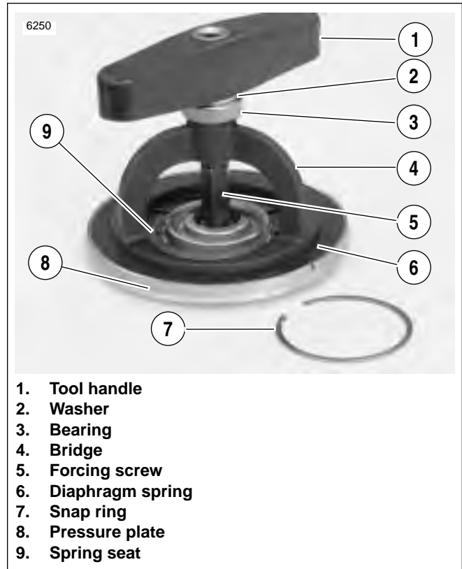
Figure 6-14. Pressure Plate Assembly
