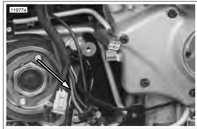
Figure 7-28. Positive Regulator Cable (red wire)
