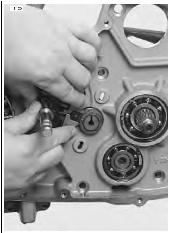
Figure 6-97. Installing Shifter Shaft Assembly
