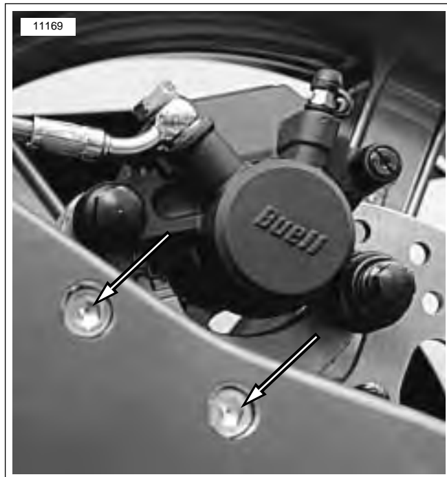
Figure 2-21. Rear Brake Caliper Carrier Fasteners
