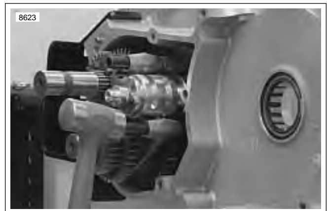
Figure 6-89. Installing Shift Fork Shafts
