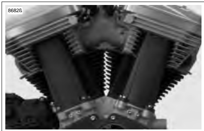
Figure 3-80. Push Rod Locations
