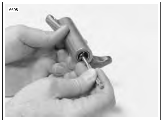
Figure 3-67. Measuring Rocker Arm Bushing Inner Diameter
