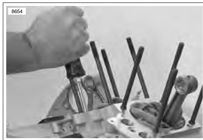
Figure 3-134. Checking Cam Gear End Play
