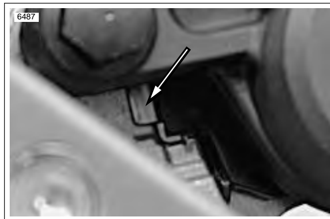
Figure 1-21. Rear Brake Pad Spring Location
