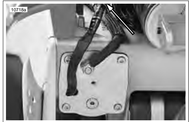
Figure 4-97. Fuel Pump connector [86] (swingarm removed for illustration)
