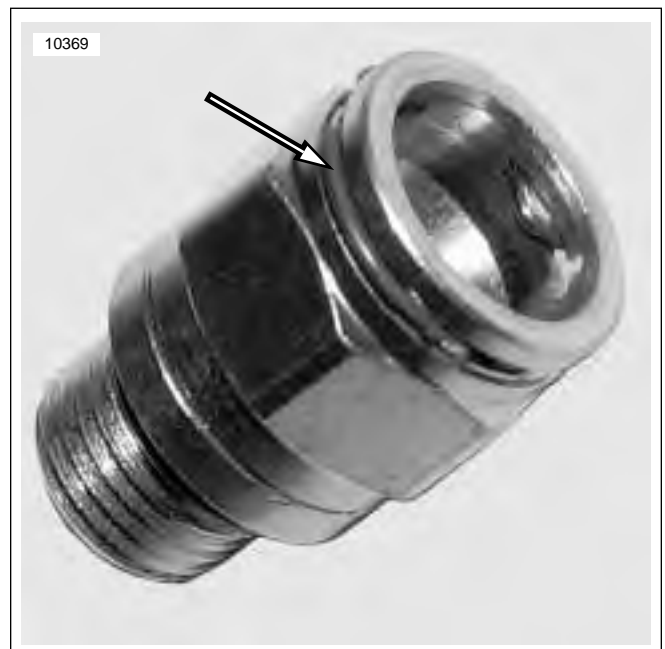
Figure 3-111. Oil Line Fitting with Spring Clip
