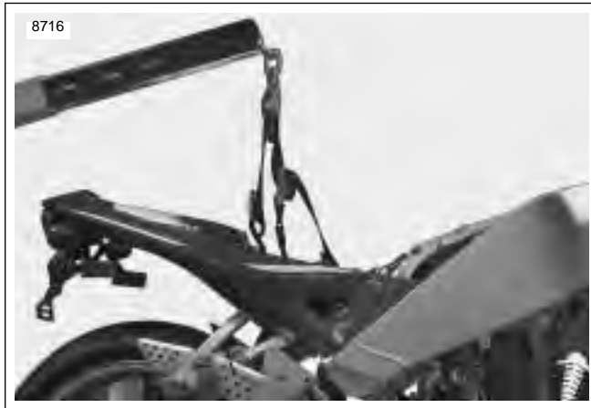
Figure 3-23. Supporting Vehicle for Disassembly (Typical)
