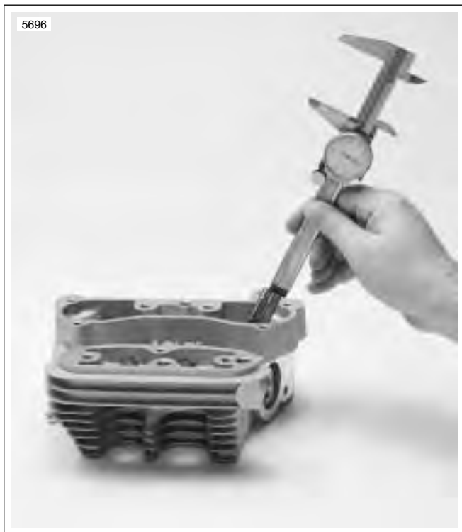
Figure 3-68. Measuring Valve Stem Protrusion
