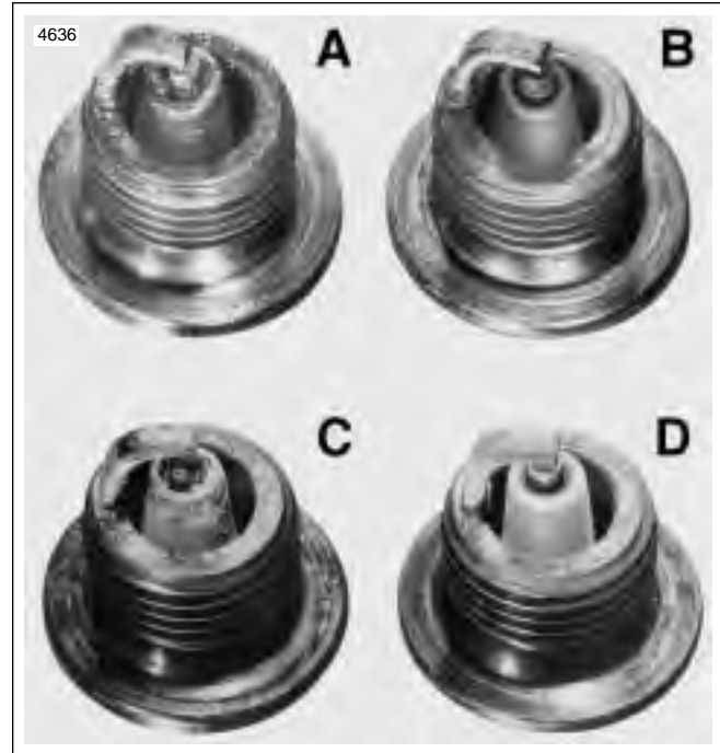
Figure 1-41. Typical Spark Plug Deposits
