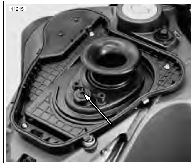
Figure 4-78. Intake Air Temperature Sensor Installed
