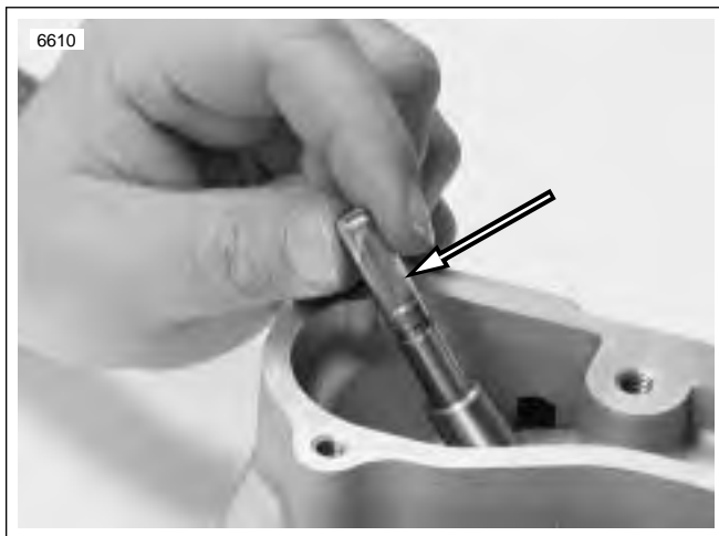
Figure 3-76. Valve Guide Seal Protector Sleeve
