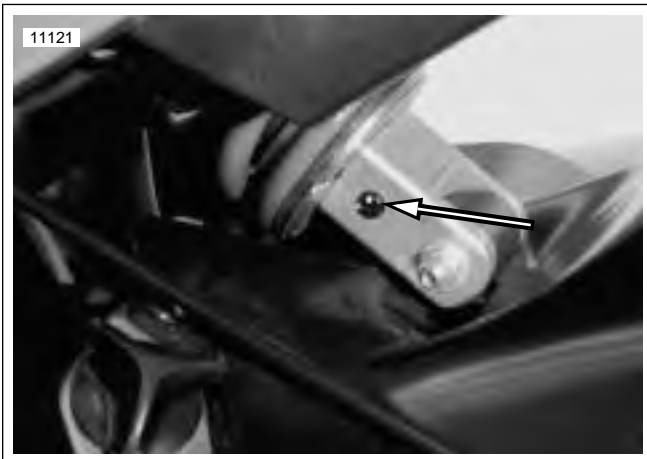
Figure 1-38. Rear Shock Rebound Adjustment Dial
