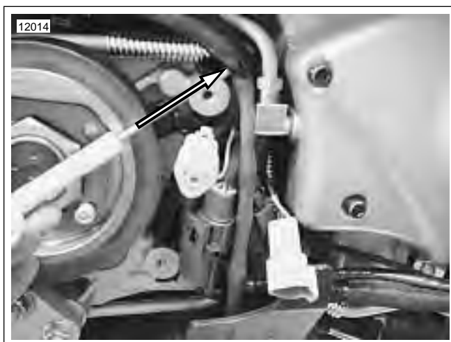
Figure 7-99. Cable Strap Wire Bundle to Return Oil Line, Upper Part of Sprocket Cover
