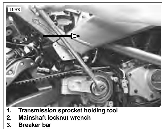
Figure 6-101. Removing Transmission Sprocket Locknut
