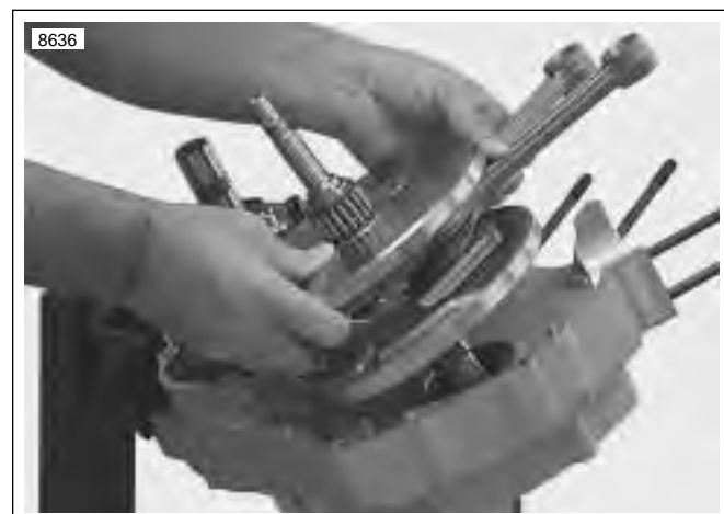
Figure 6-54. Removing Flywheels from Left Case Half
