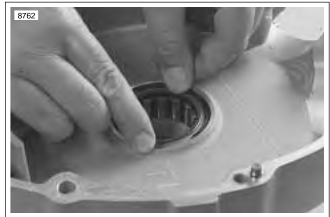
Figure 3-142. Removing Sprocket Shaft Bearing Retaining Ring
