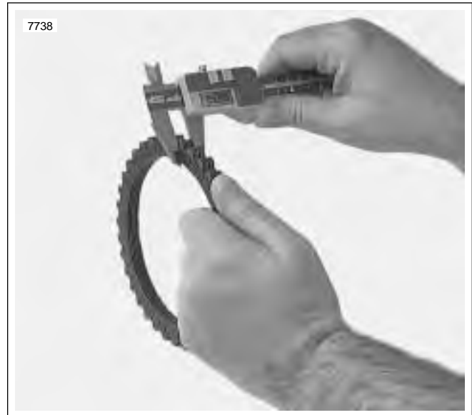
Figure 6-17. Measuring Friction Plates
