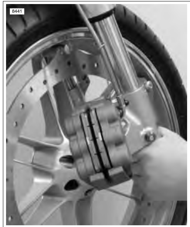
Figure 2-19. Front Wheel Installation
