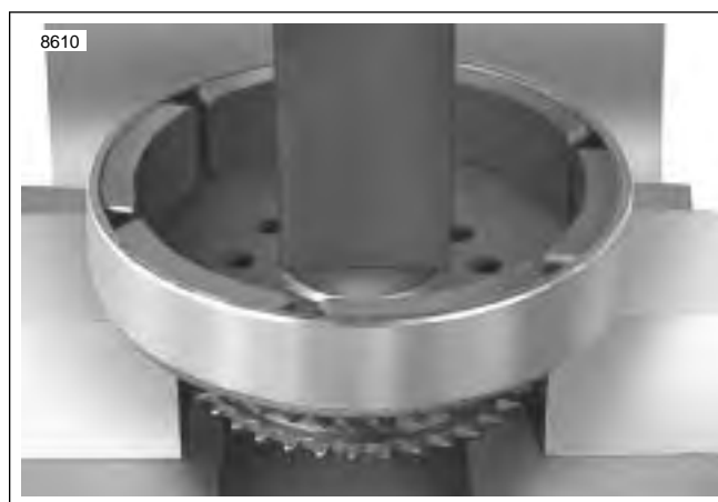
Figure 7-33. Removing Rotor From Sprocket
