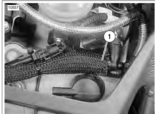
Figure 4-76. Engine Temperature Sensor Connector Approximate Location [90]
