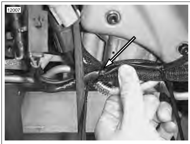
Figure 7-98. Cable Strap Wire Bundle to Return Oil Line
