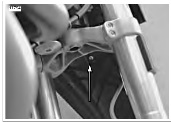
Figure 1-60. Vertical Headlight Adjustment Screw
