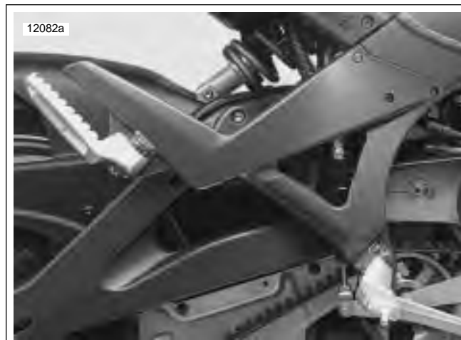
Figure 2-118. Right Side Heel Guard and Footpeg Mount
