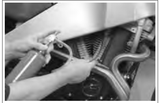
Figure 4-106. Checking for Intake Leak
