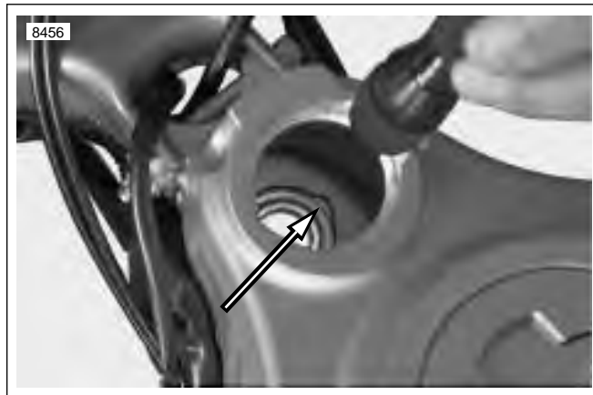
Figure 2-79. Lower Steering Head Bearing Notches (upper bearing removed for clarity)
