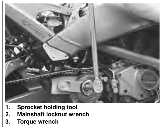
Figure 6-102. Transmission Sprocket Tightening
