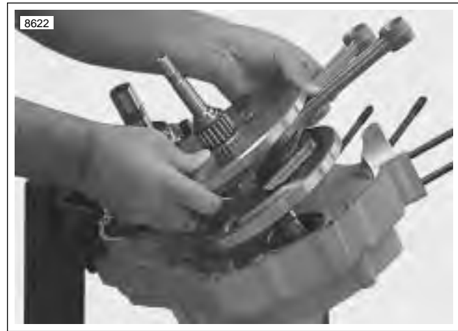
Figure 3-138. Removing Flywheels from Left Crankcase
