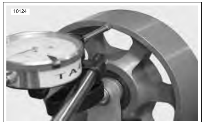
Figure 1-31. Checking Lateral Side Play on Idler Pulley with a Dial Indicator
