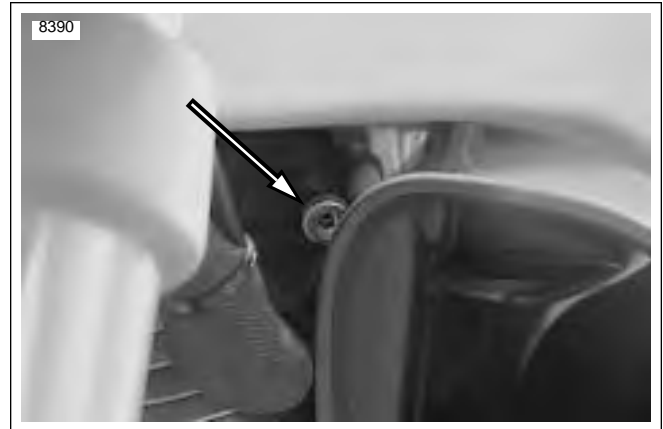
Figure 1-62. Idle Adjuster (behind left fork)
