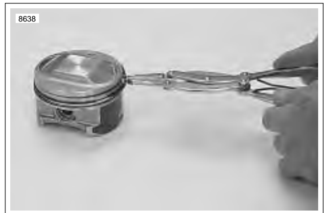
Figure 3-89. Removing Piston Rings
