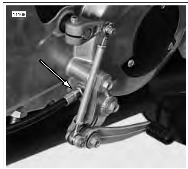
Figure 2-104. Clutch Cable and Fitting
