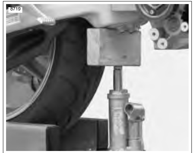
Figure 3-25. Supporting the Swingarm (Typical)
