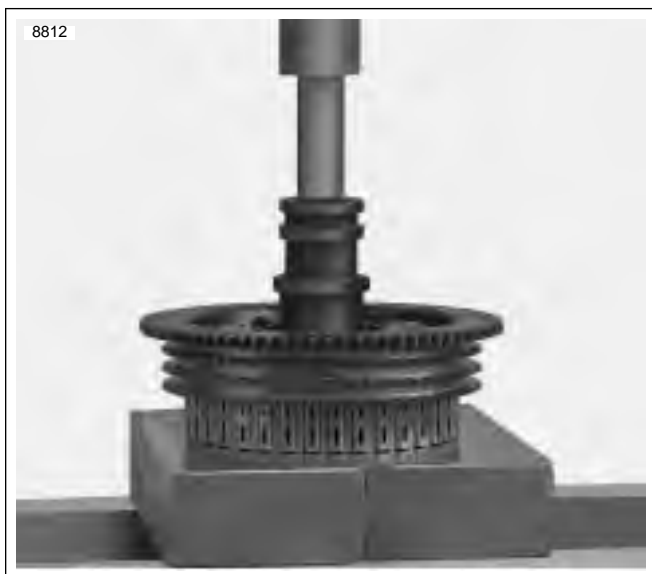
Figure 6-30. Removing Clutch Shell Needle Bearing
