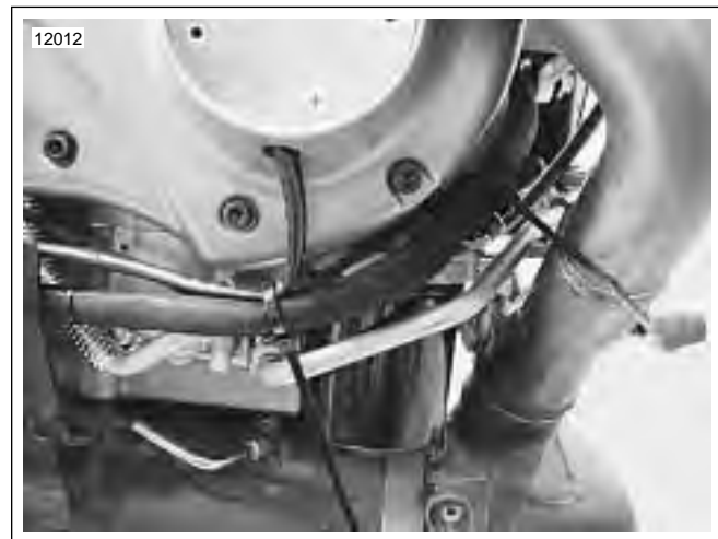
Figure 7-96. Cable Strap Locations
