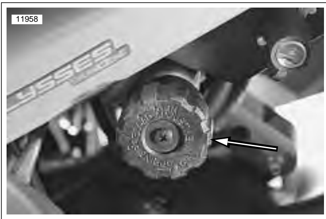
Figure 1-37. Rear Shock Preload Adjuster
