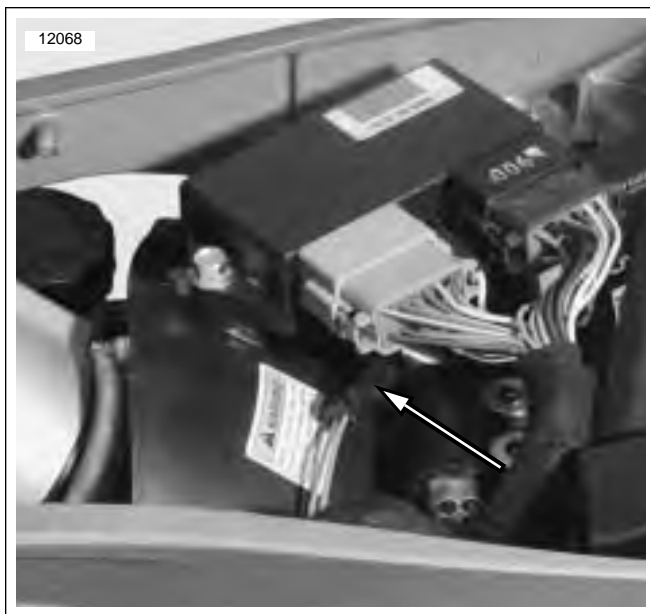
Figure 2-57. Brake Light Switch Connector
