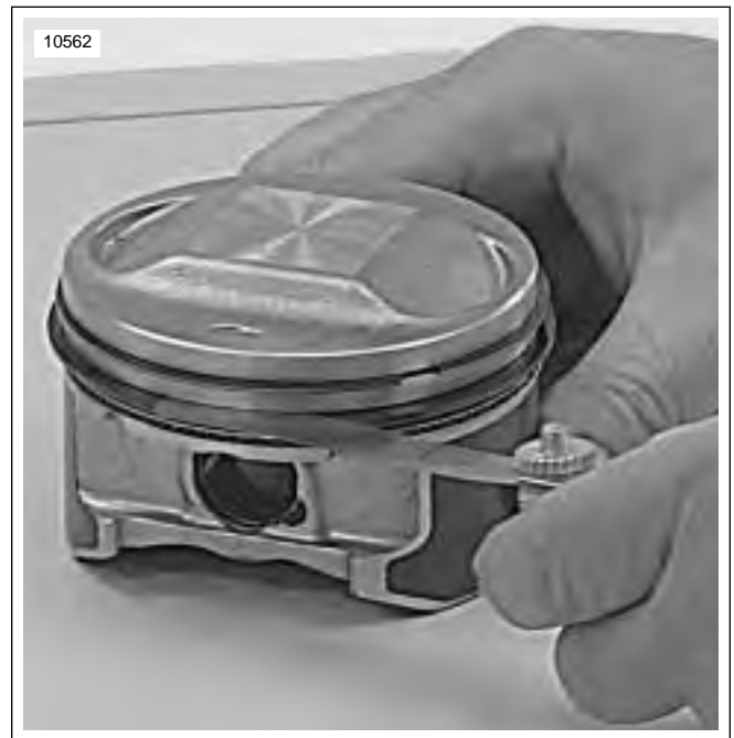
Figure 3-96. Measuring Ring Clearance in Groove
