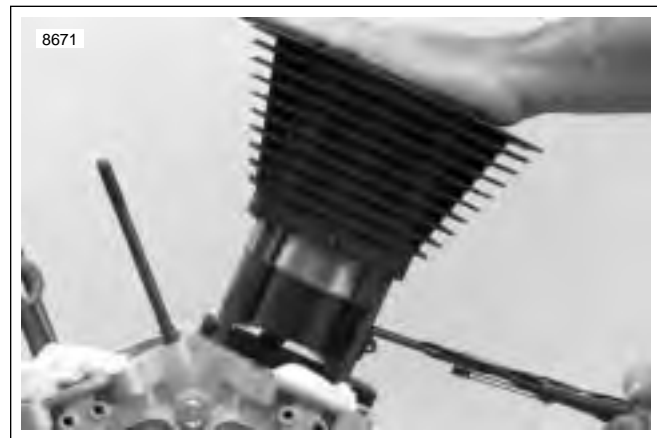
Figure 3-106. Compressing Piston Rings Using Piston Ring Compressor (Part No. HD-96333-51C)
