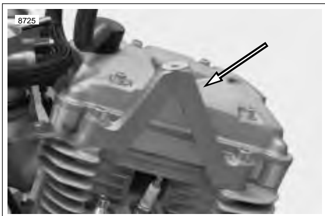
Figure 3-35. Center Tie Bar Mount
