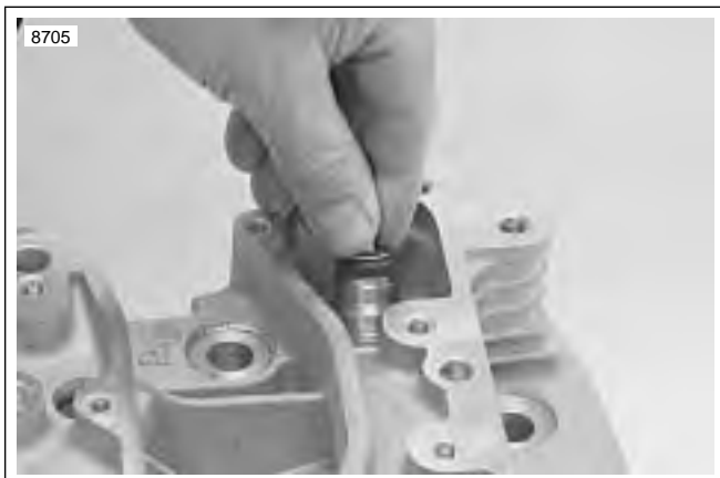
Figure 3-78. Valve Seal and Lower Collar Assembly Installation
