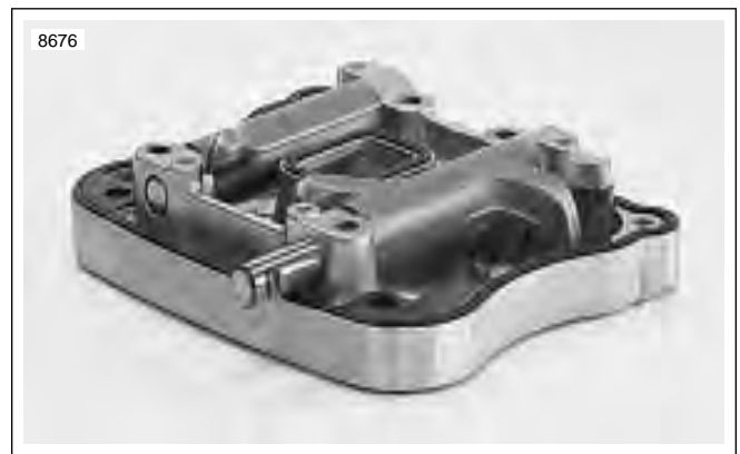
Figure 3-59. Removing Rocker Arm Shafts
