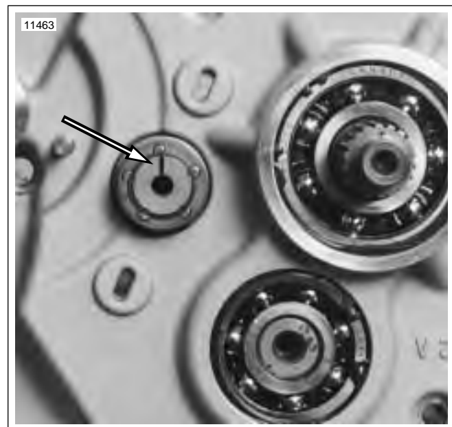
Figure 6-48. Shifter Drum and Mainshaft (Transmission in Neutral)
