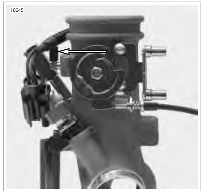
Figure 4-113. Emissions Hose Attachment, California Models Only
