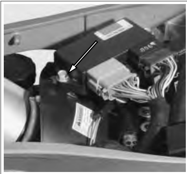
Figure 2-131. ECM Fastener with Captured Nut
