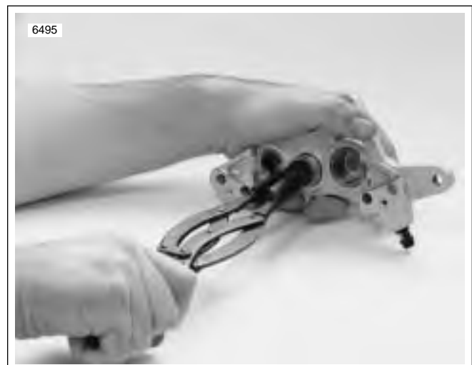
Figure 2-49. Removing Pistons (B-42887)
