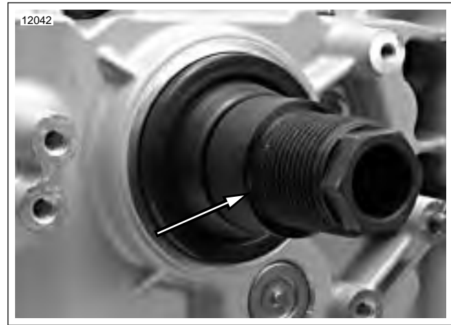
Figure 6-79. Install ADAPTER (Part No. HD-47856-4) (Typical)
