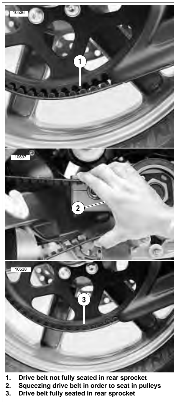
Figure 6-42. Seating Drive Belt Into Pulley Teeth
