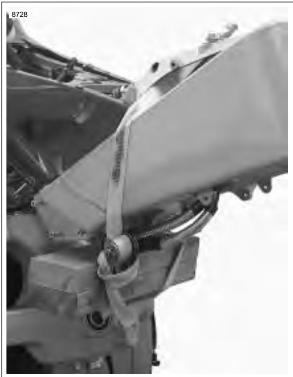
Figure 3-31. Securing Vehicle for Relocation (Typical)
