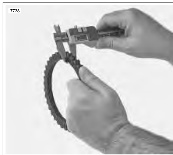
Figure 6-17. Measuring Friction Plates
