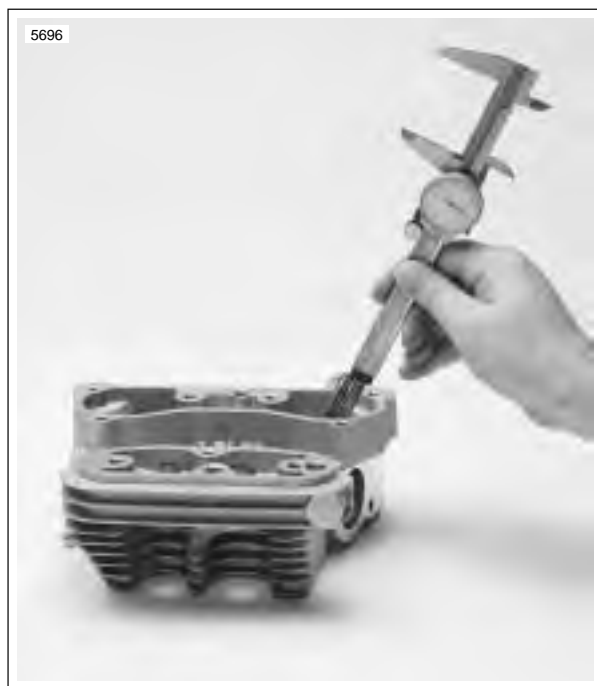
Figure 3-67. Measuring Valve Stem Protrusion
