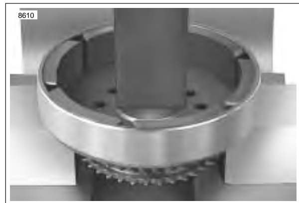
Figure 7-33. Removing Rotor From Sprocket
