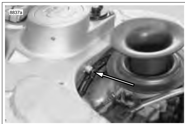
Figure 7-85. Wire Harness Clip
