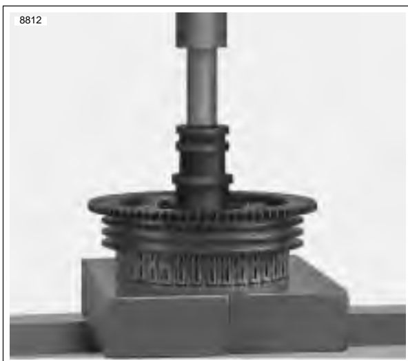
Figure 6-30. Removing Clutch Shell Needle Bearing
