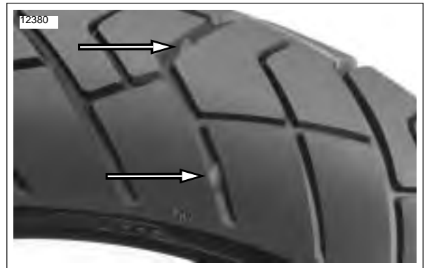
Figure 1-23. Tire Wear Indicator Bars (TWI) Pirelli Scorpion Sync
