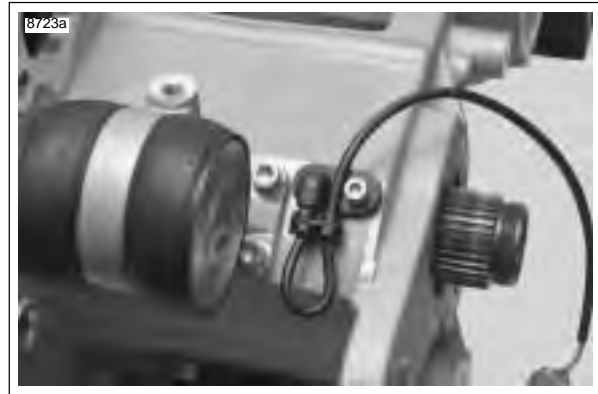
Figure 3-133. Rear Isolator Assembly
