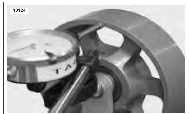
Figure 1-30. Checking Lateral Side Play on Idler Pulley with a Dial Indicator
