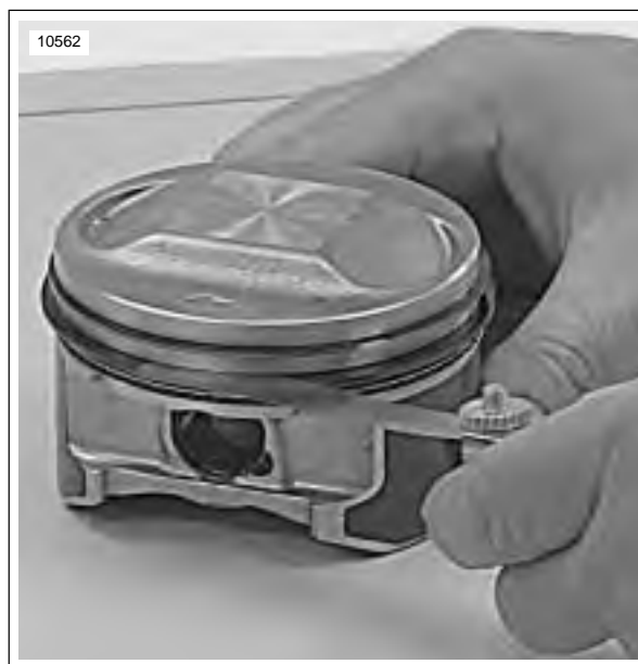
Figure 3-95. Measuring Ring Clearance in Groove
