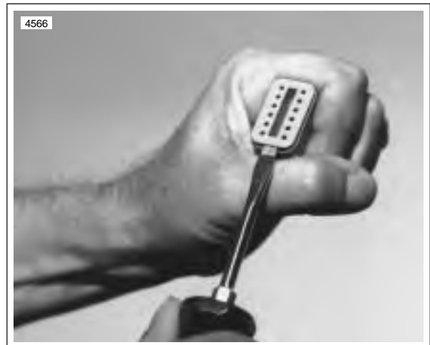
Figure B-6. Remove Secondary Locking Wedge
