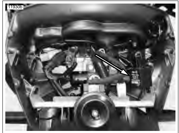
Figure 7-59. Turn Signal Flasher
