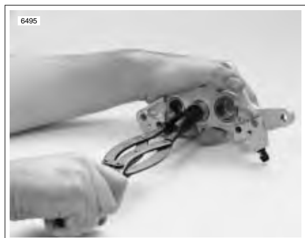
Figure 2-48. Removing Pistons (B-42887)
