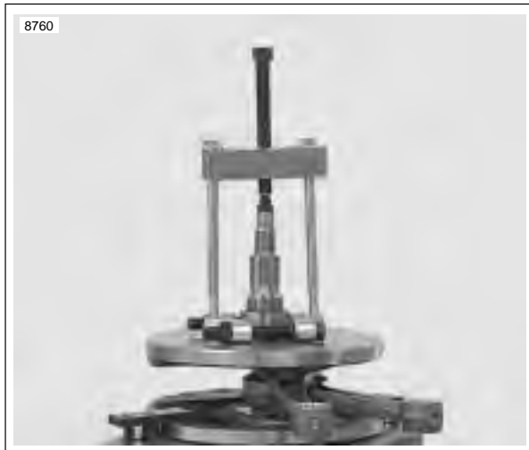
Figure 3-138. Removing Sprocket Shaft Inner Bearing Race
