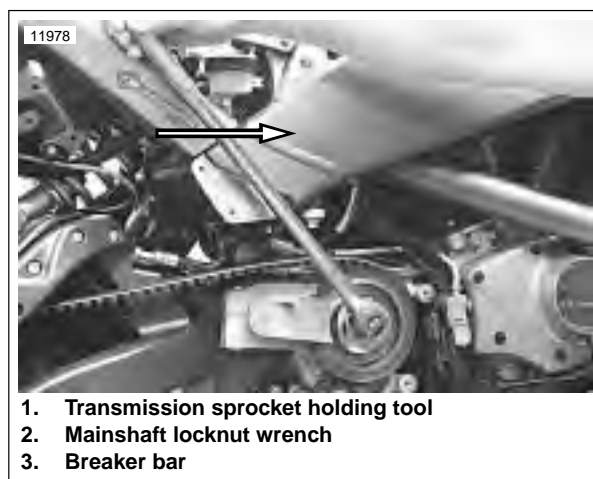
Figure 6-102. Removing Transmission Sprocket Locknut
