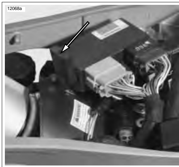
Figure 2-130. ECM Fastener with Captured Nut
