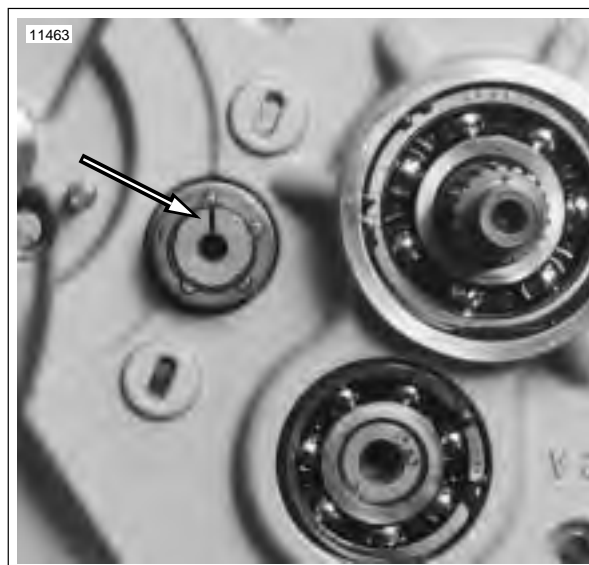
Figure 6-48. Shifter Drum and Mainshaft (Transmission in Neutral)
