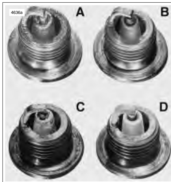
Figure 1-40. Typical Spark Plug Deposits
