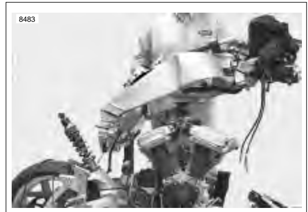
Figure 2-89. Lift Frame Off Motorcycle (Typical)
