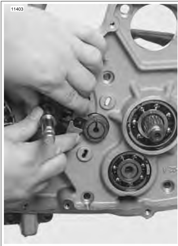
Figure 6-98. Installing Shifter Shaft Assembly
