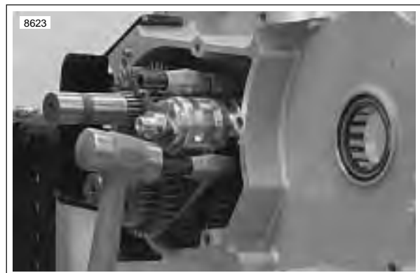
Figure 6-90. Installing Shift Fork Shafts
