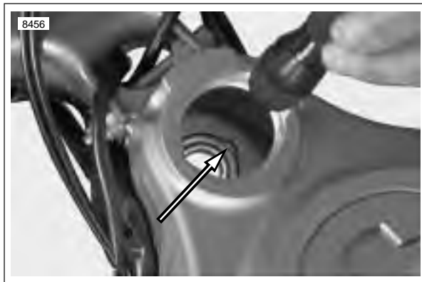
Figure 2-78. Lower Steering Head Bearing Notches (upper bearing removed for clarity)
