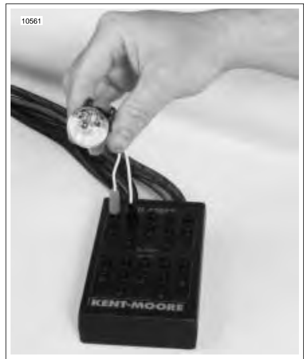
Figure 4-48. Testing Ignition Coil Connectors
