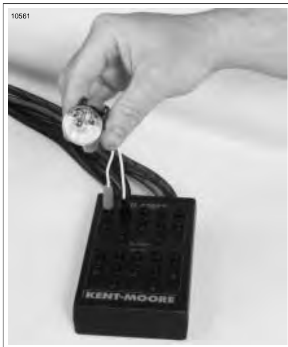
Figure 4-19. Ignition Coil Circuit Test
