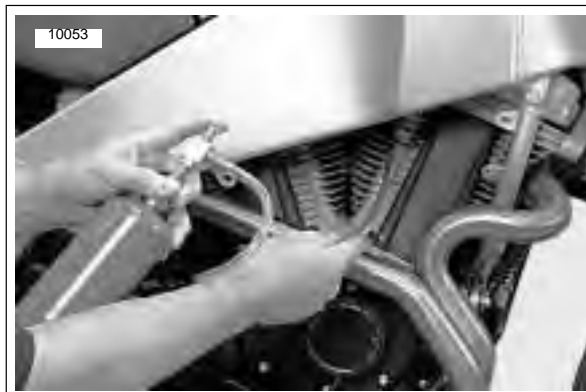
Figure 4-110. Checking for Intake Leak
